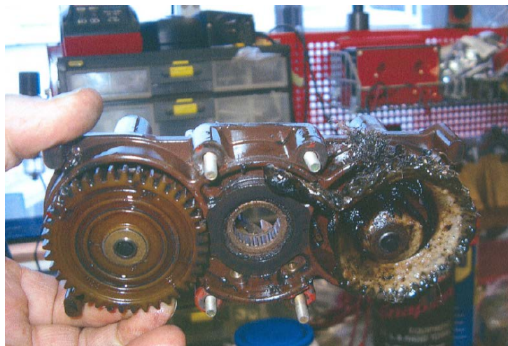
Figure 23 - Missing bearing retainer plate screws
