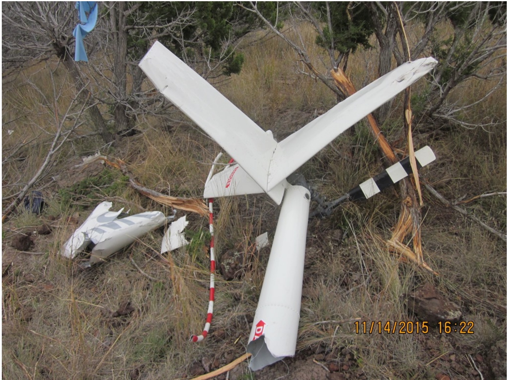
Photo 4 – Tailboom/Tail Rotor (FAA Photo)
