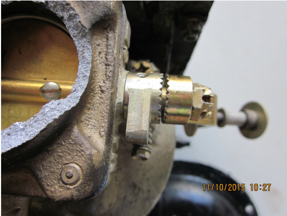
Photo 1: Disconnected throttle arm
