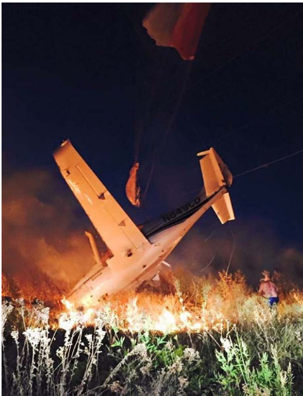
Photo 1 – accident airplane suspended from power lines
