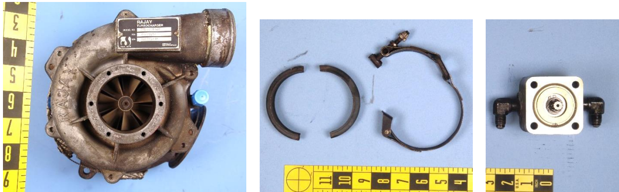
Figure 1. As-received Rajay turbocharger assembly (left side of page), fractured band clamp assembly (center of page), and scavenger pump assembly (right side of page).
