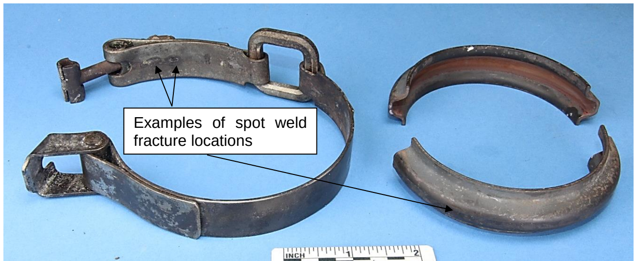
Figure 2. Close-up view of the as-received band clamp assembly showing the strap portion (left side of page) and two U-shaped retainers (right side of page). The cross section of a U-shaped retainer appears similar to a “U” groove. The fractured spot welds coincided with the bottom of the “U” groove portion. Arrows indicate examples of spot weld fracture locations.
