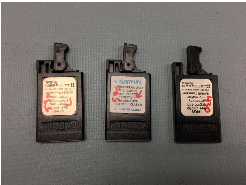
Figure 4. Garmin GNS 530 and 430 memory cards
