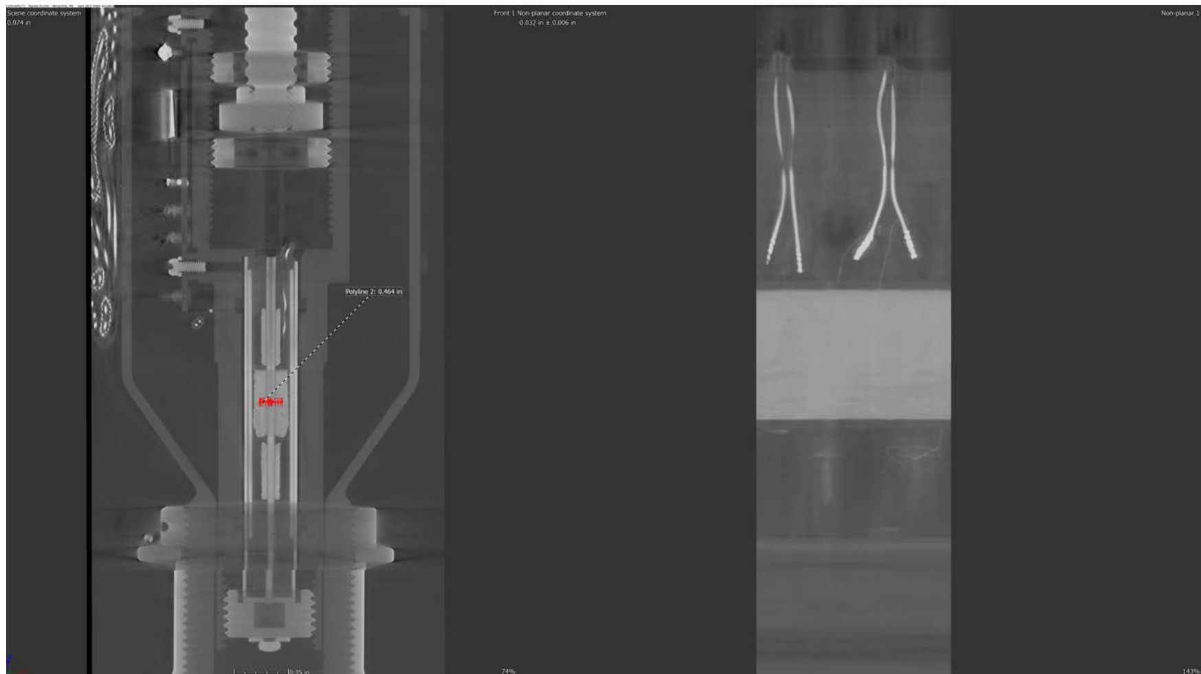
Figure 77 Right pitch linear actuator – LVDT connections – virtually unrolled
