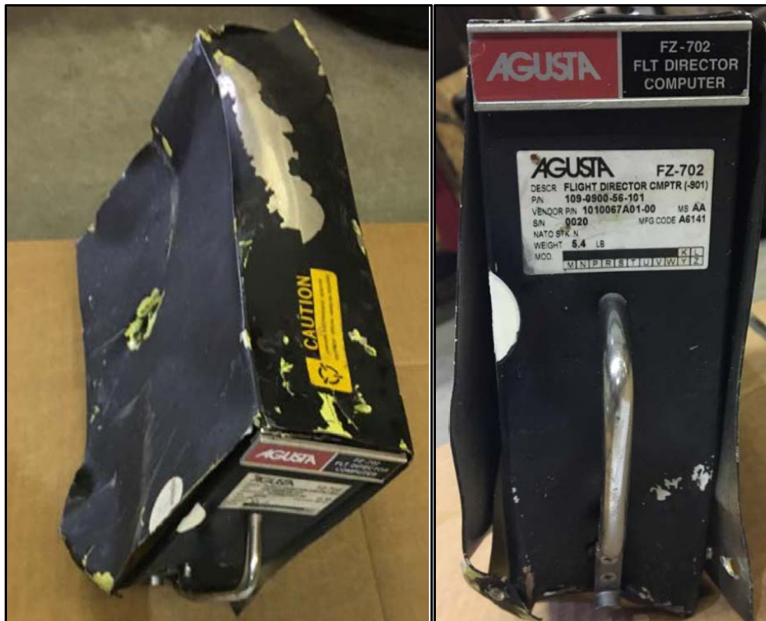
Figure 19 Flight director computer as photographed at the wreckage examination
