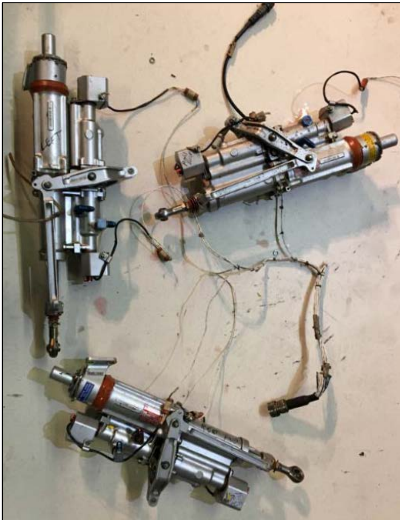
Figure 21 Main rotor actuators - at the wreckage examination
