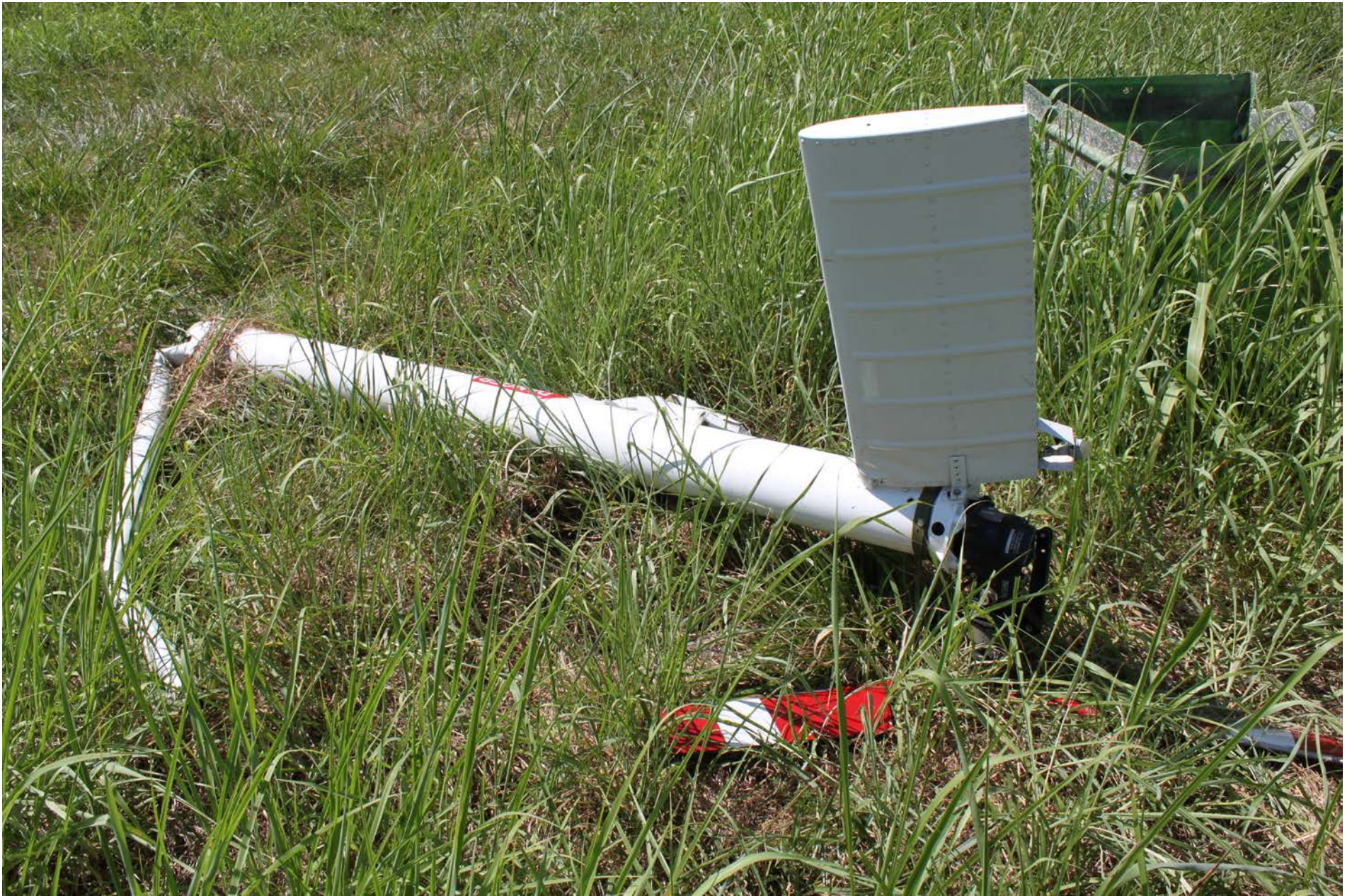
Photo 5 – View of Separated Tail Boom
