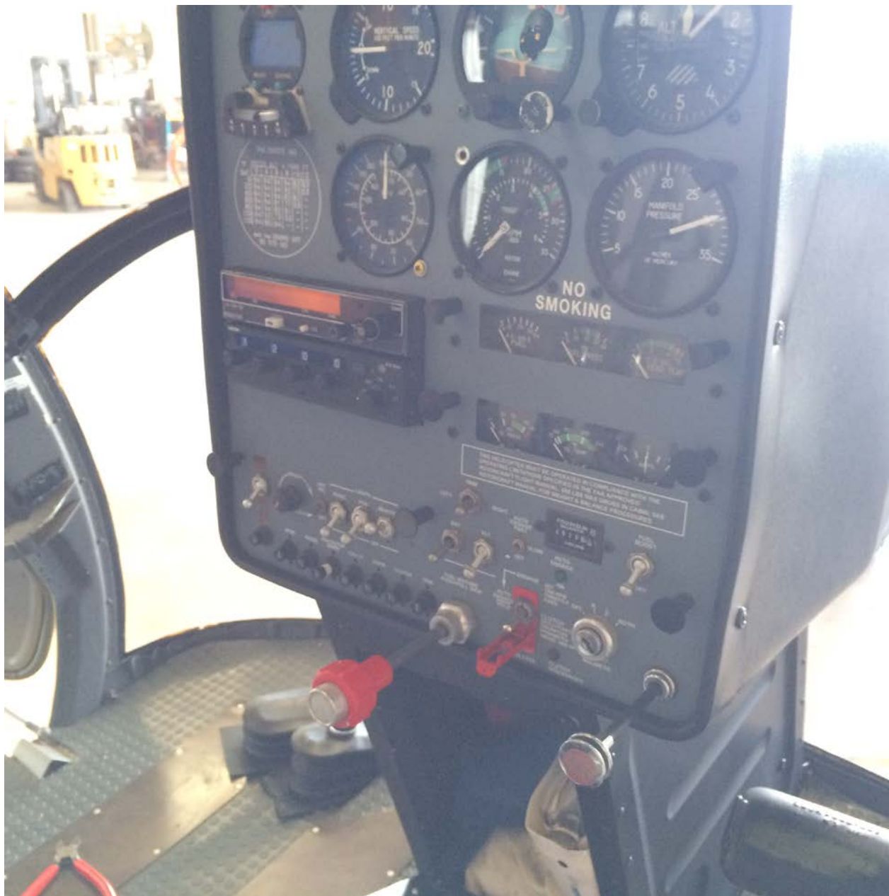
Photo 10 - Exemplar helicopter instrument panel.
