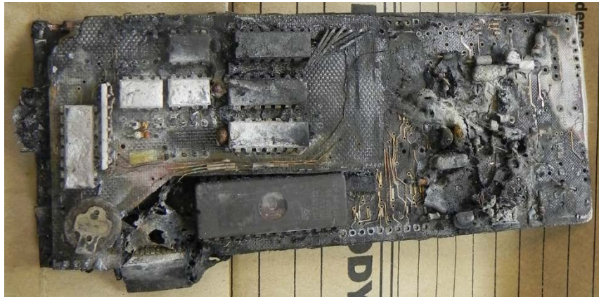
Figure 1. Image of the main printed circuit board showing effects of catastrophic fire damage.
