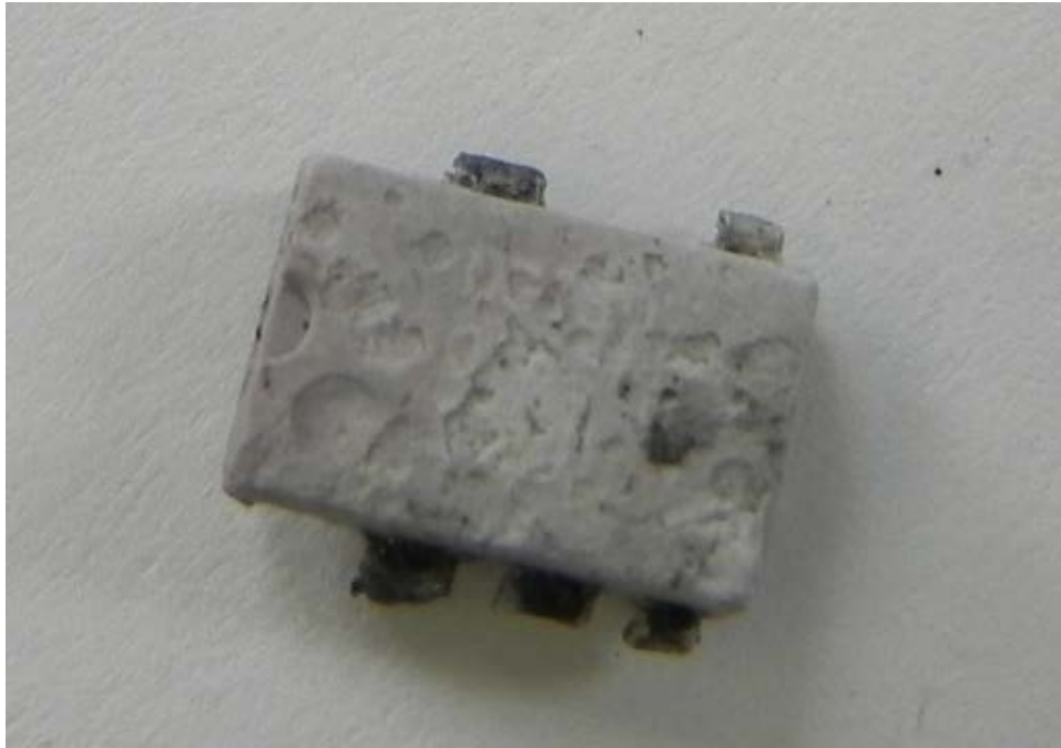
Figure 3. Image of FLASH memory integrated circuit showing fire damage to leads and packaging
