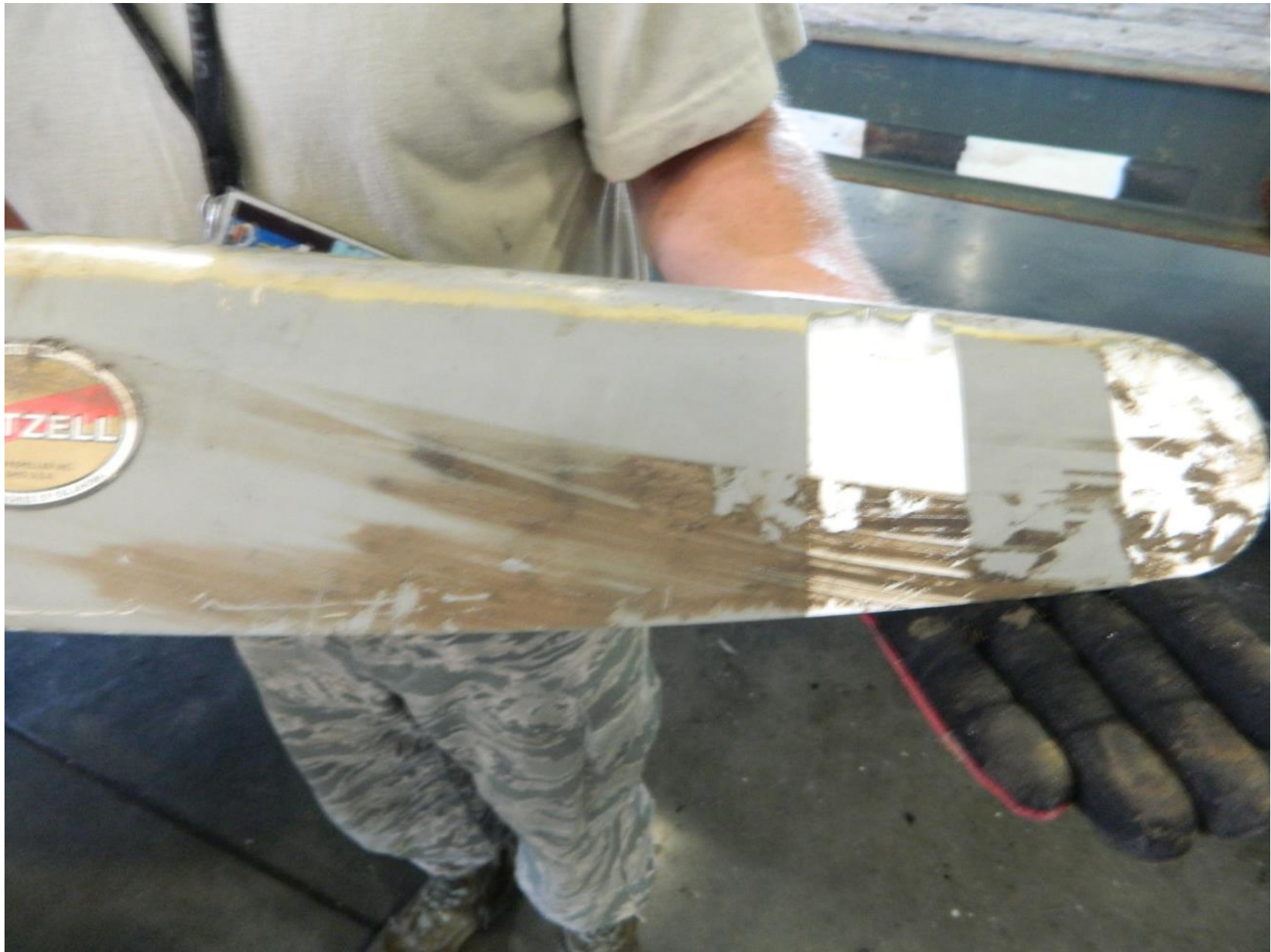
Photo 6 – Right Propeller Broken Blade
