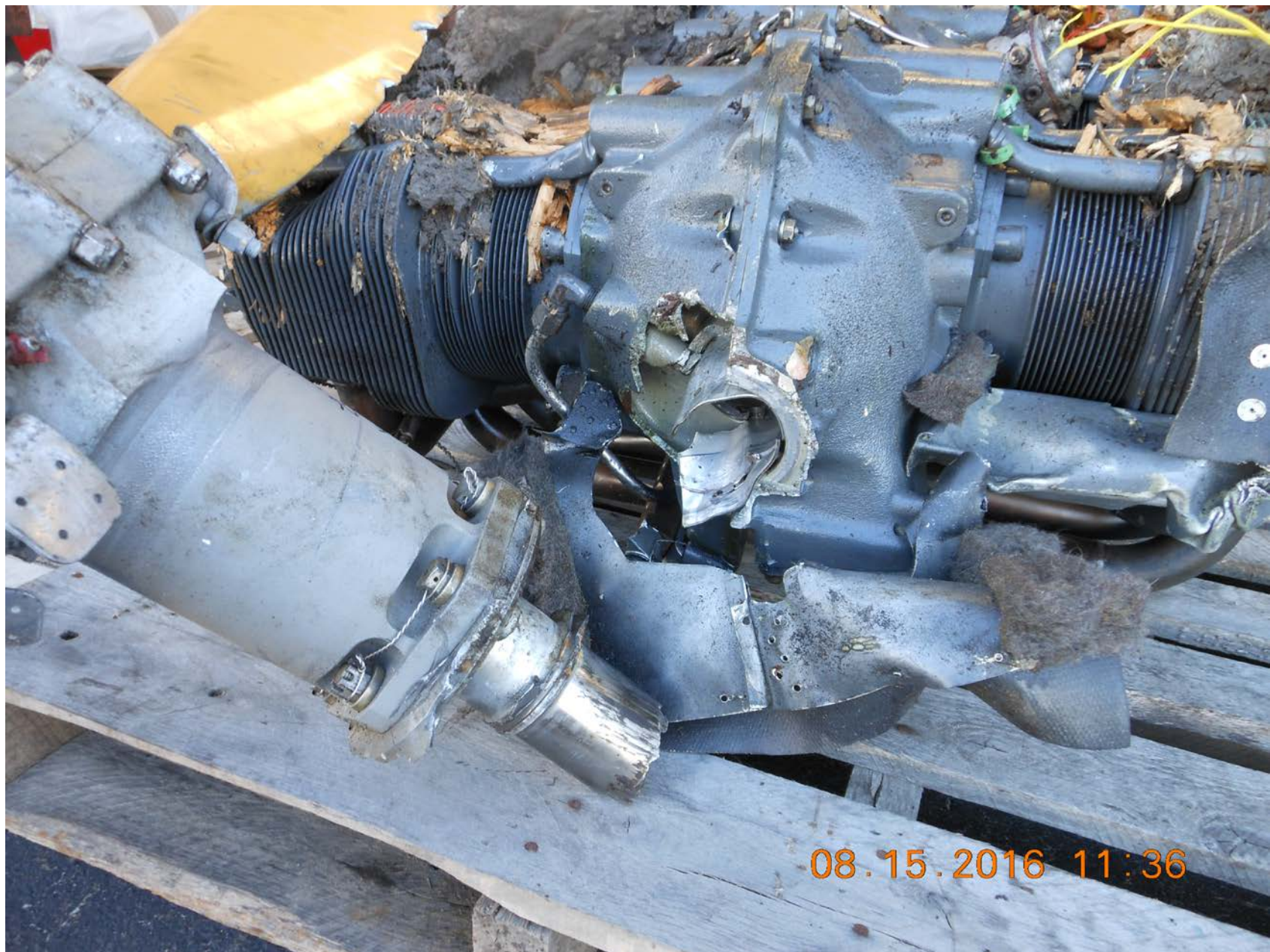
Photo 1 – View of the left propeller, separated crankshaft, and left engine. (Image supplied by Hartzell)
