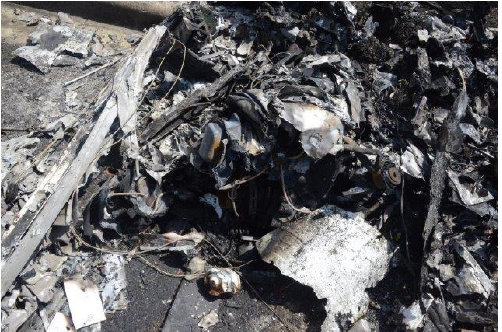
Photo 13 - View of the right engine within the main wreckage site.
