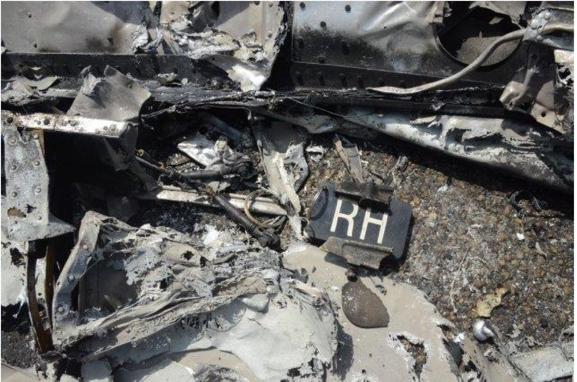
Photo 17 - View of right wing control cables within the main wreckage.
