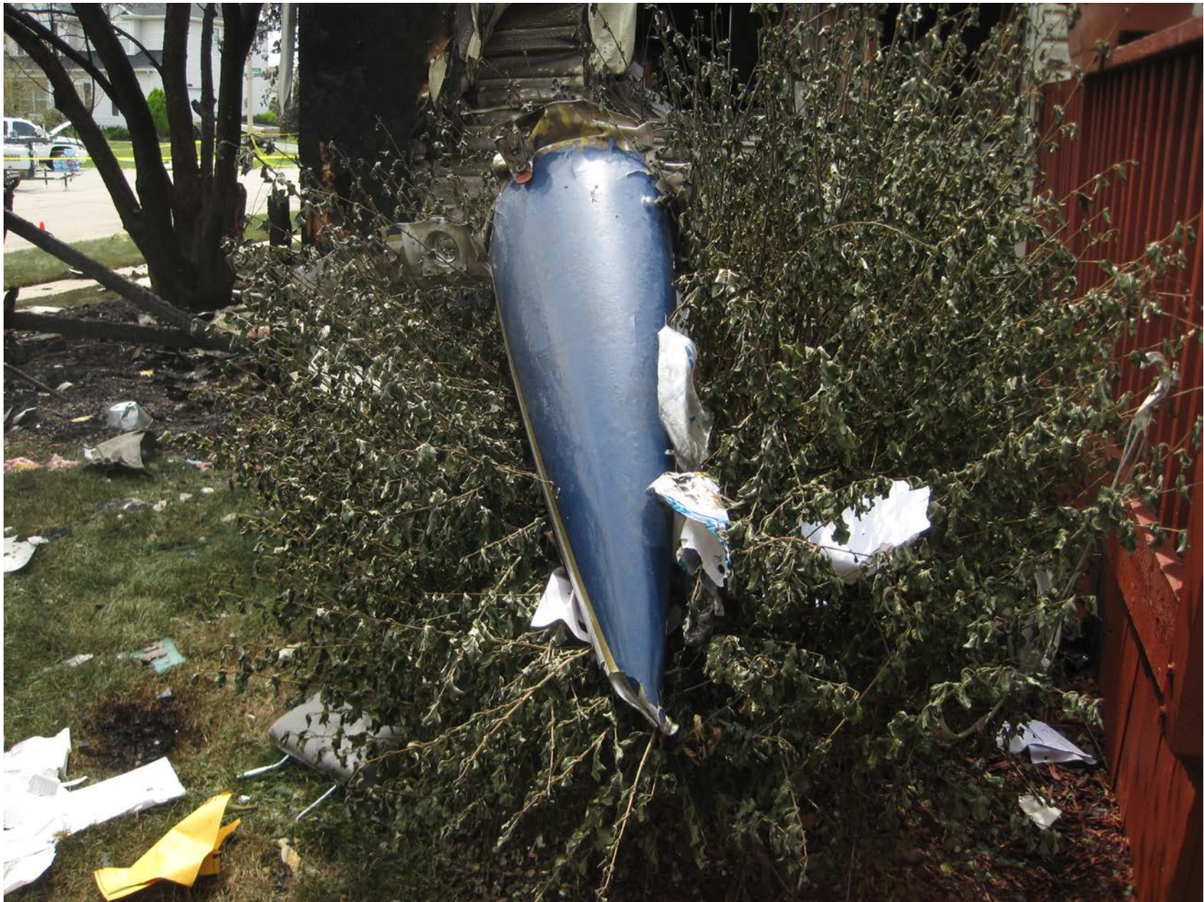
Photo 19 - View of the right tip tank near the main wreckage.
