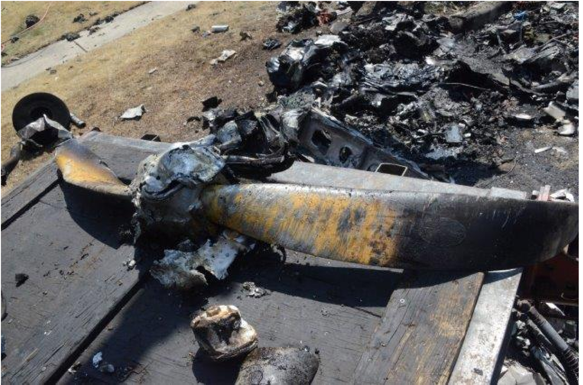
Photo 14 - View of the recovered right propeller.
