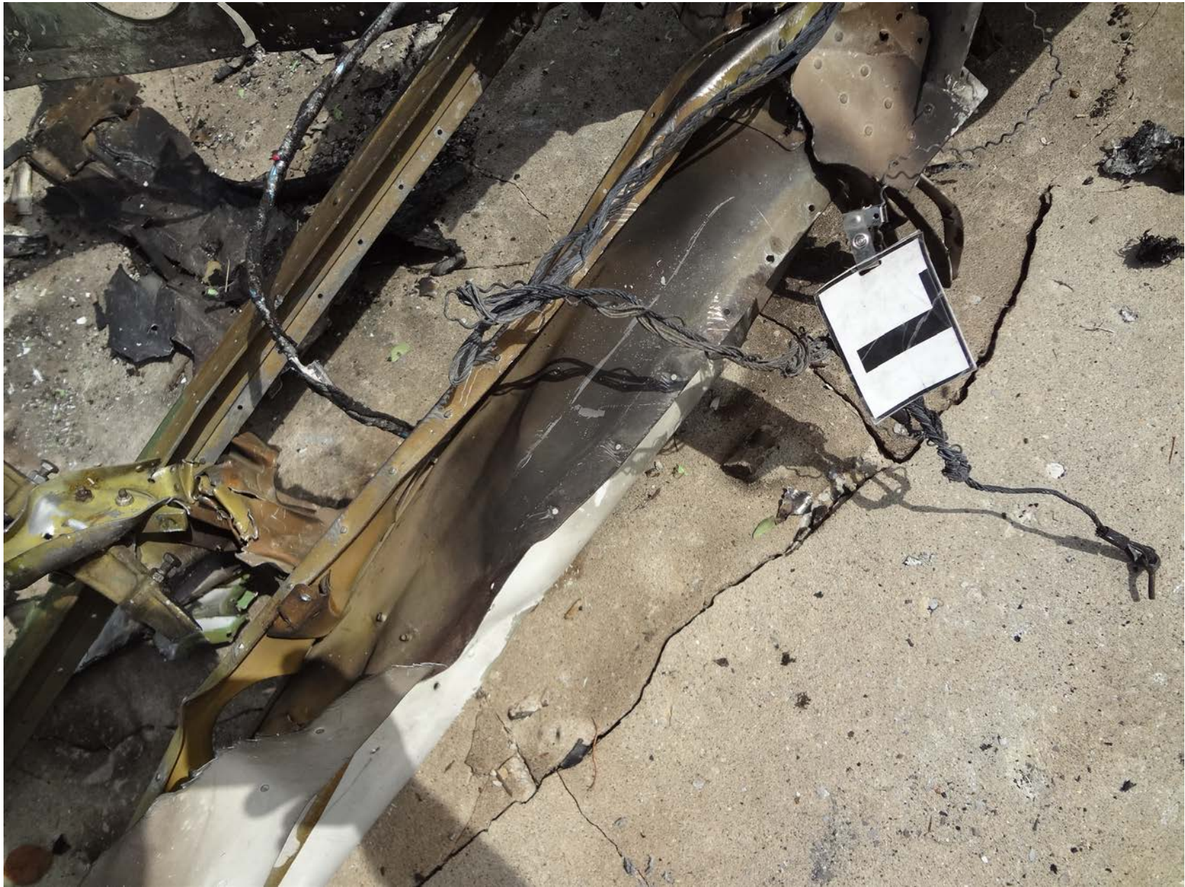
Photo 18 - View of left wing control cables within the main wreckage.
