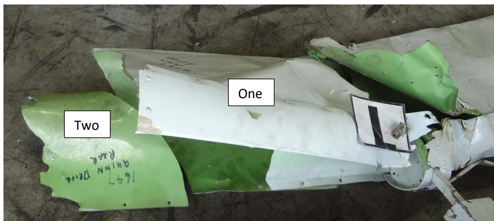
Figure 13 - Two additional aileron skin pieces recovered away from main wreckage and outboard left-wing section.
