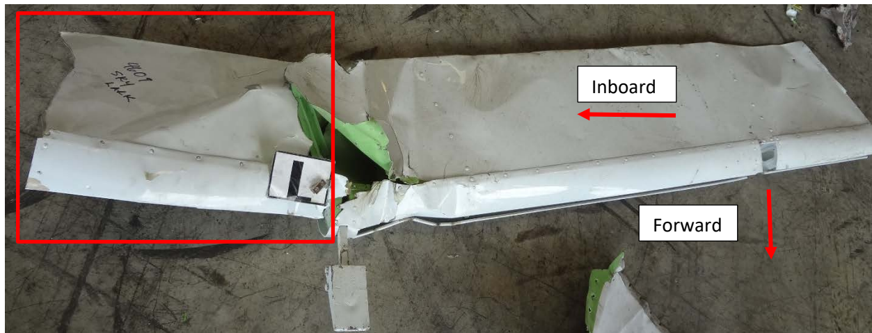
Figure 12 – Left aileron with additional skin panel recovered away from the main wreckage and left outboard wing.
