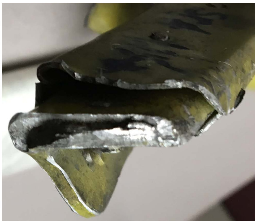
Figure 3 – Inboard side of left wing upper spar chord fracture at station 135 exhibiting evidence of up bending.
