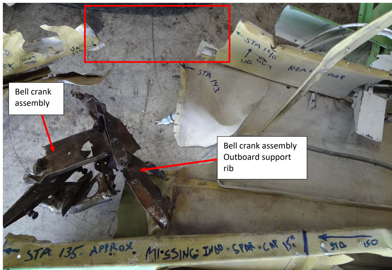
Figure 9 – Missing left-wing rear spar in the area of the inboard aileron hinge fitting.
