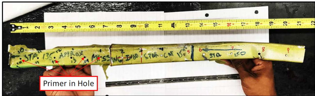
Figure 20 – Fastener holes with primer.
