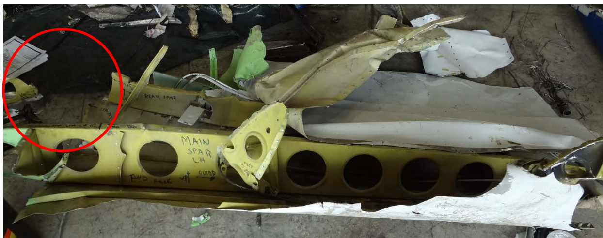
Figure 8 – Missing left-wing rear spar and aileron hinge fitting.
