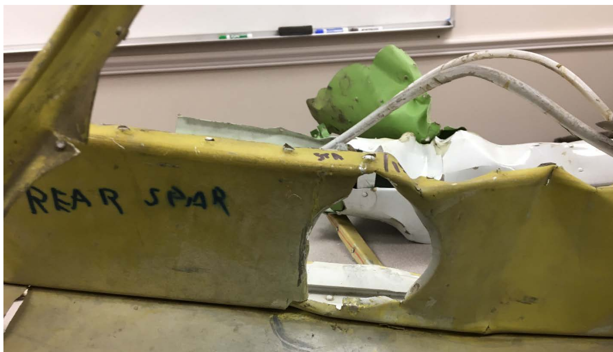
Figure 14 – left wing balance weight cut out damage in rear spar.
