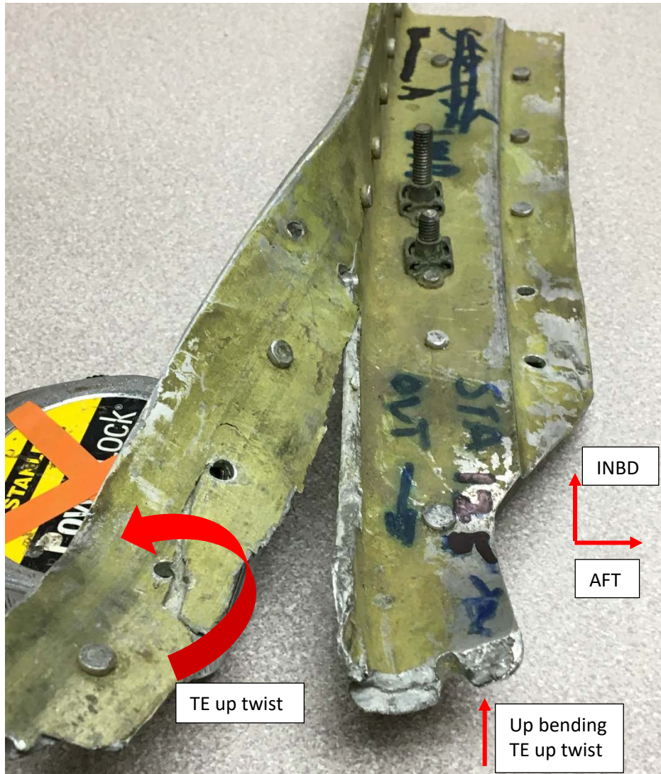
Figure 6 – Left wing lower main spar chord fracture at station 125.
