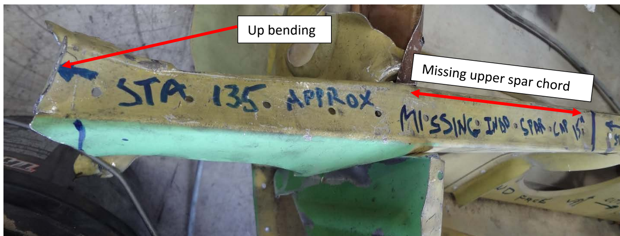
Figure 4 – Outboard section of left wing main spar fracture at station 135.
