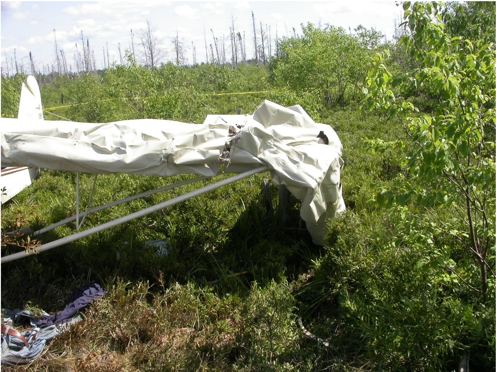
Photo 4 – View of damage to the left wing
