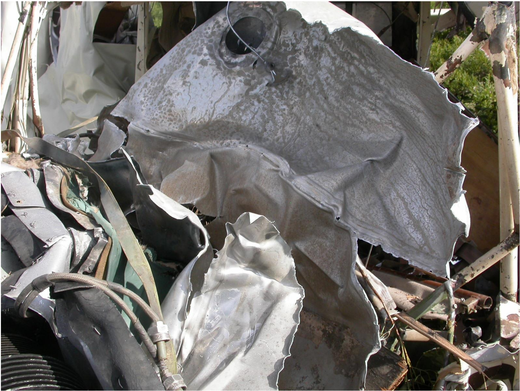
Photo 12 – View of inside of the main fuel tank
