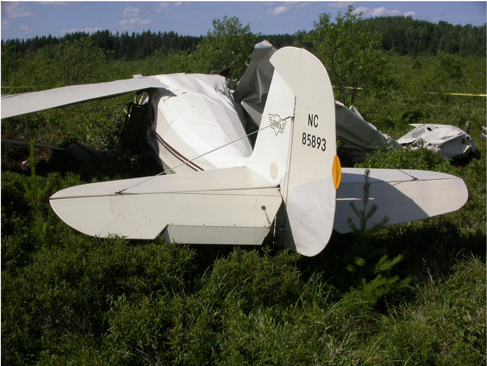
Photo 7 – View of the empennage
