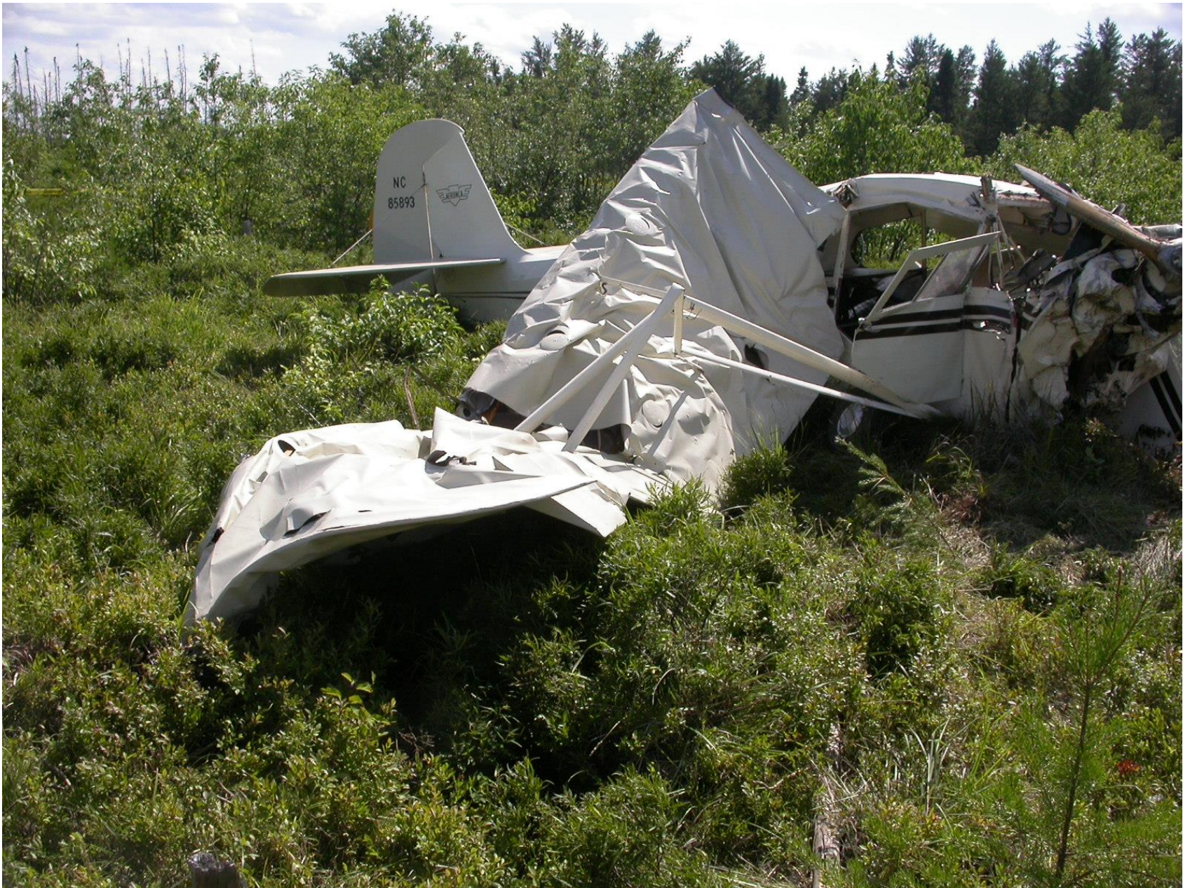
Photo 6 – View of damage to the right wing
