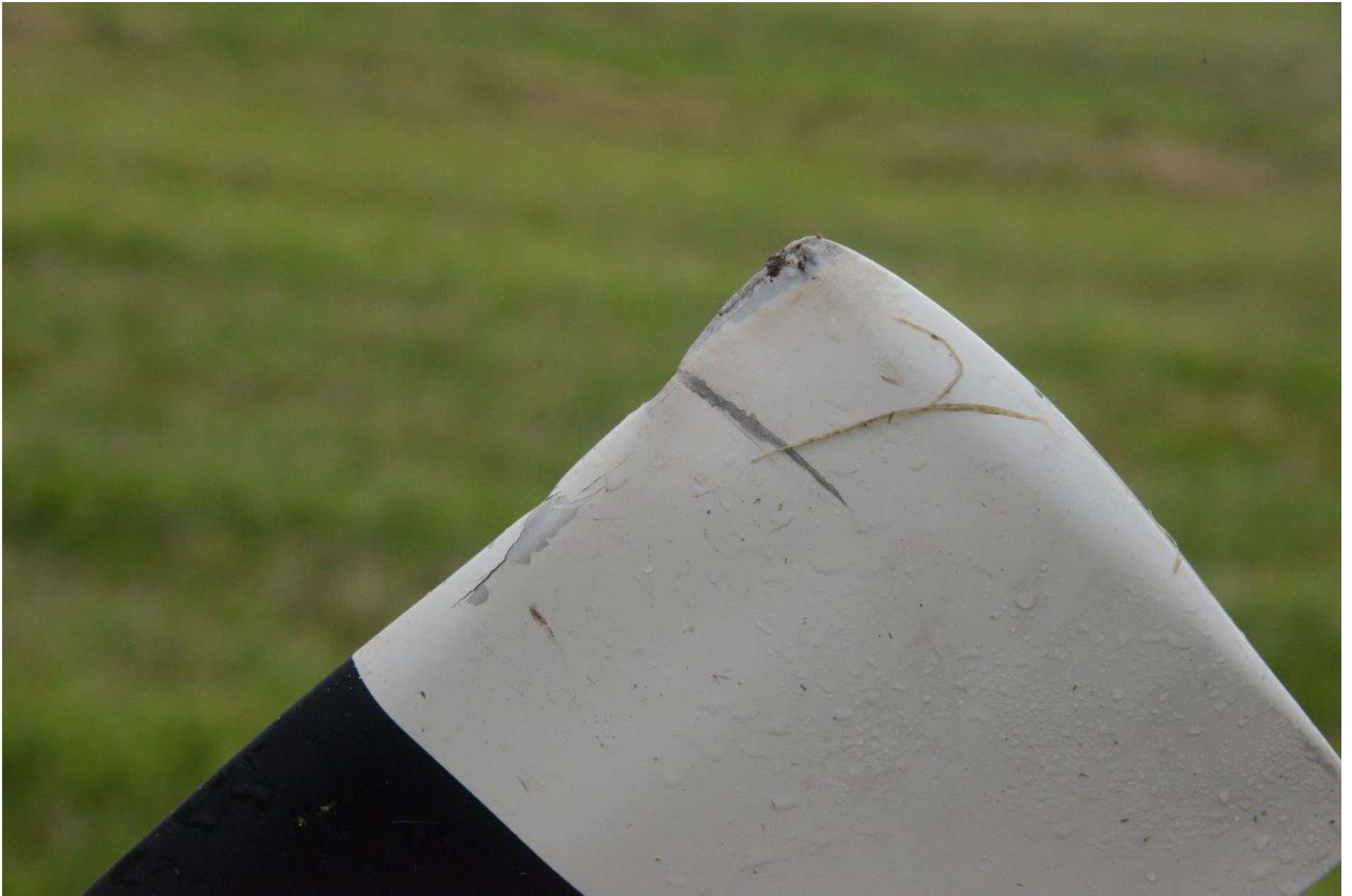
Photo 4 - View of witness marks on a separated tail rotor blade.
