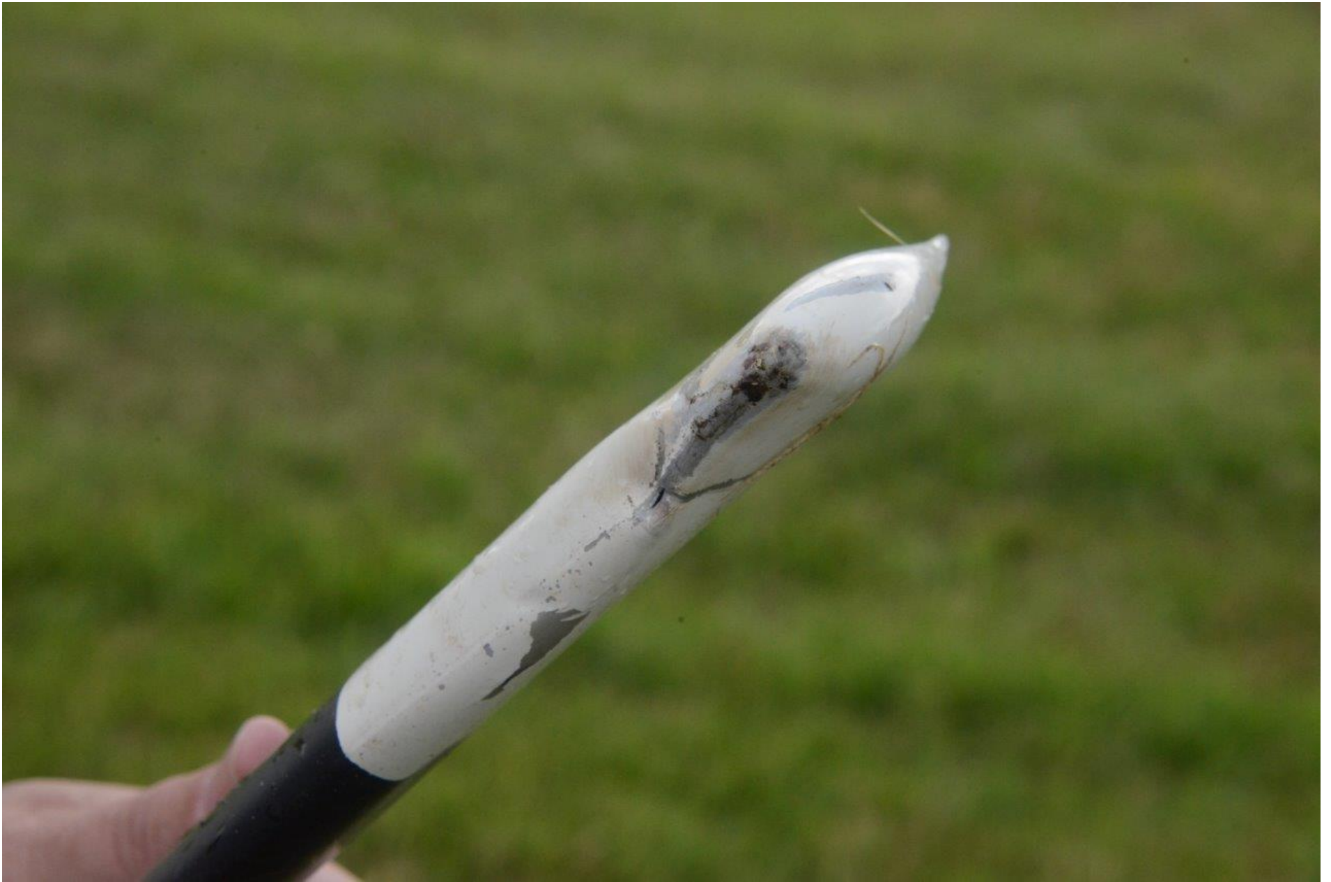
Photo 5 - View of witness marks on a separated tail rotor blade.
