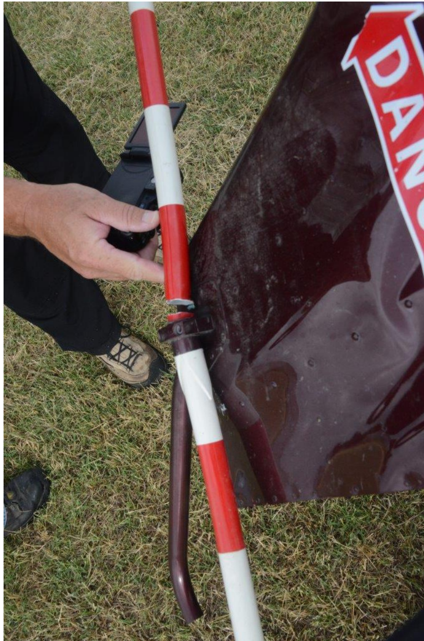
12BPhoto 13 - View of the tail rotor guard separation.
