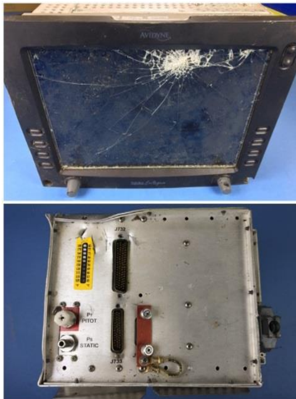
Figure 1. Damaged exterior Avidyne PFD from N508AJ.
