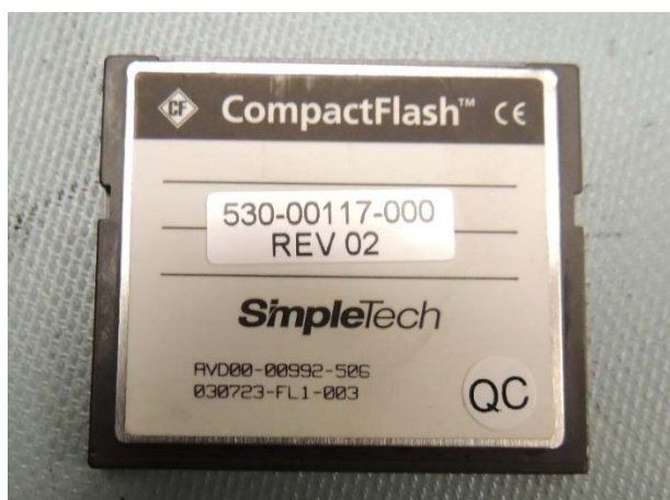
Figure 3. Internal CF Card from Avidyne MFD.
