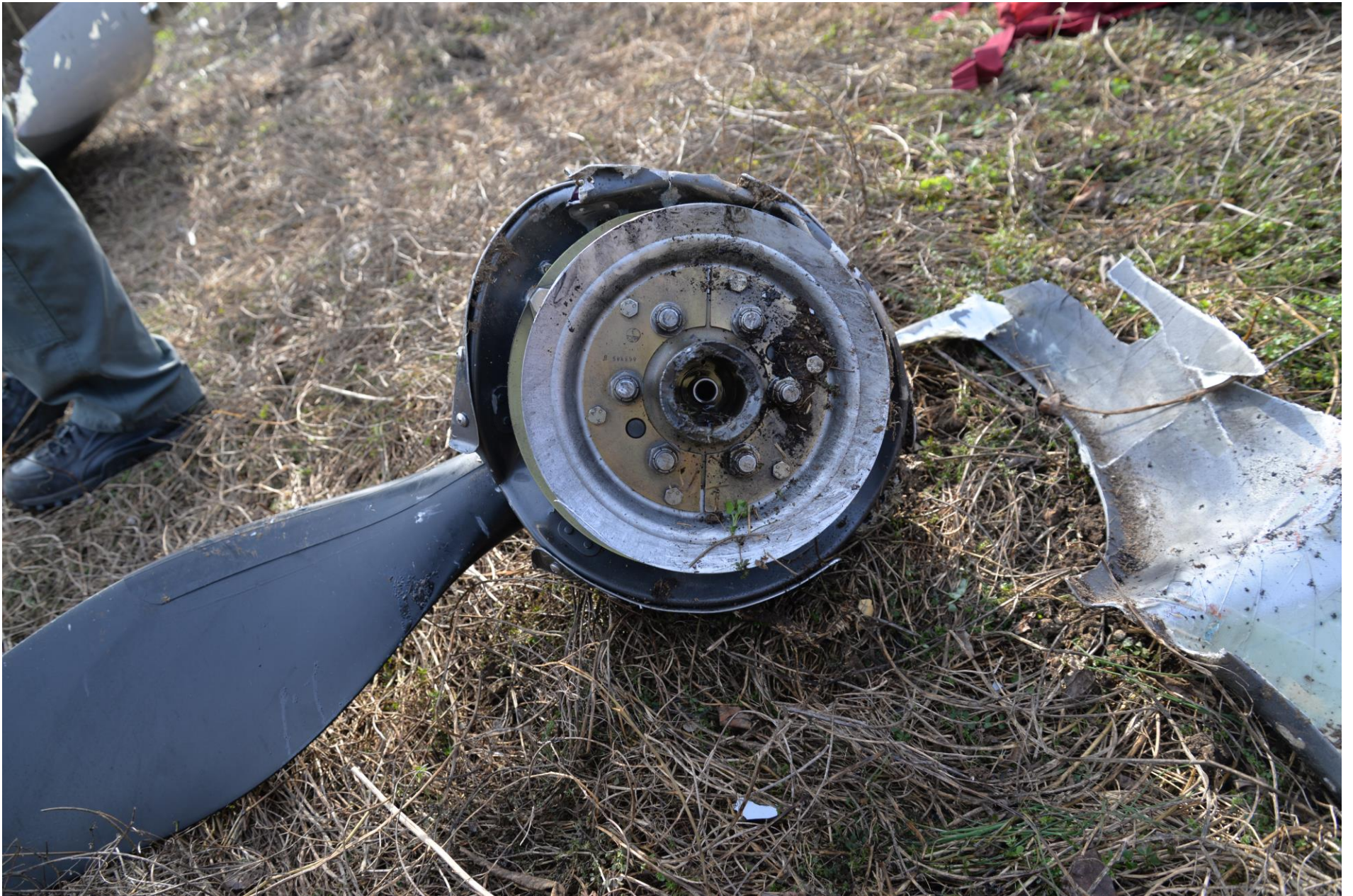
Photo 10 – Propeller Flange and Crankshaft Fracture
