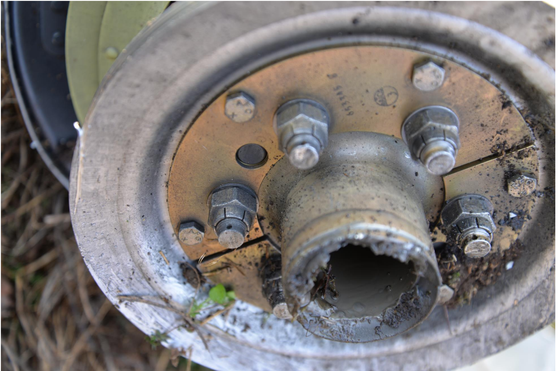
Photo 11 – Crankshaft Fracture, Detail
