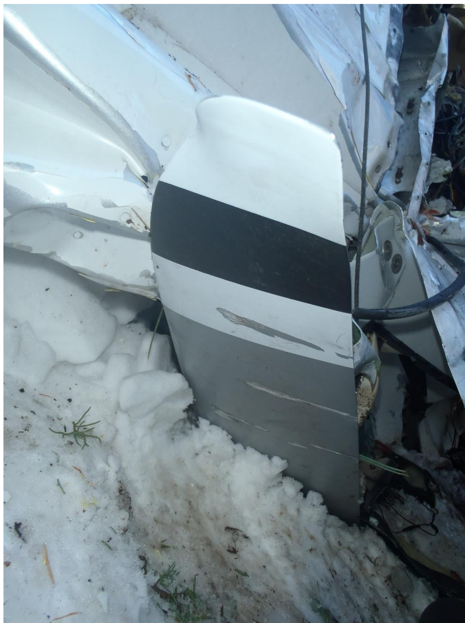
Photo 12 - Propeller blade B. Note spanwise striations on cambered surface.
