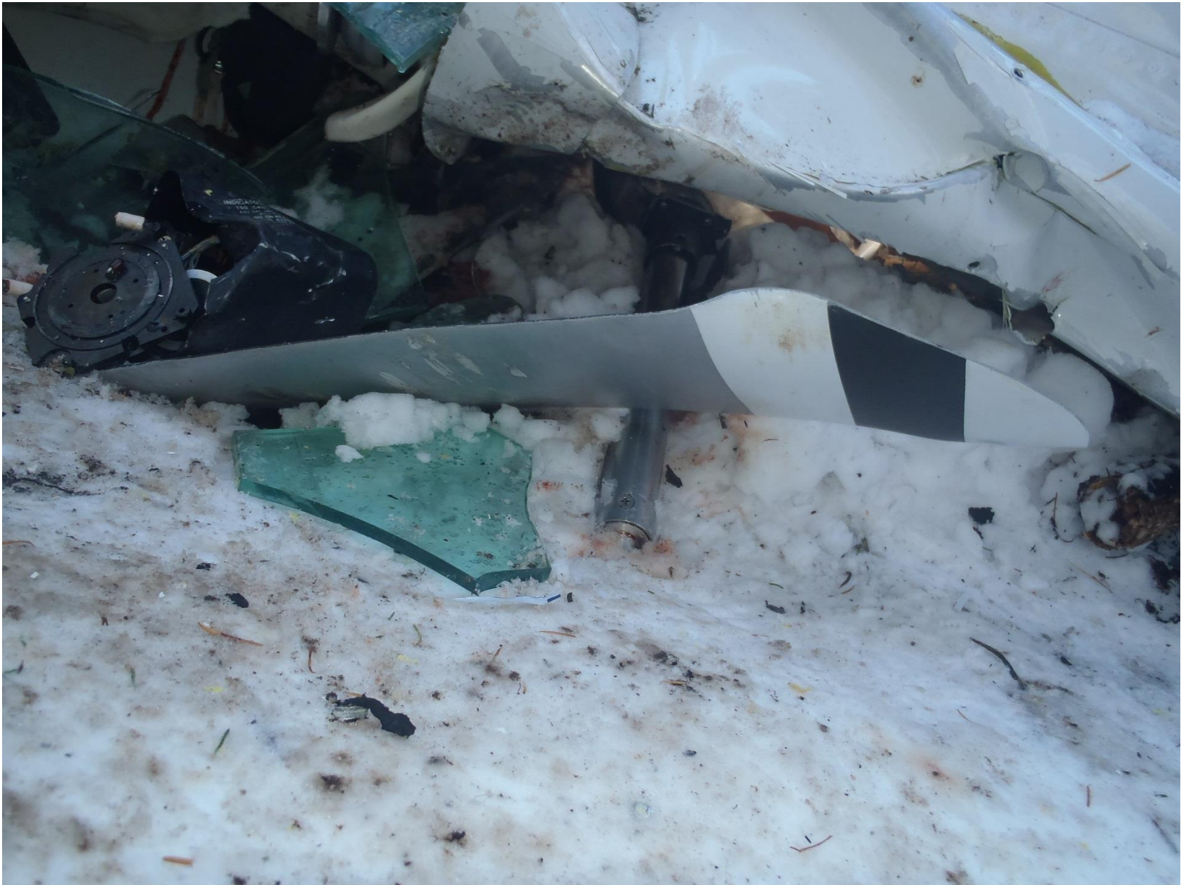
Photo 11 - Propeller blade A. Note forward bending near the blade tip.
