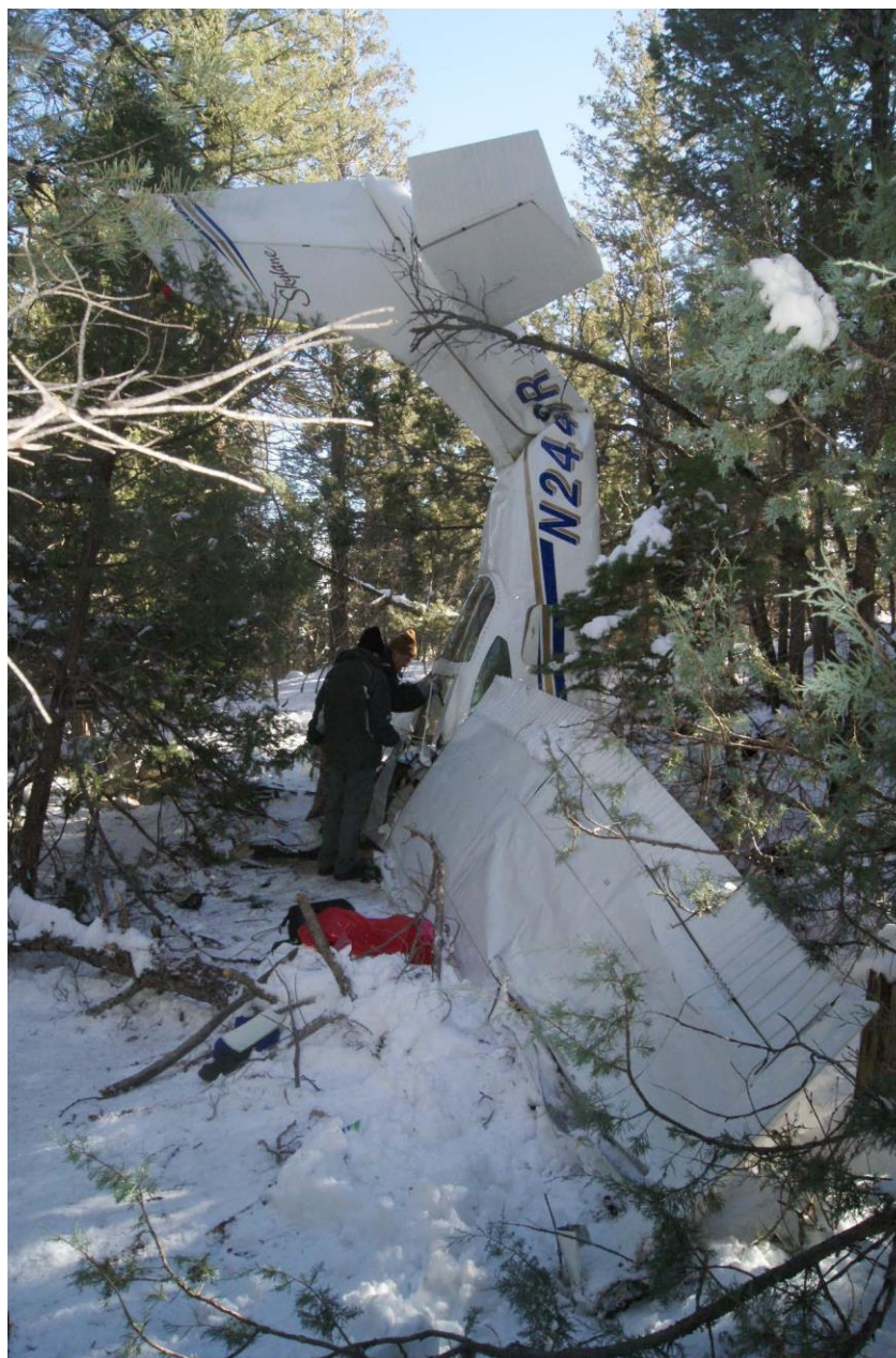
Photo 8 - Left side of airplane. Note near-horizontal impact with mountainous terrain.
