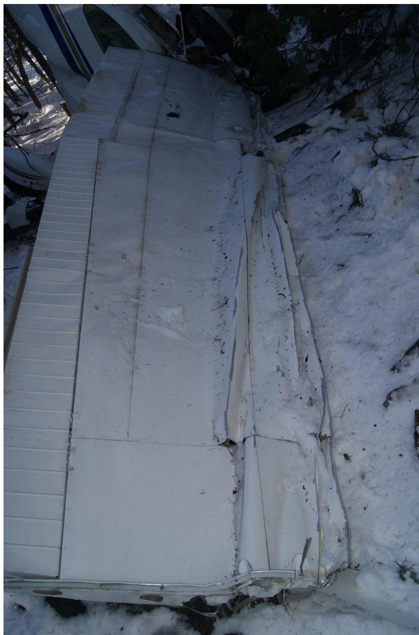
Photo 10 - Right wing and leading edge accordion-type crush damage.
