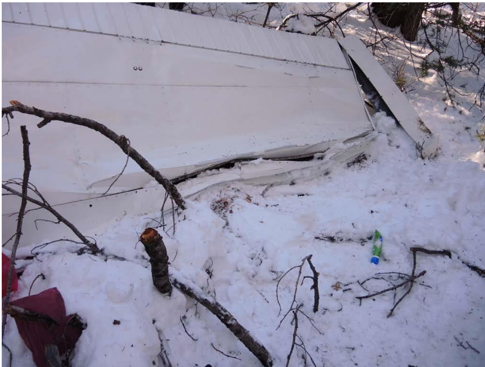
Photo 5 - Left wing leading edge. Note indentation consistent with a tree strike and scattered branches next to left wing.
