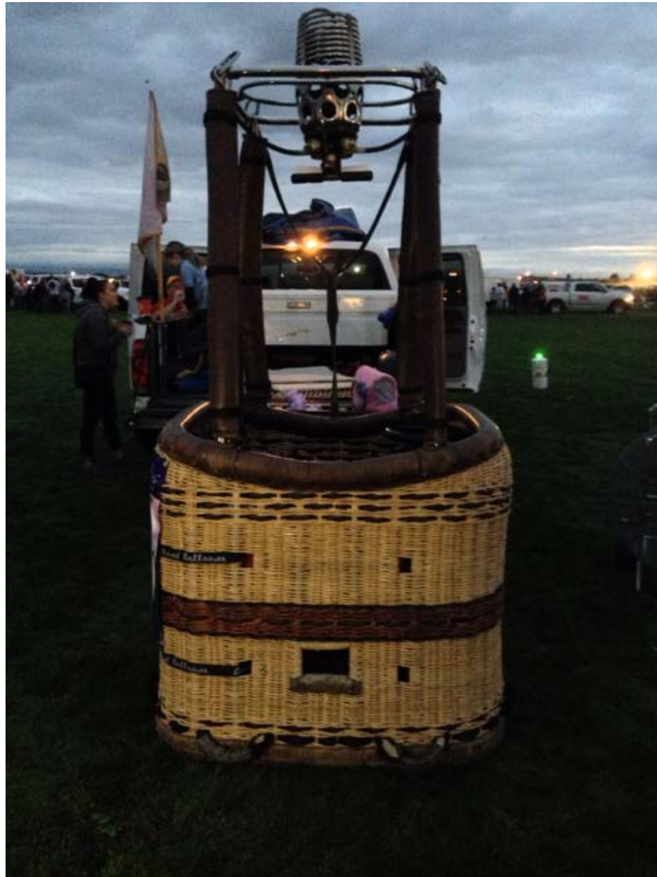
Photo 1 – Accident Balloon Basket with Uprights and Burner
