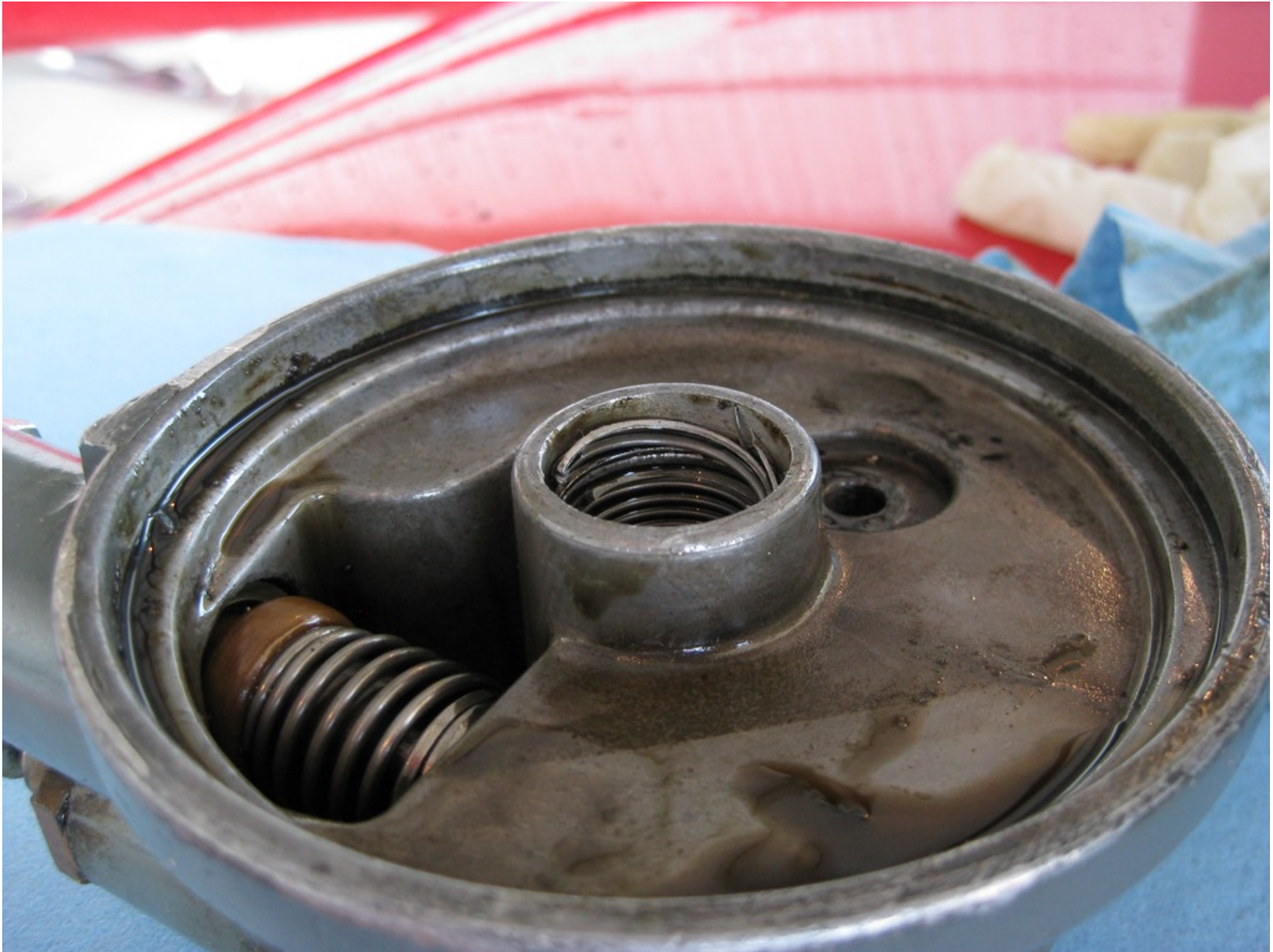
Photo 2 – Damaged Heli-Coil Insert Threads
