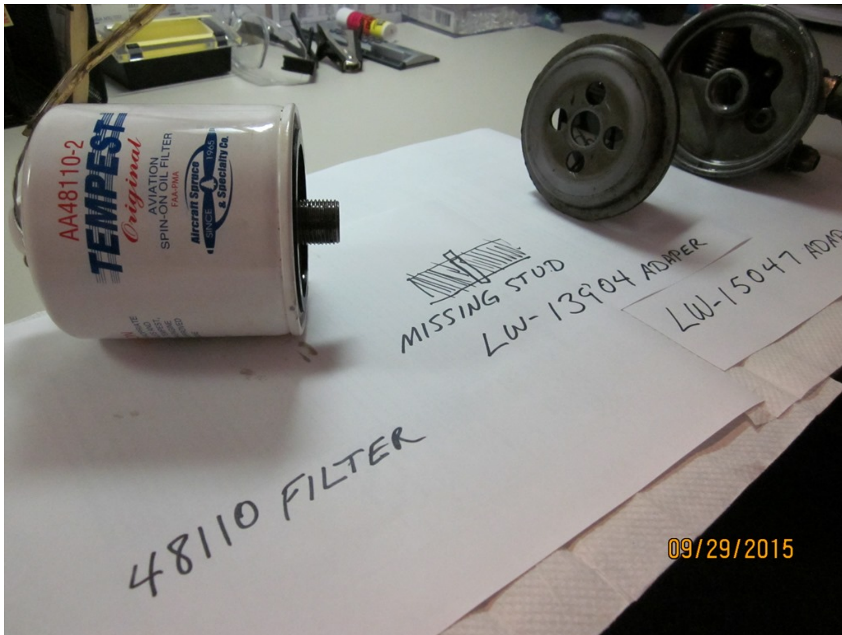
Photo 1 – Oil Filter Adapter Assembly Component Layout
