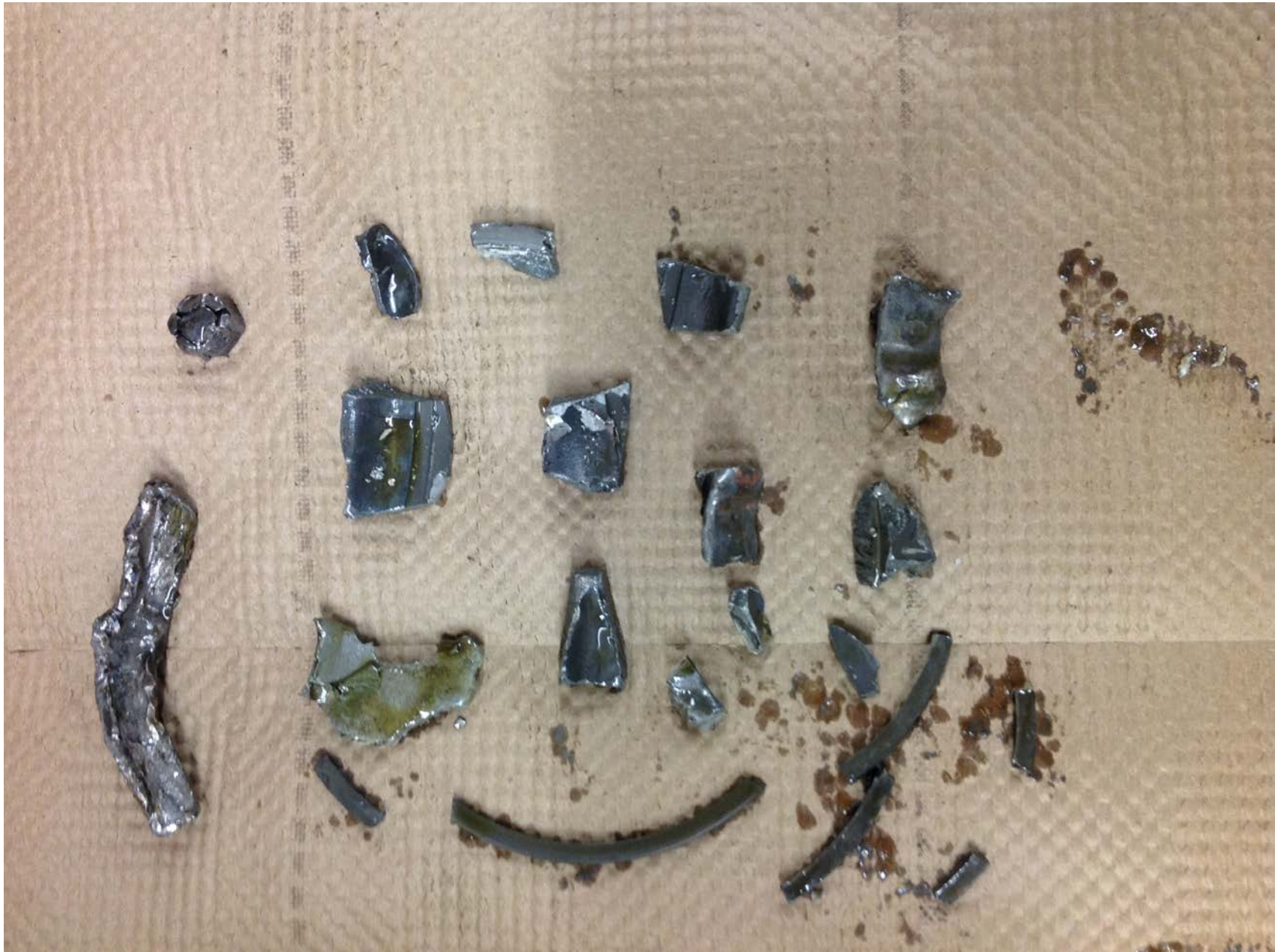
Photo 3 – Debris contents of the engine oil sump
