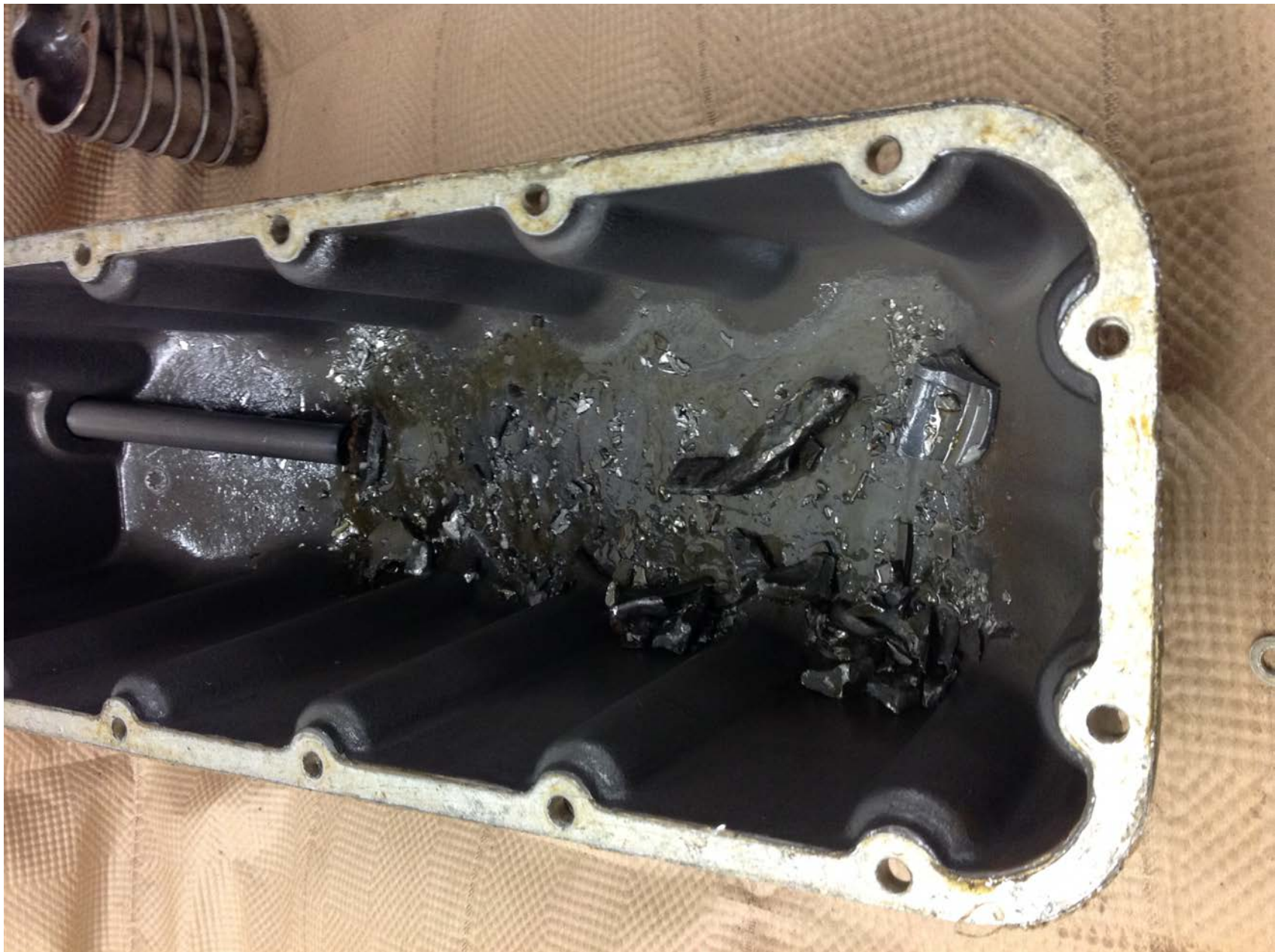
Photo 2 – Engine oil sump with visible debris
