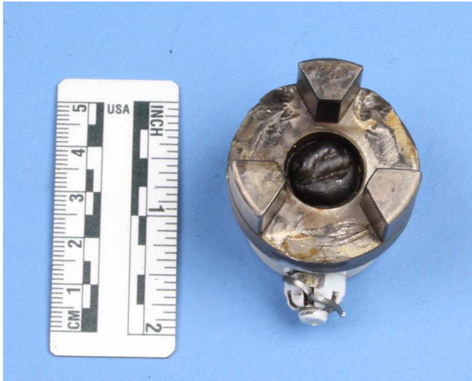
Figure 2: Jaw side of coupling exhibiting dents and gouges.
