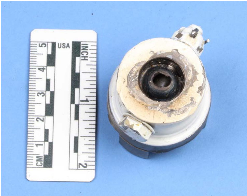
Figure 3: Bore side of coupling with a portion of the driveshaft visible.
