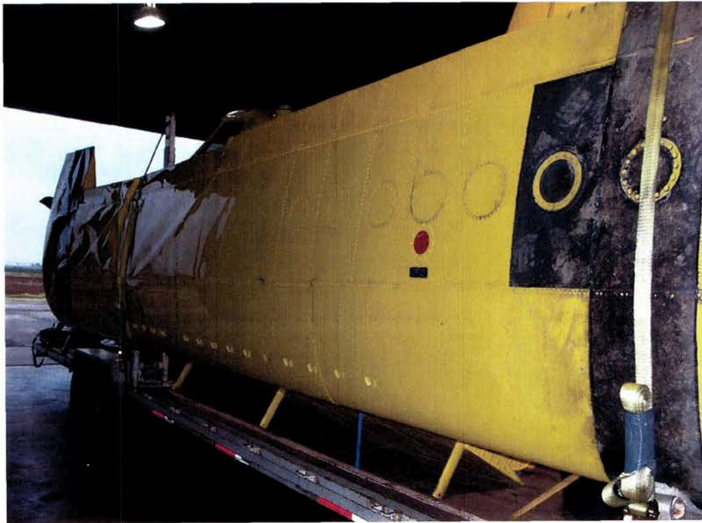
Damage to Righthand Wing
