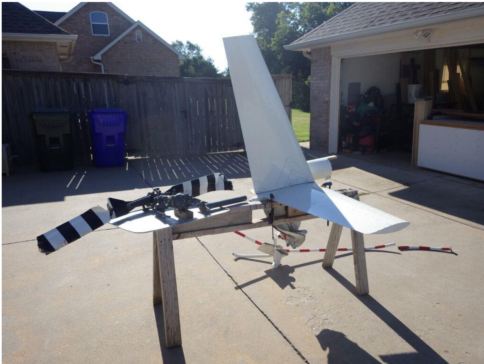
Photo 7 – View of the mockup of the tail rotor and empennage
