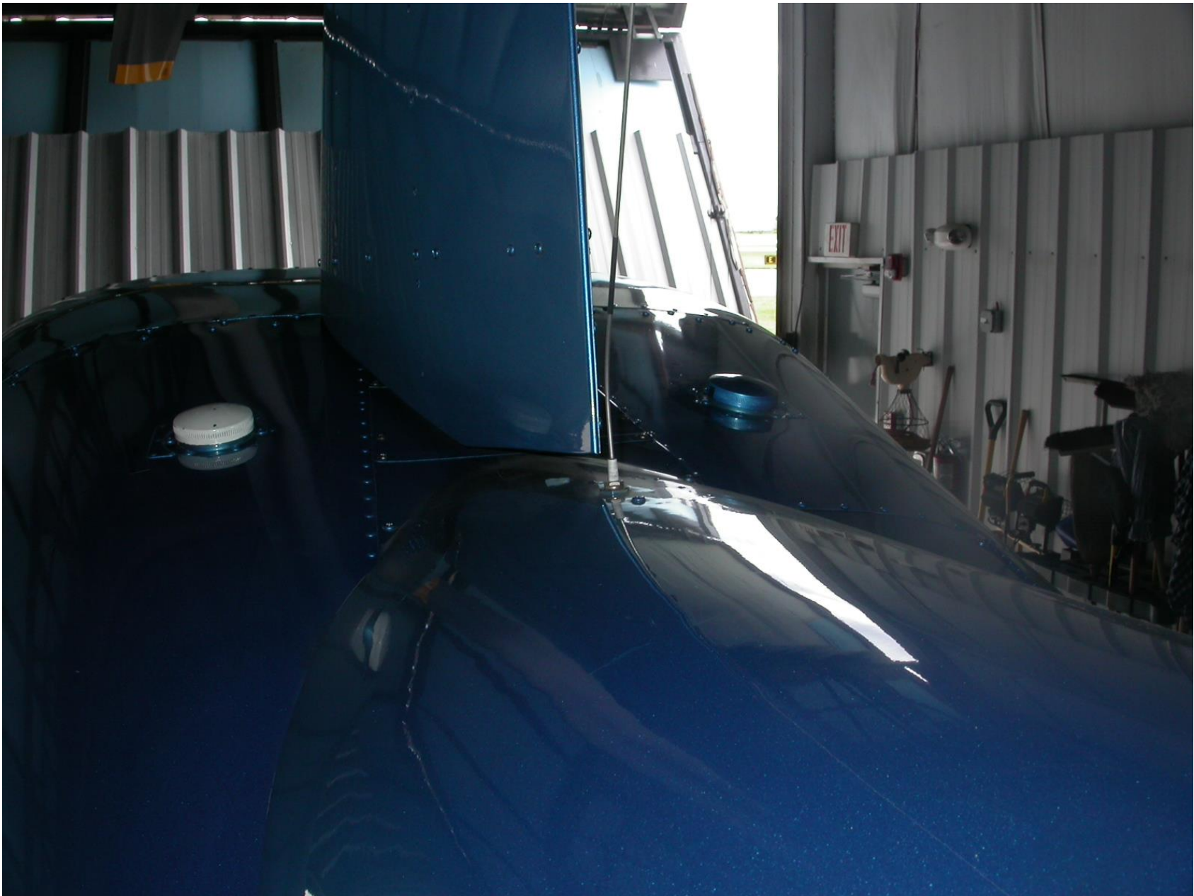
Photo 15 – Accident fuel cap installed on exemplar R-44
