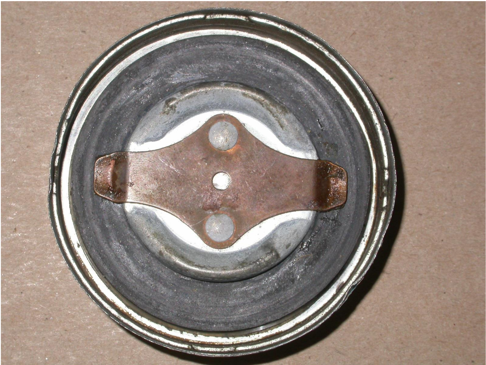
Photo 14 – View of the underside of the fuel cap
