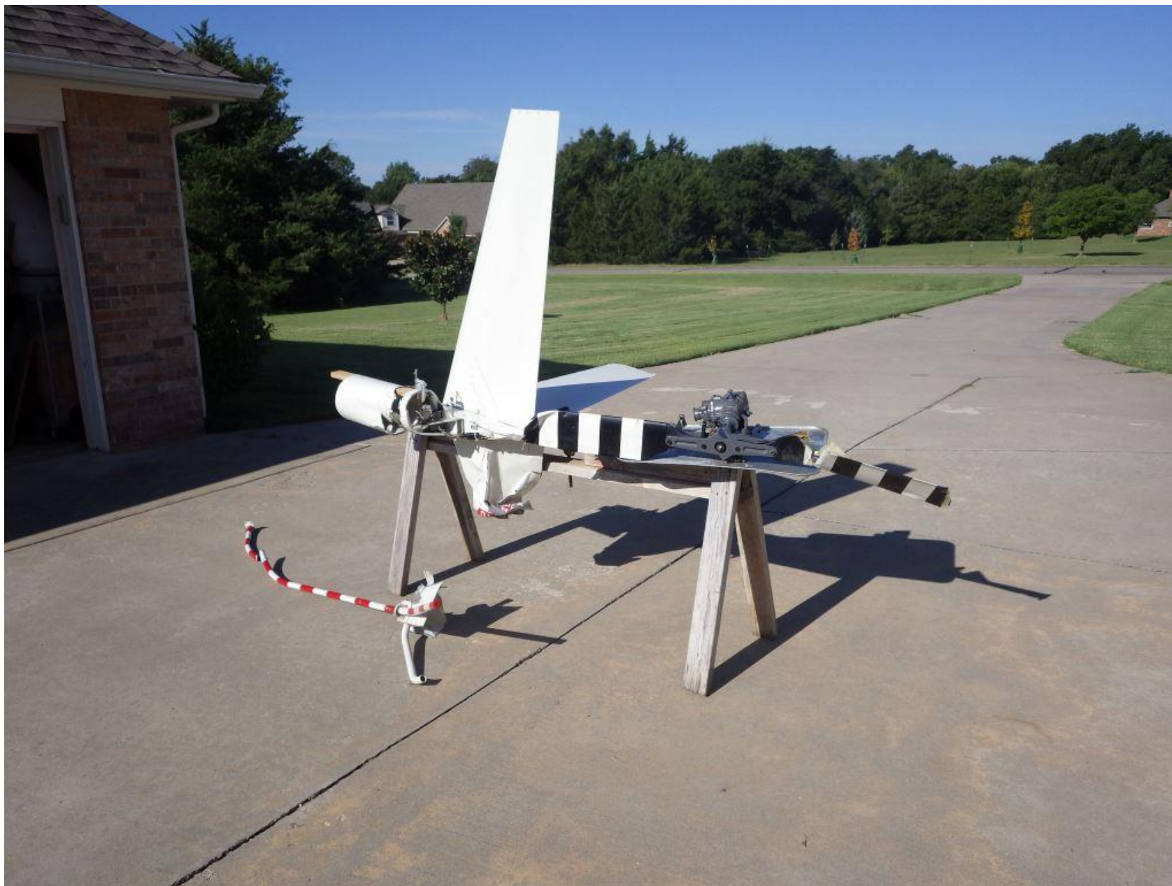
Photo 6 – A mockup of the empennage and tail rotor gearbox and tail rotor blades
