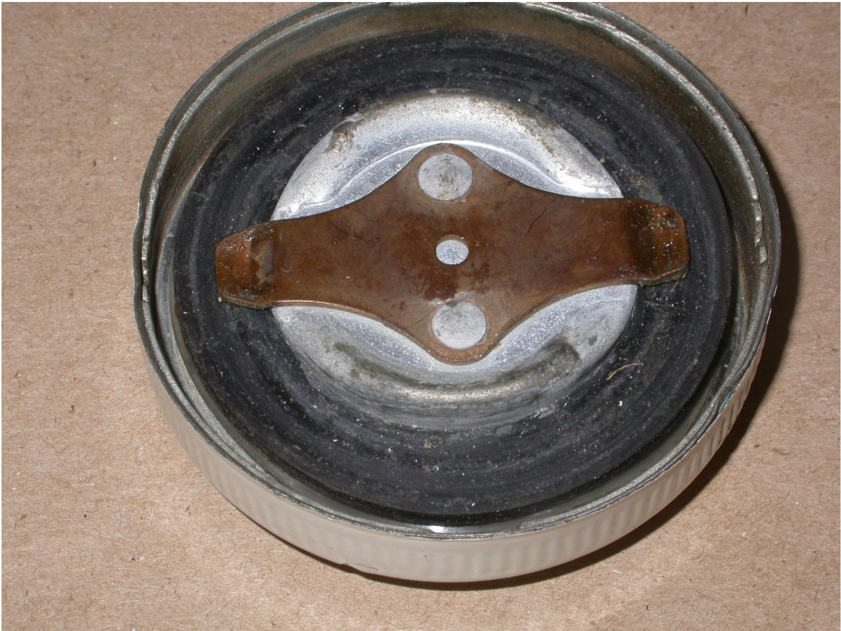
Photo 13 – View of the underside of the fuel cap
