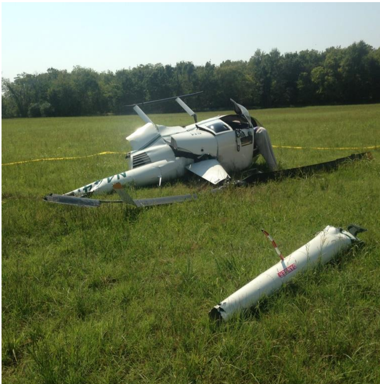
Photo 11 – View of about a 6 ft section of the tail boom at the main wreckage site
