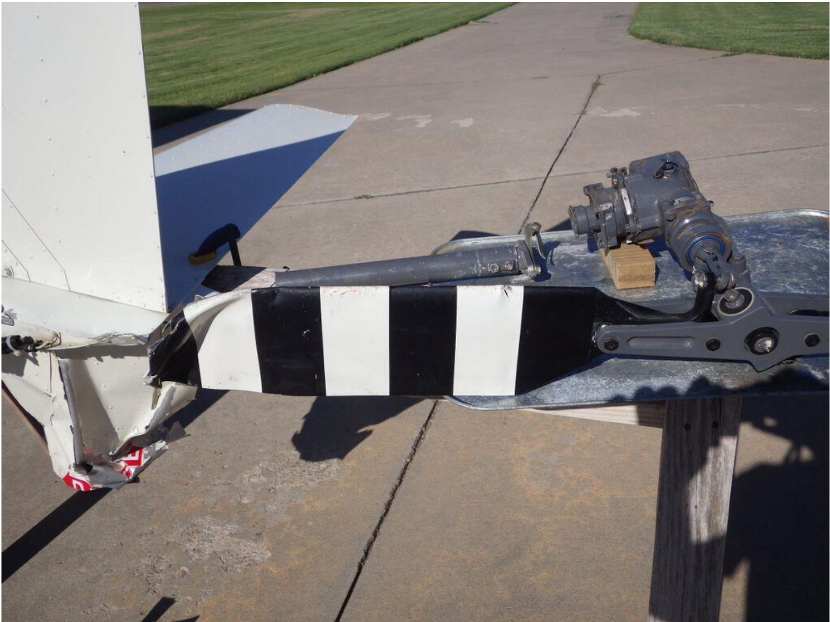
Photo 9 – View of tail rotor gearbox and one of the tail rotor blades
