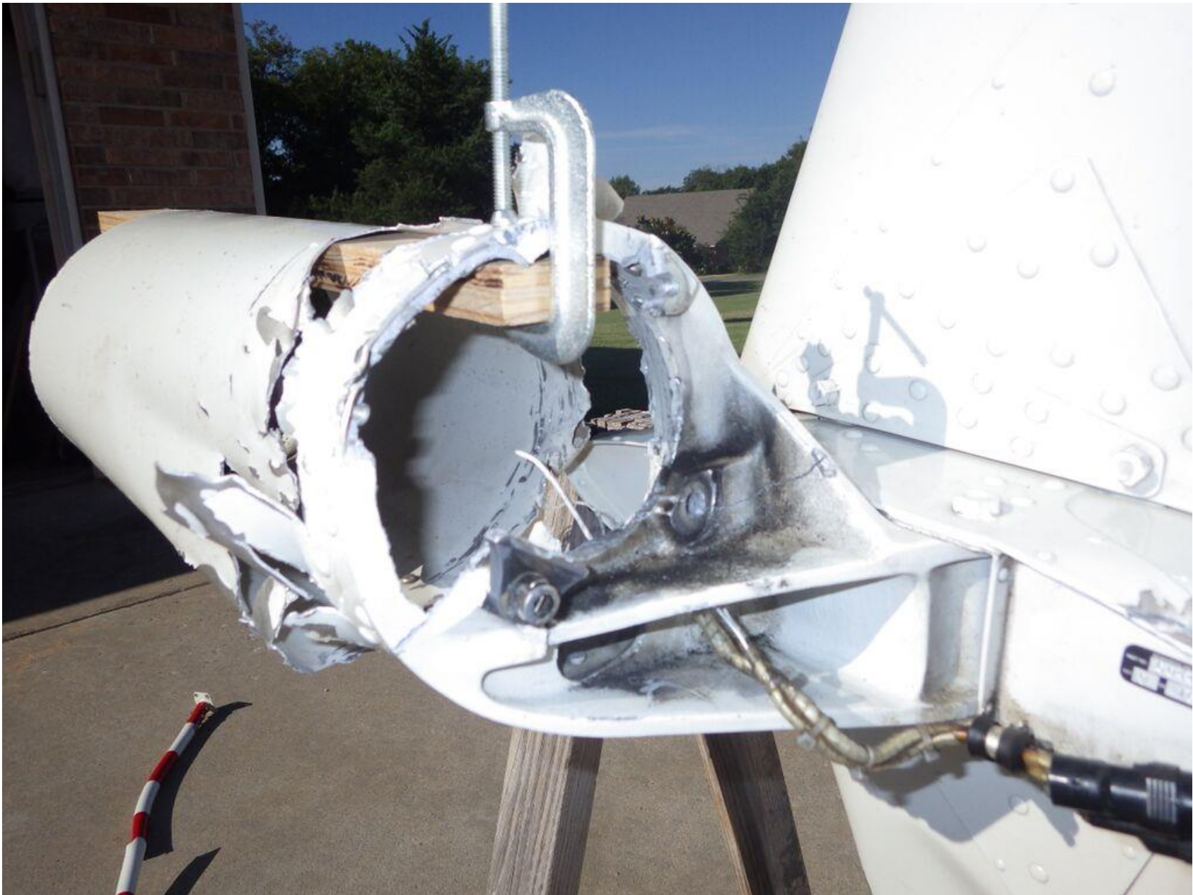
Photo 8 – View of the tail boom where the tail rotor gearbox was attached
