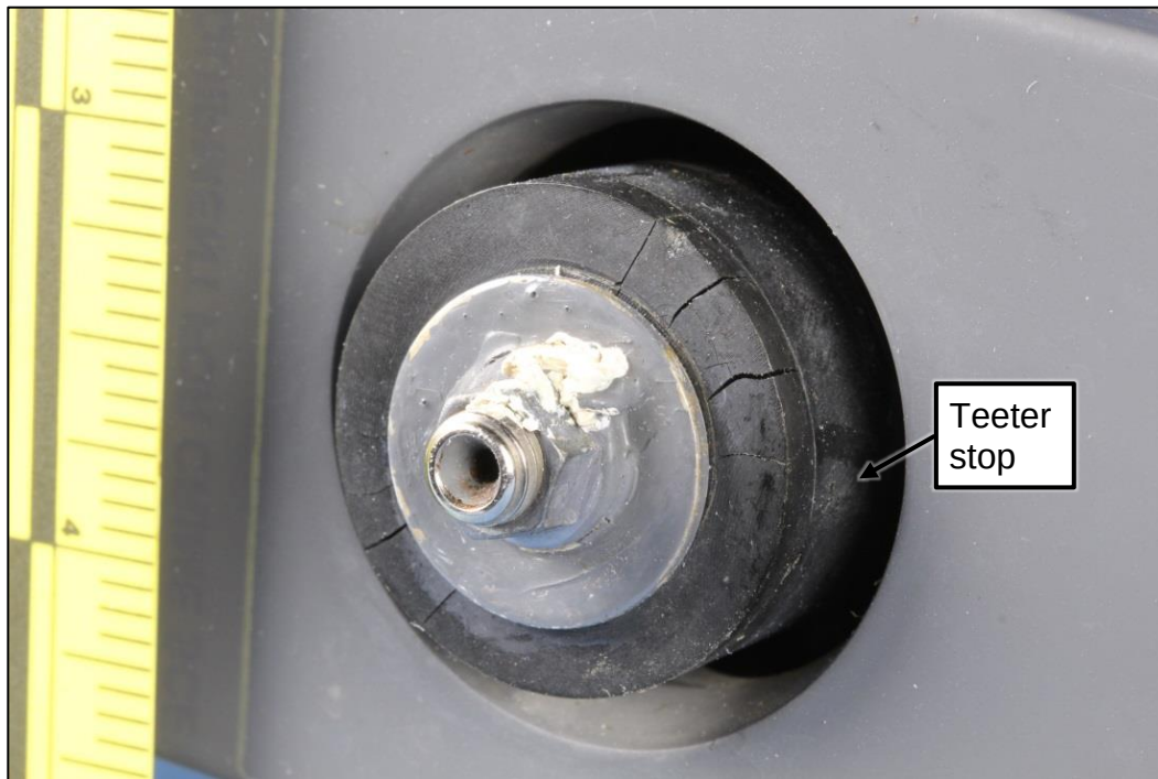
Figure 9. Close view of the teeter stop. The stop was deformed corresponding to contact with the hub, and radial cracks were present adjacent to the contact area.
