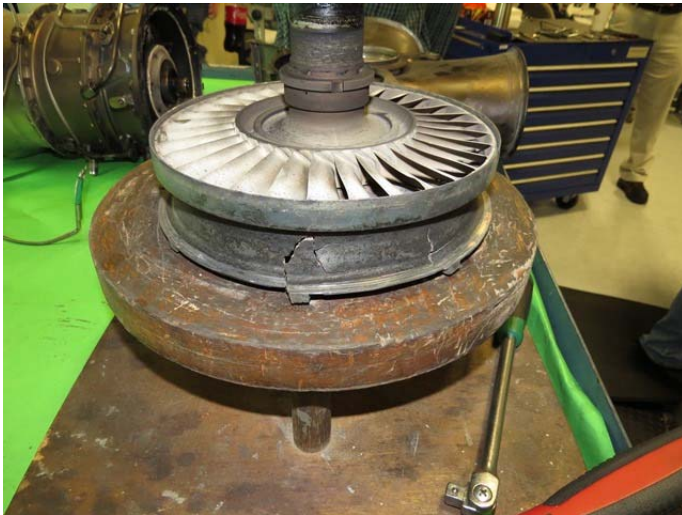
Power Turbine Rotor Stage Four Nozzle and Wheel
