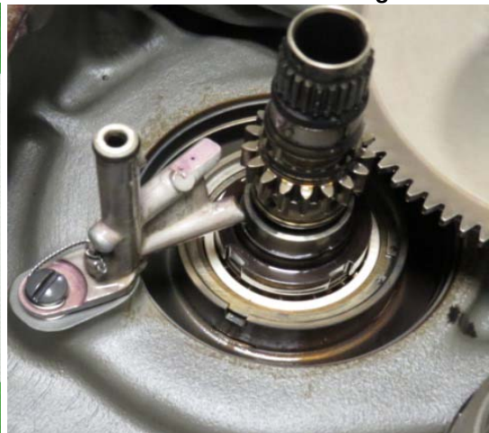
Spur Adapter Gear Shaft in Position
