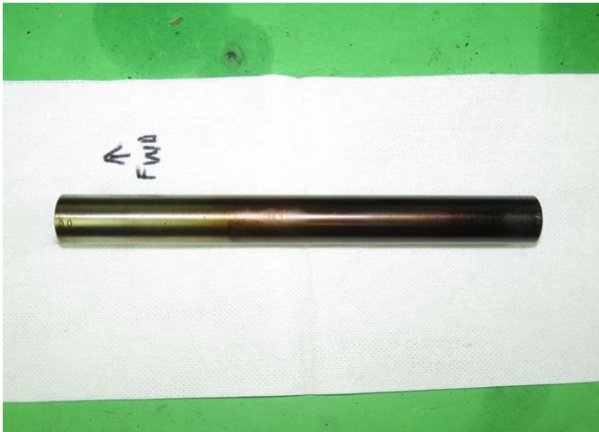
Turbine to Compressor Coupling
