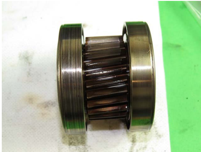
#4 and #3 Bearing on Pinion Gear
