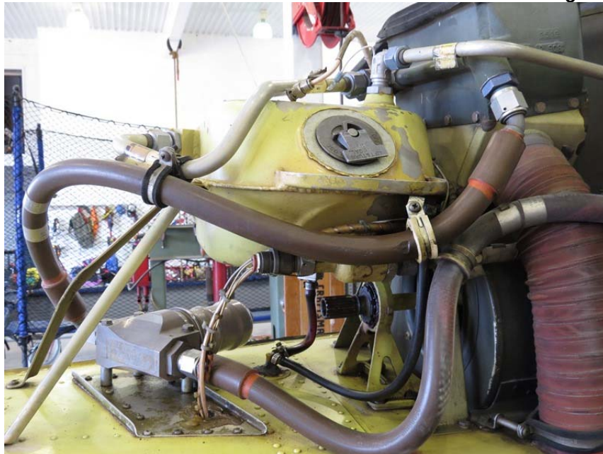
Oil Tank and External Filter
