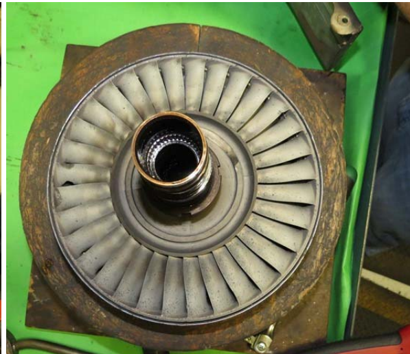
Stage Four Wheel Suction Side
