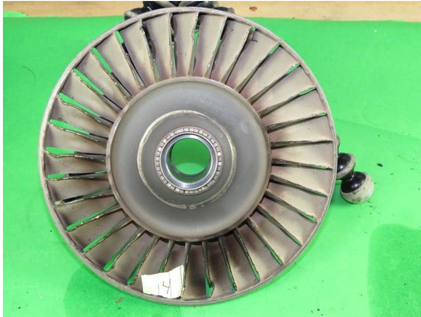
Stage Four Wheel Pressure Side
