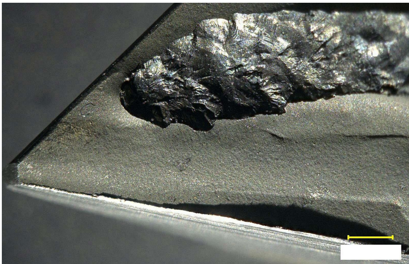
Figure 27. Low angle lighting showing the casting wax weld adjacent to the airfoil No. 22 trailing edge.
