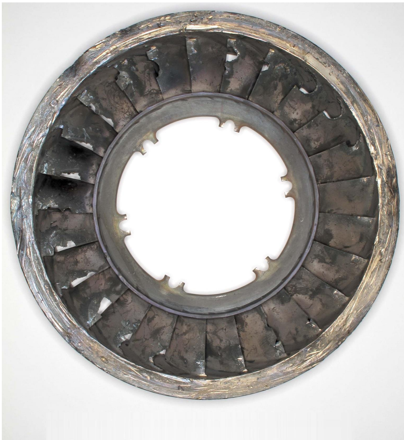
Figure 45. Forward looking aft view of the third stage turbine nozzle showing the damage to the trailing edge vane surfaces.
