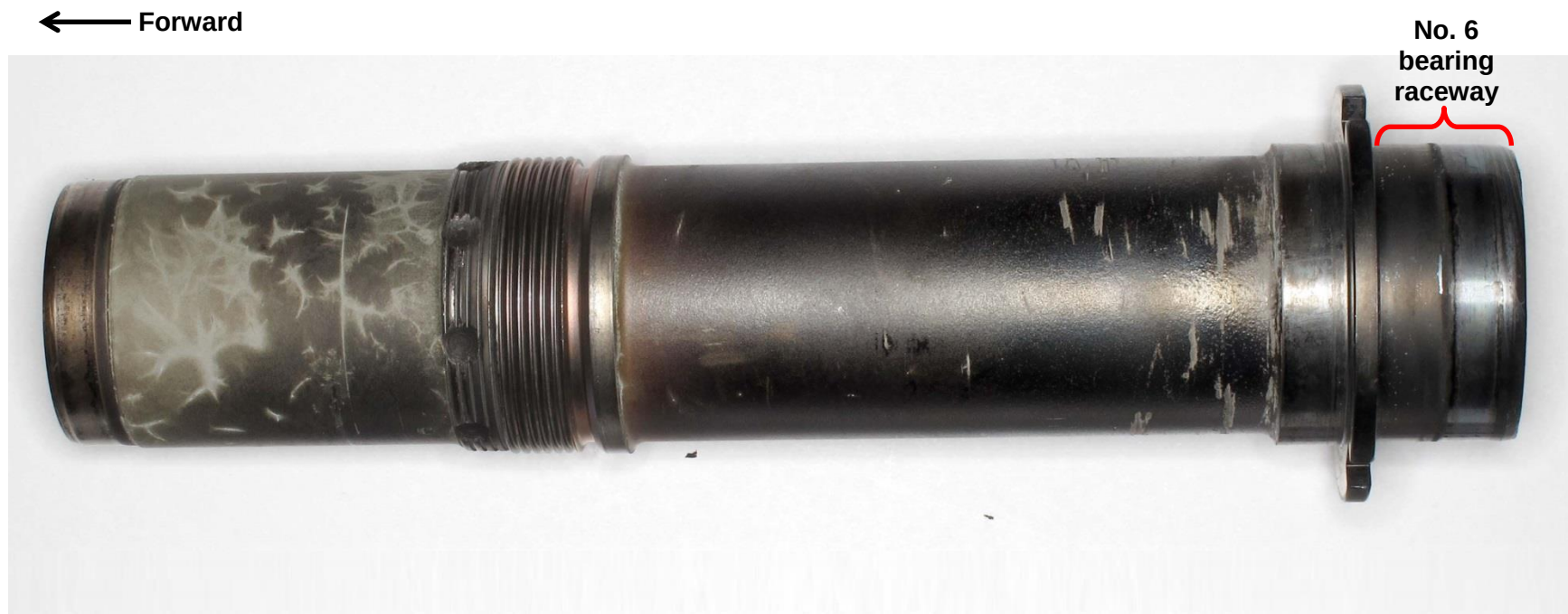
Figure 73. Photograph of the power turbine inner shaft.
