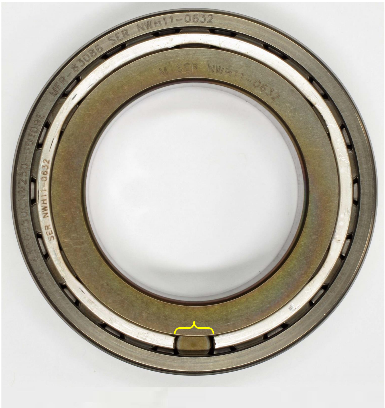
Figure 62. Aft looking forward view of the No. 4 bearing. The bracket highlights the portion of the separator that fractured.
