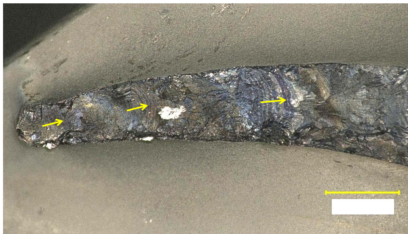
Figure 20. Photographs showing the fractured third stage turbine wheel airfoil No. 3.
