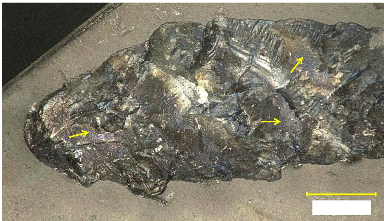
Figure 26. Photographs showing the fractured third stage turbine wheel airfoil No. 22.
