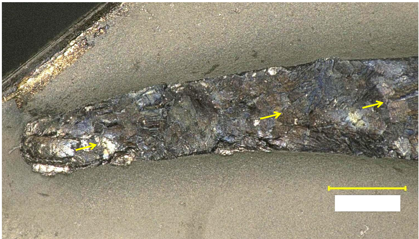
Figure 32. Photographs showing the fractured third stage turbine wheel airfoil No. 24.
