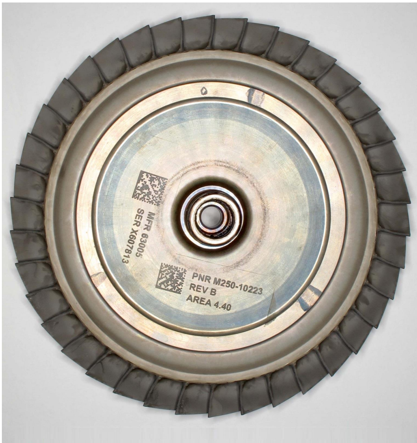
Figure 69. Aft looking forward view of the first stage turbine wheel.
