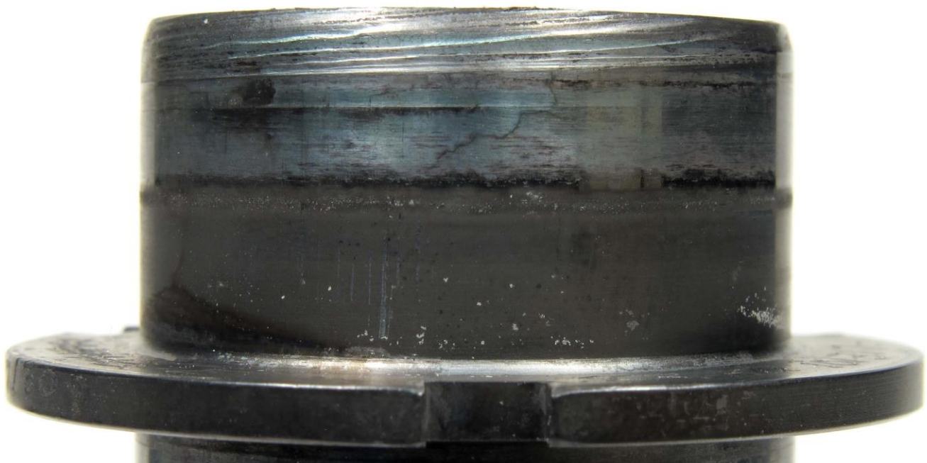
Figure 75. Photographs showing the damage to the ID surface at the aft end of the power turbine inner shaft (upper image). The lower image shows the condition of the No. 6 bearing inner ring raceway.
