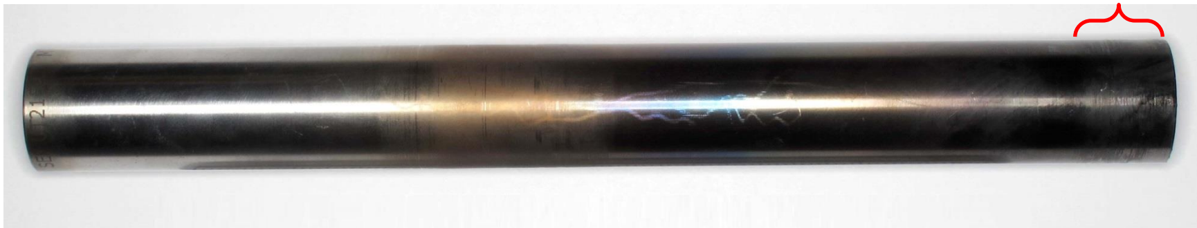
Figure 77. Photographs of the turbine to compressor coupling showing the scoring damage on the aft end OD surface.
