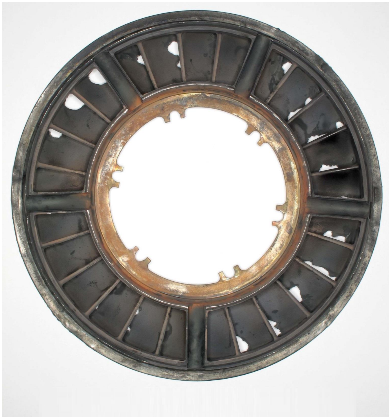
Figure 44. Aft looking forward view of the third stage turbine nozzle.
