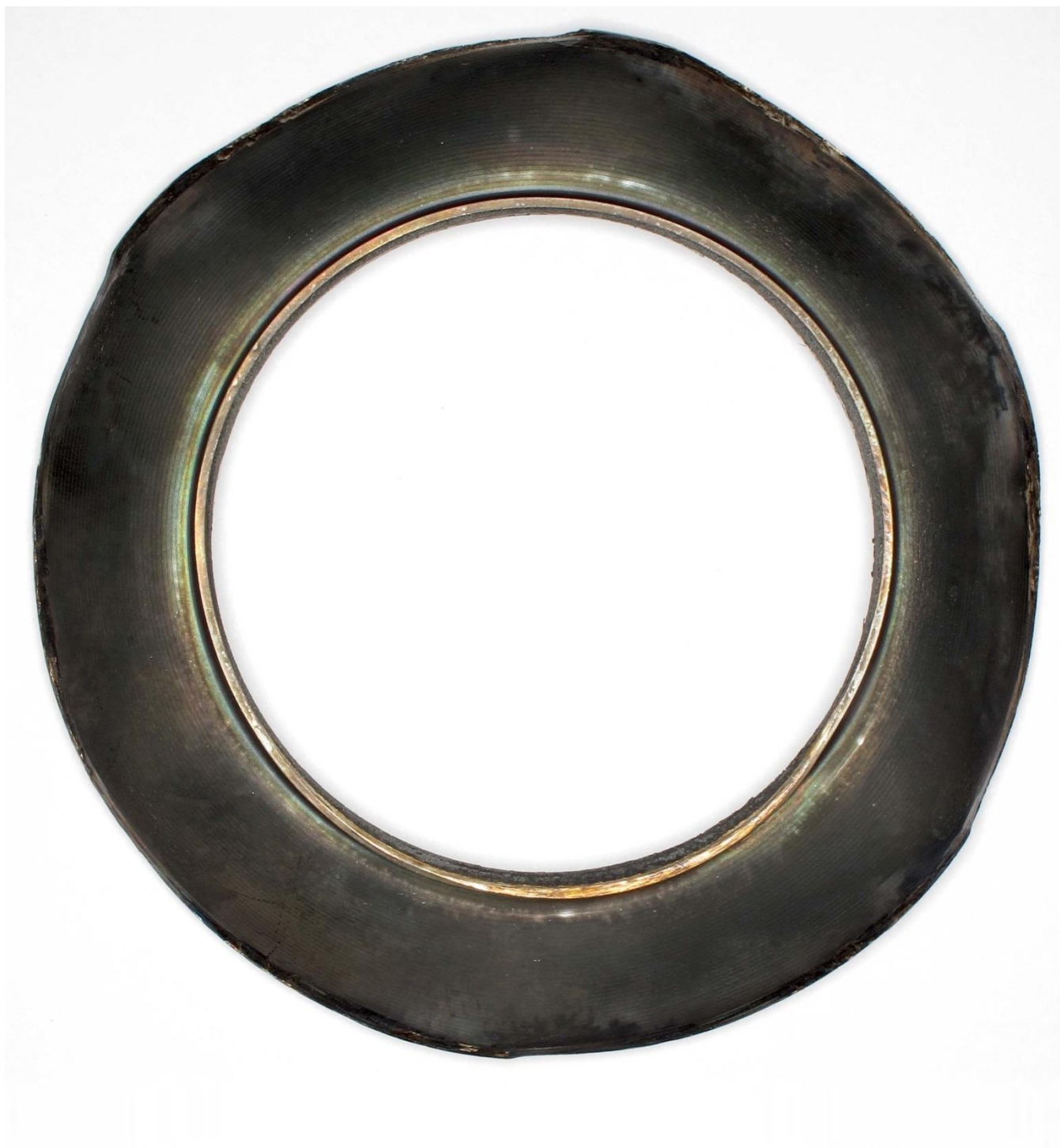
Figure 51. Photograph of the diaphragm that detached from the bore of the fourth stage turbine nozzle (forward looking aft view).
