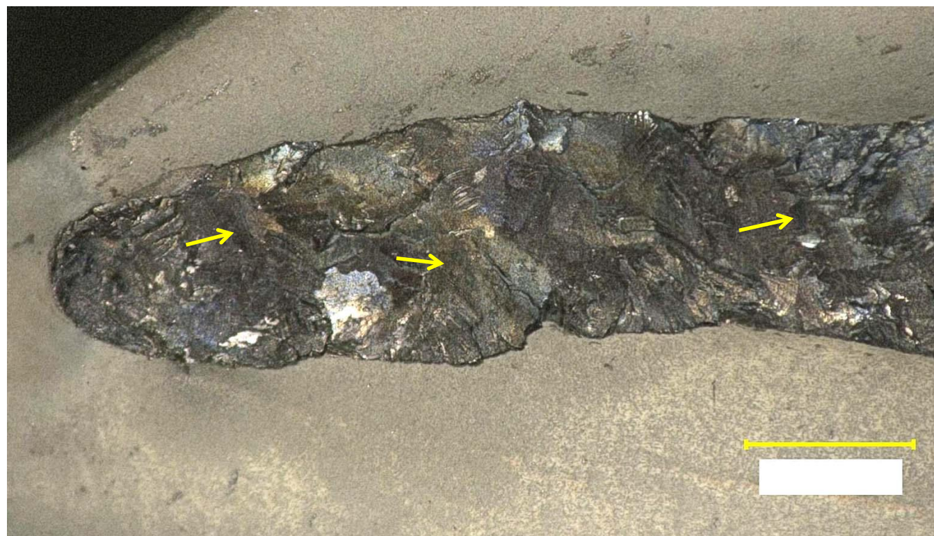
Figure 14. Photographs showing the fractured third stage turbine wheel airfoil No. 2.
