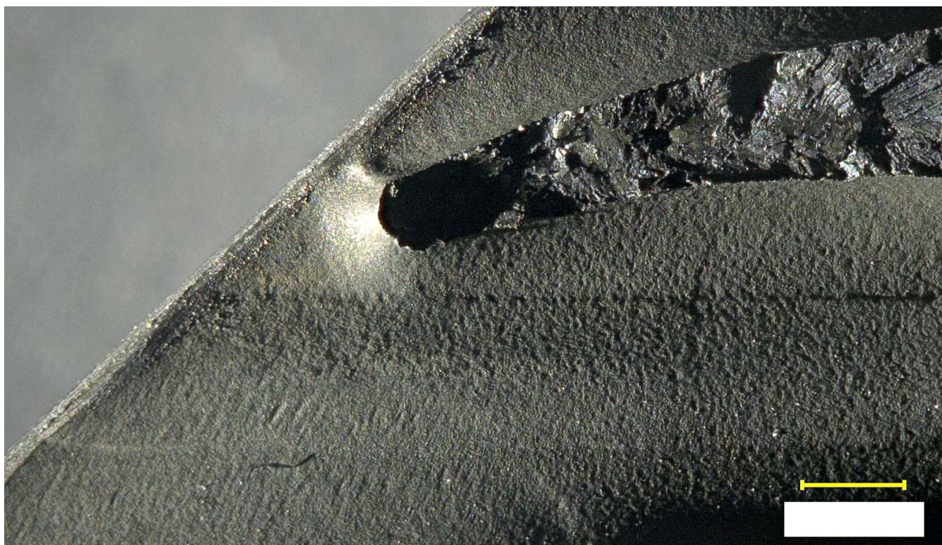
Figure 33. Low angle lighting showing the casting wax weld adjacent to the airfoil No. 24 trailing edge.
