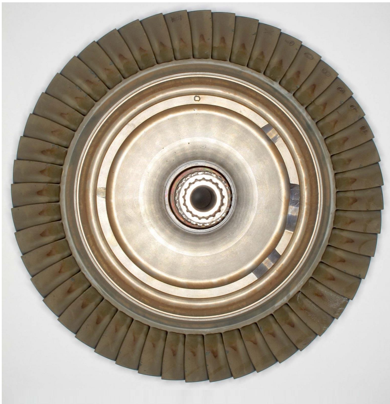
Figure 70. Forward looking aft view of the second stage turbine wheel.
