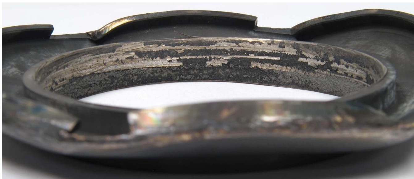
Figure 52. Detailed views showing the rub damage to the bore of the fourth stage turbine wheel diaphragm.
