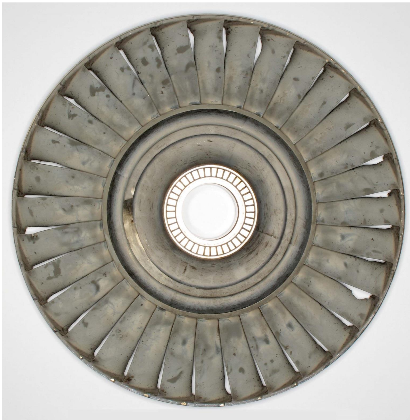
Figure 54. Forward looking aft view of the fourth stage turbine wheel.
