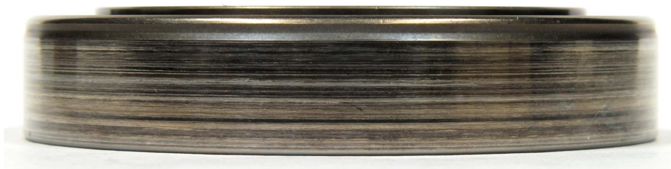
Figure 64. Photograph of the outer ring OD surface showing circumferential score marks.
