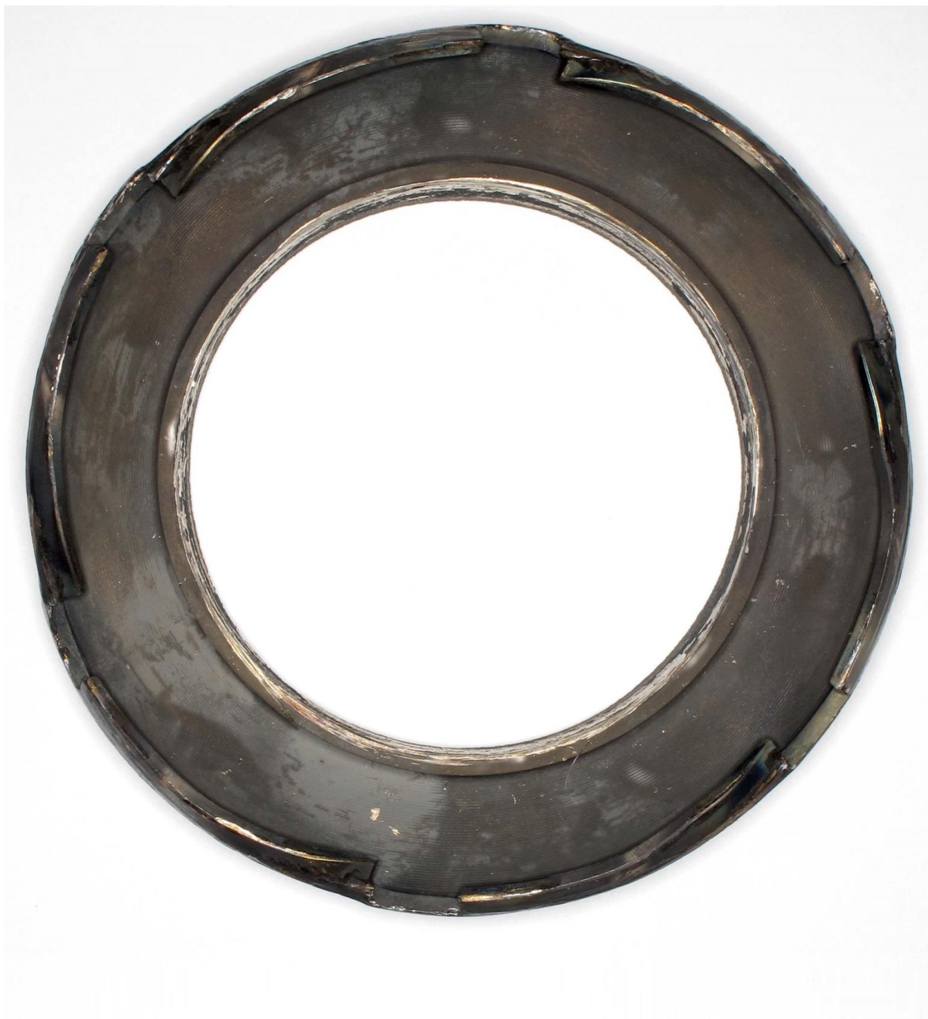
Figure 50. Photograph of the diaphragm that detached from the bore of the fourth stage turbine nozzle (aft looking forward view).
