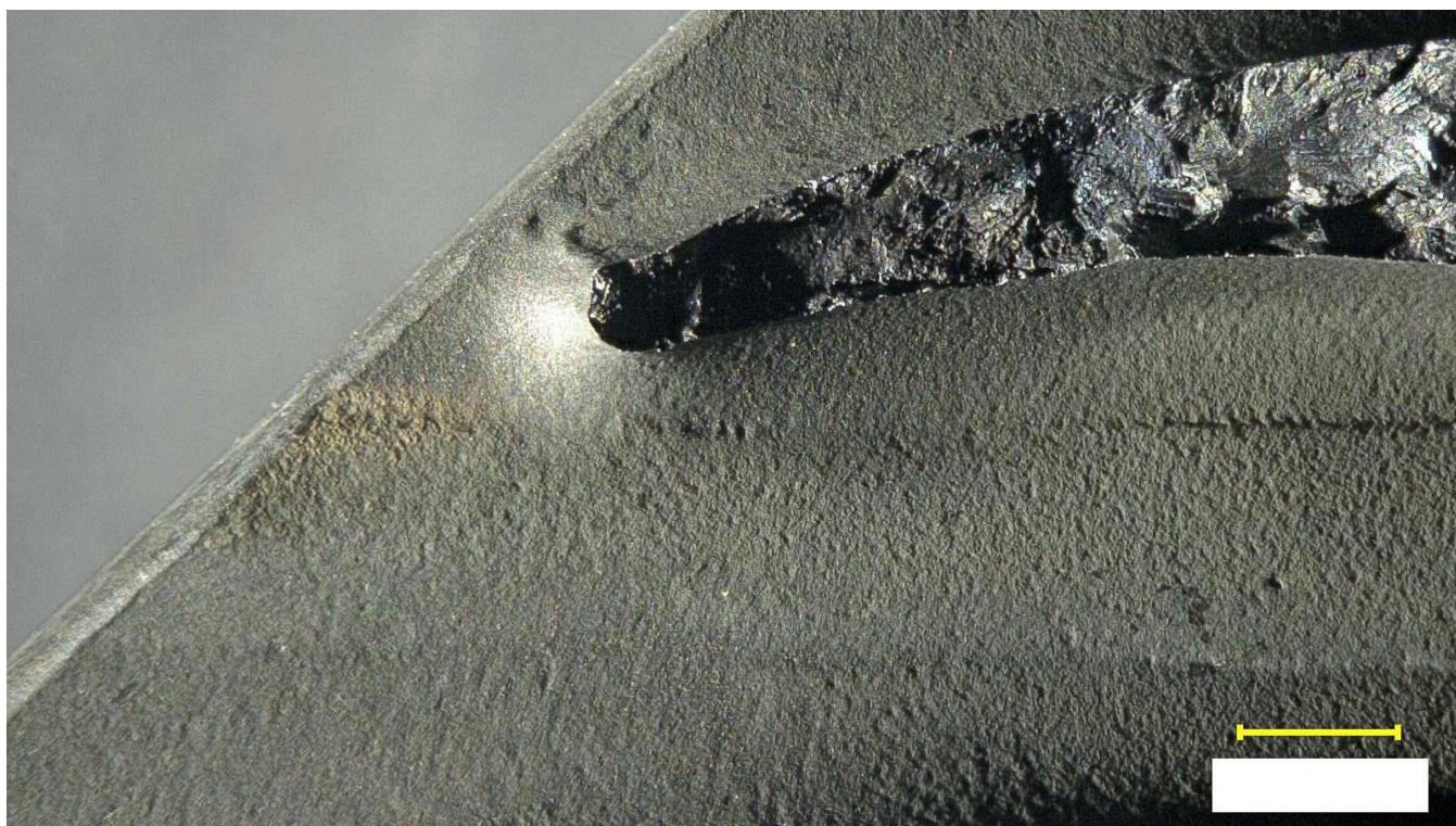
Figure 21. Low angle lighting showing the casting wax weld adjacent to the airfoil No. 3 trailing edge.
