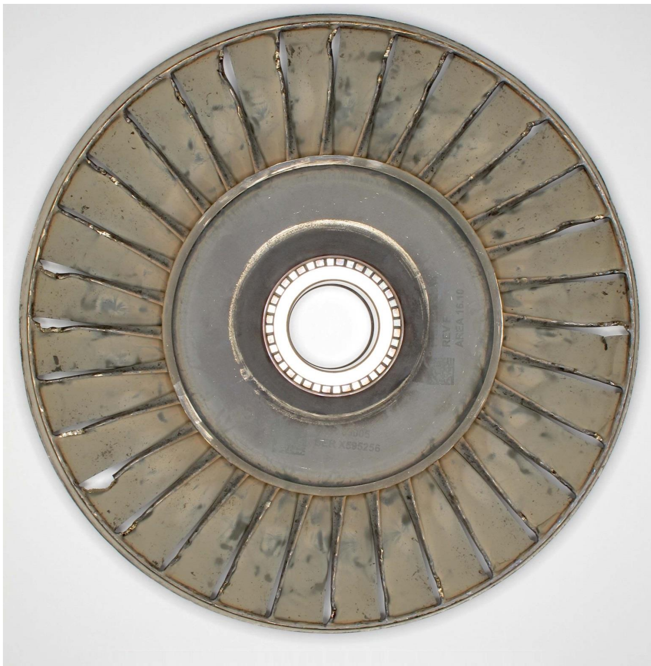
Figure 53. Aft looking forward view of the fourth stage turbine wheel. Note the damage to the airfoil leading edge surfaces.
