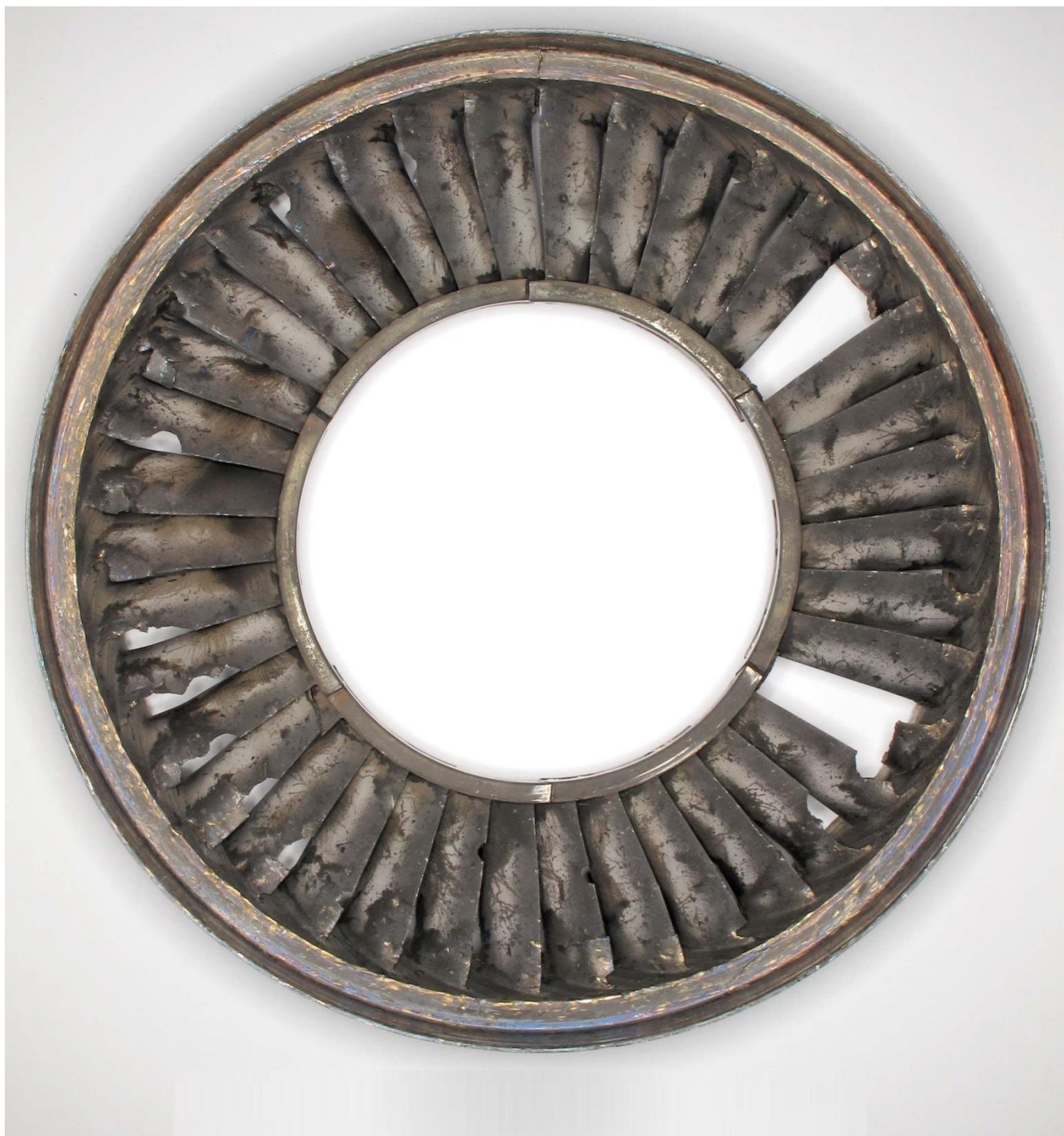
Figure 47. Forward looking aft view of the fourth stage turbine nozzle assembly showing the damage to the vane trailing edge surfaces.
