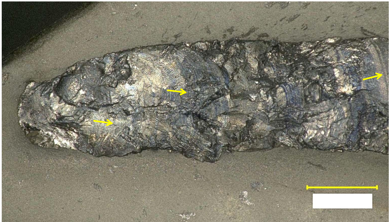
Figure 8. Photographs showing the fractured third stage turbine wheel airfoil No. 1.
