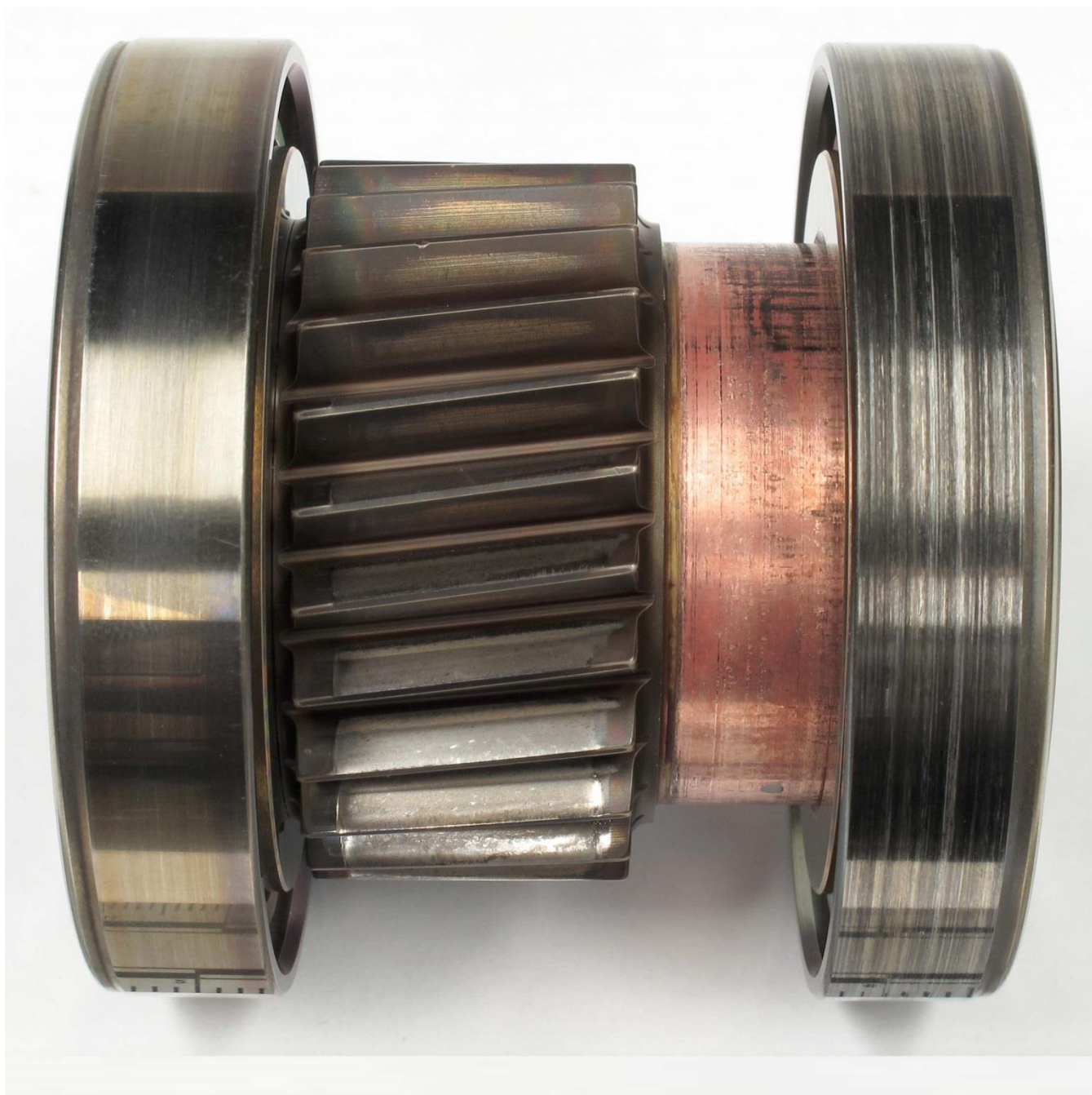
Figure 61. Photograph of the No. 3 bearing, pinion gear, and No. 4 bearing (after removal from the pinion gear).
