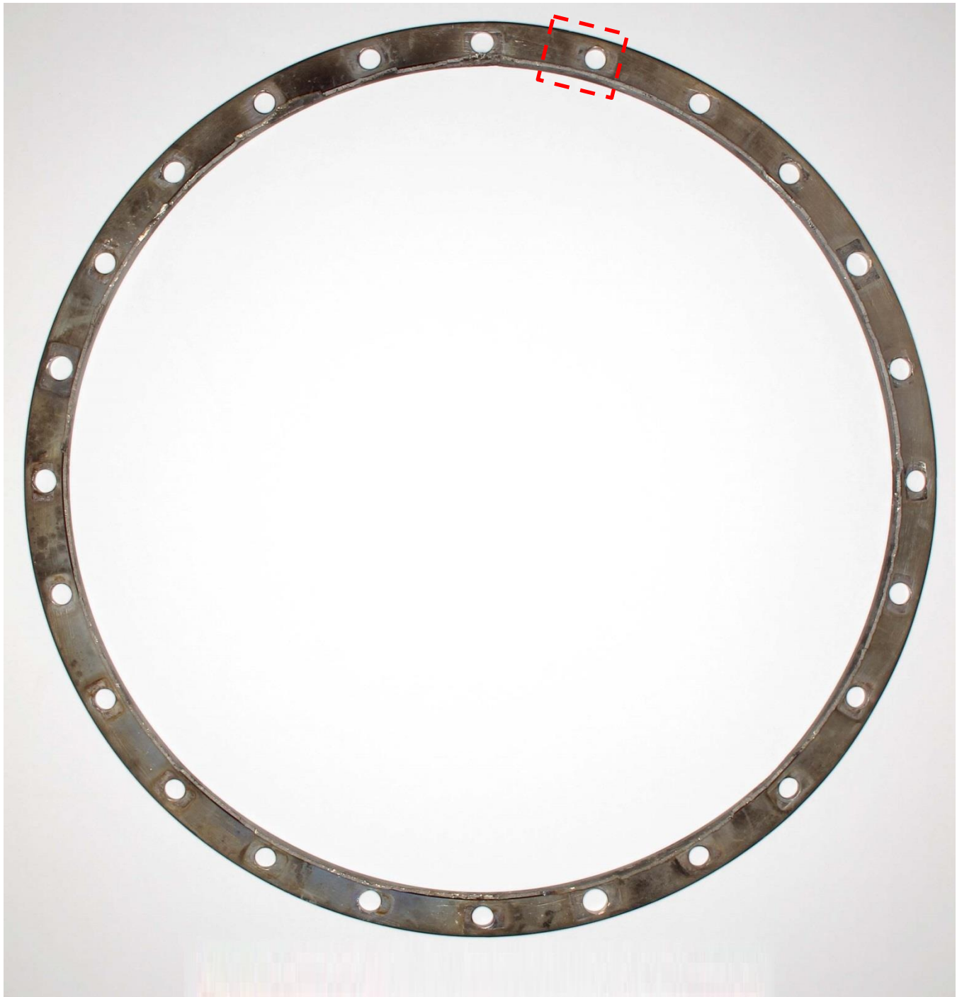
Figure 55. Forward looking aft view of the fractured exhaust collector flange. Detailed photographs of the boxed area are shown in the following figures.
