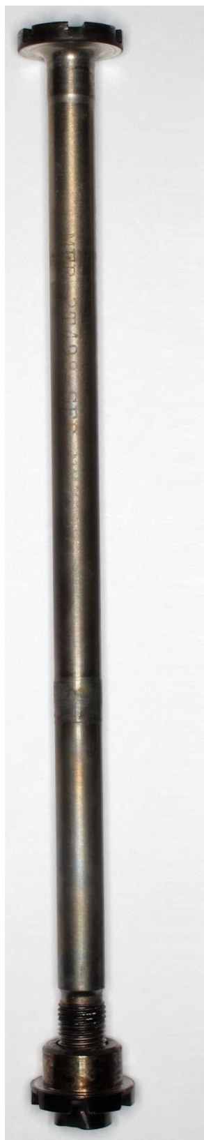
Figure 71. Photograph of the turbine tie bolt and nut.
