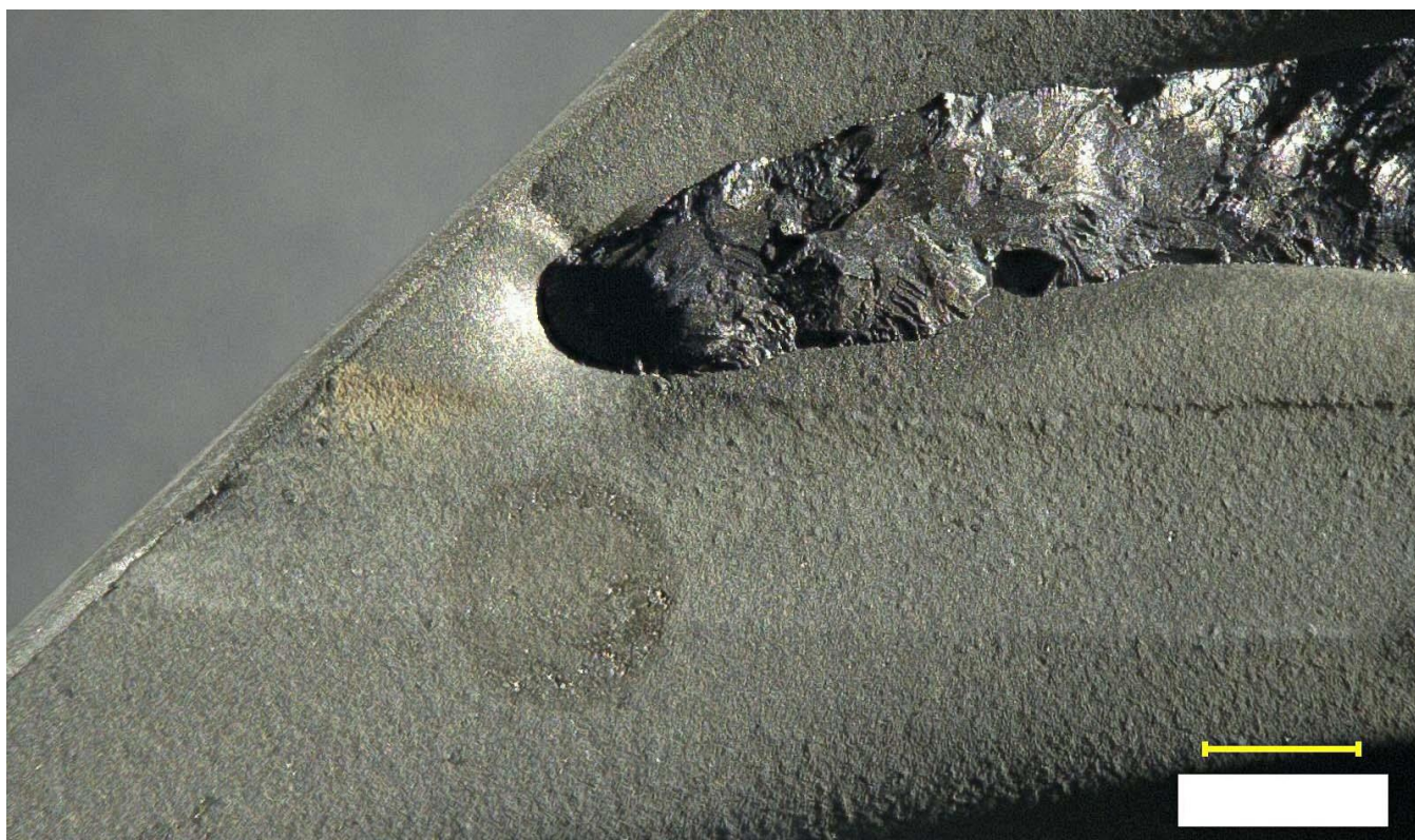
Figure 15. Low angle lighting showing the casting wax weld adjacent to the airfoil No. 2 trailing edge.
