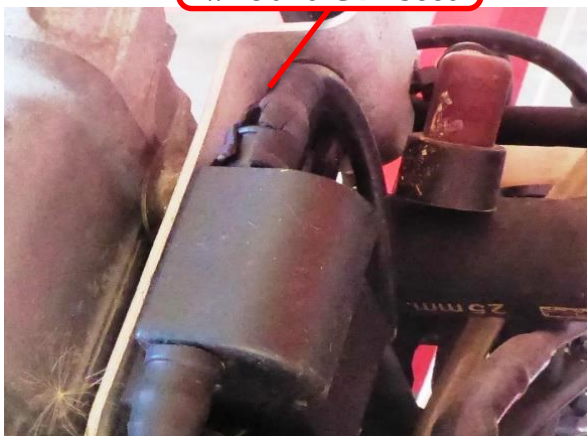
Crack in Ignition wire and CDI boot
