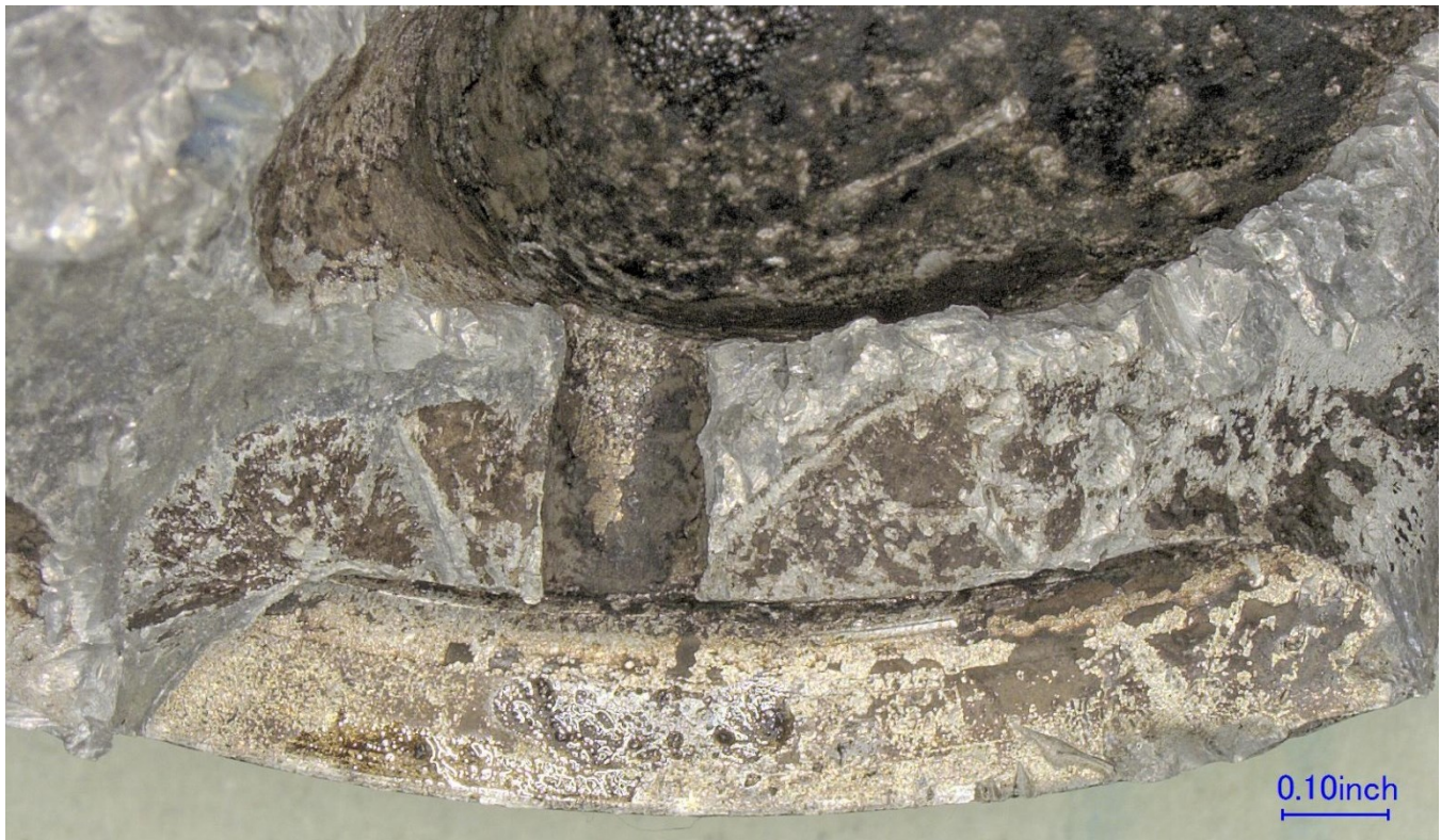
Figure 9 – Closer view of fatigue crack B, as labeled on Figure 1.
