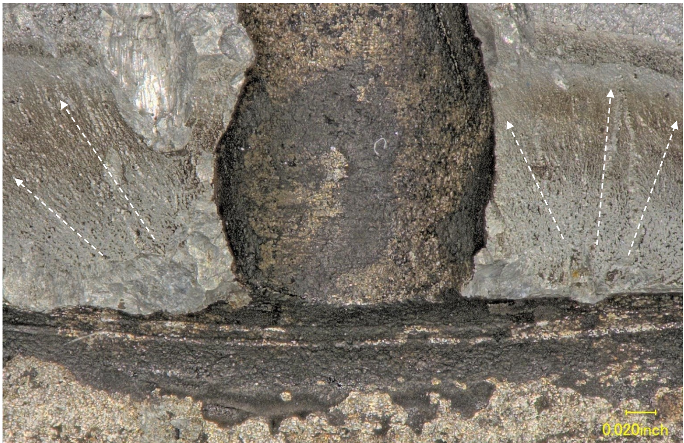
Figure 3 – Closer view of the oil hole from Figure 2, showing the crack initiation sites. The arrows denote crack direction.
