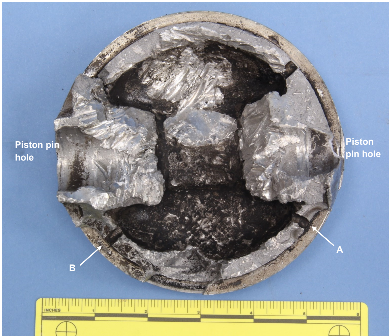
Figure 1 – The underside of the piston crown, as received. The two fatigue cracks are highlighted at the oil drain holes (arrows) where they were located.
