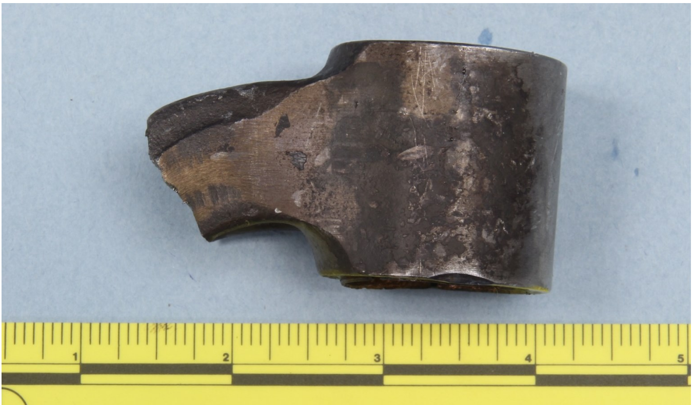
Figure 16 – The connecting rod fragment that was attached to the piston pin, after cleaning and disassembly.
