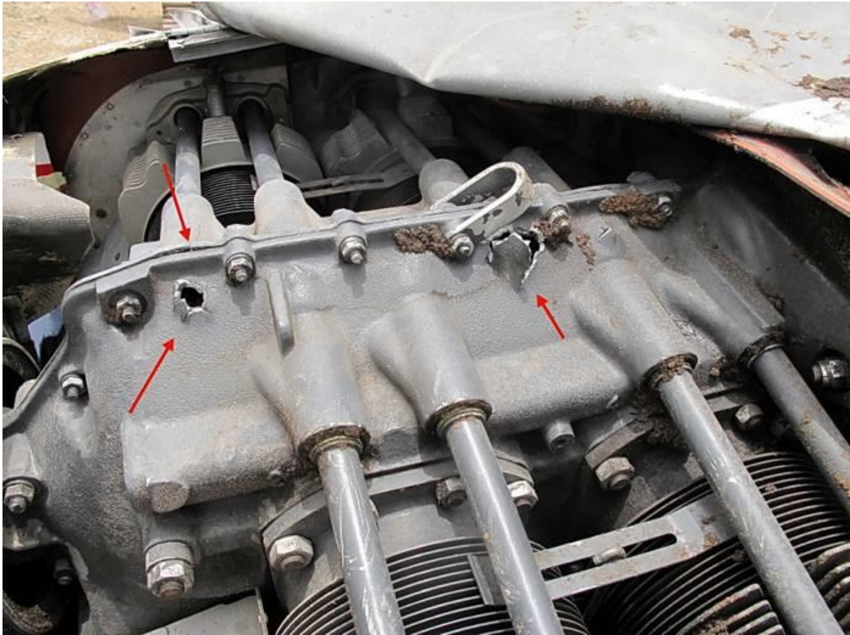
Photo 1 – engine showing 2 holes in crank case
