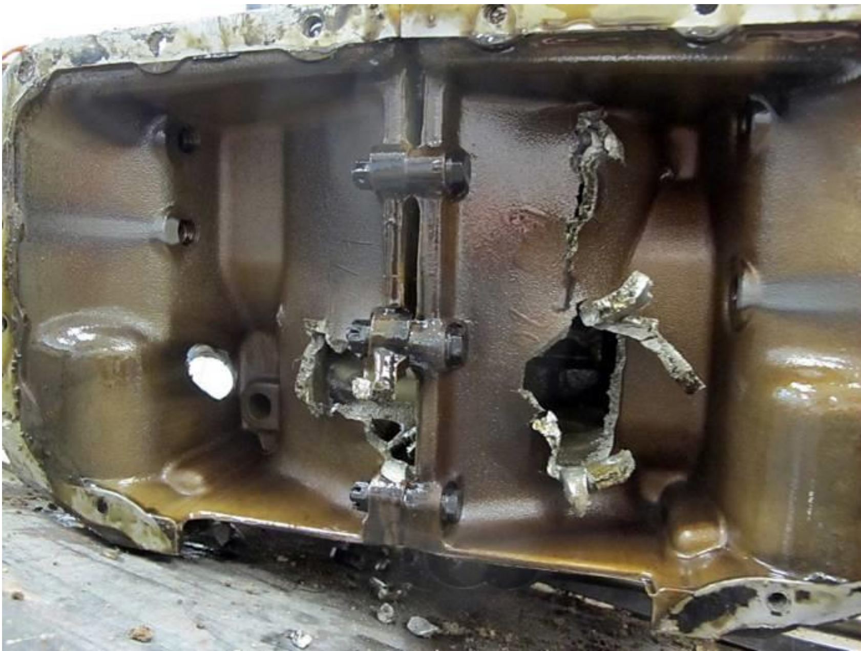
Photo 2 – view of damage to crankcase
