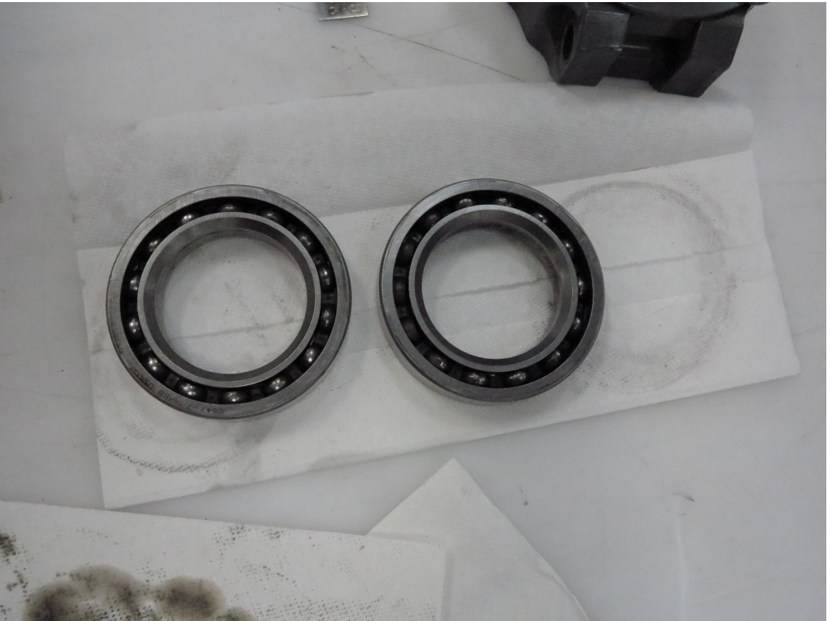
Sheave support bearings.
