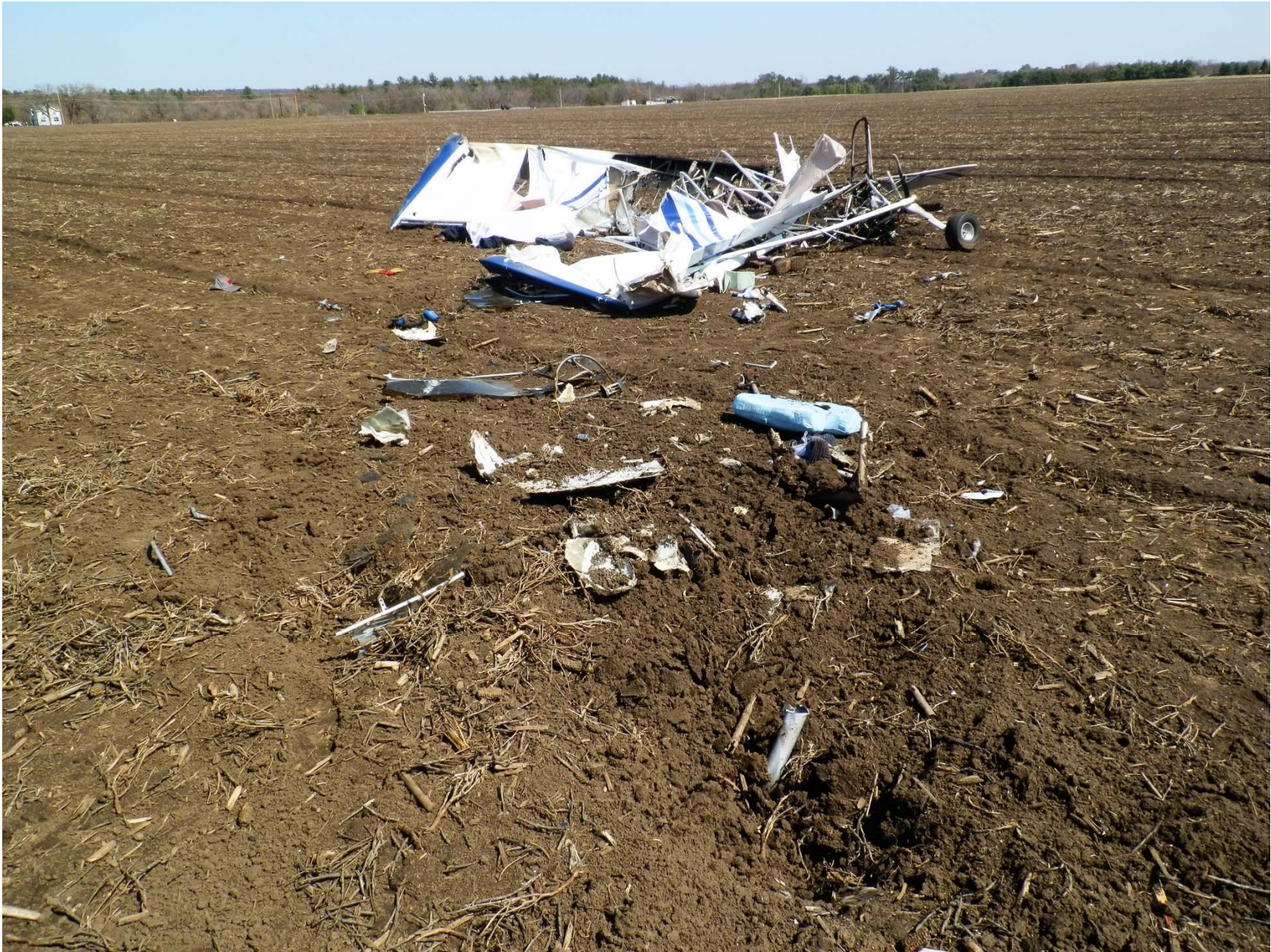
Photo of airplane at accident site, with the initial impact point and debris in the foreground
