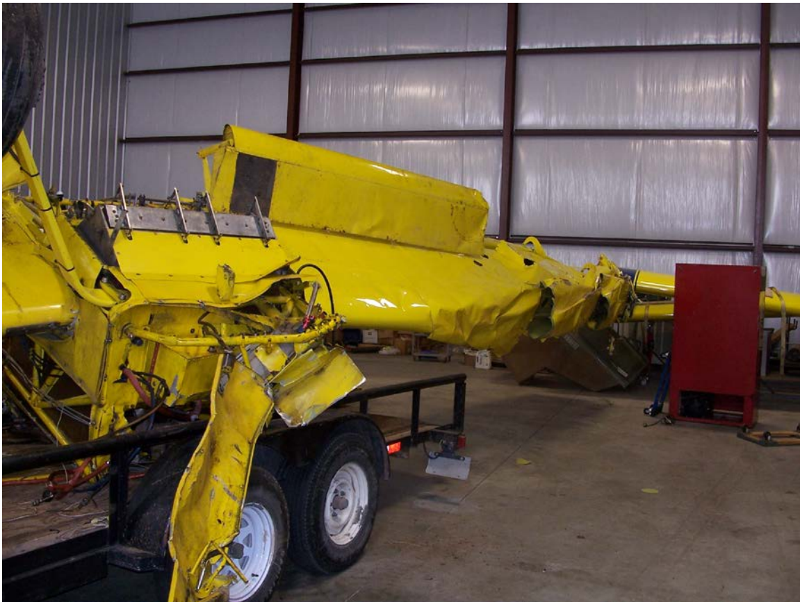
Condition of Wreckage As Examined (Mid Fuselage and R/H Wing Shown)
