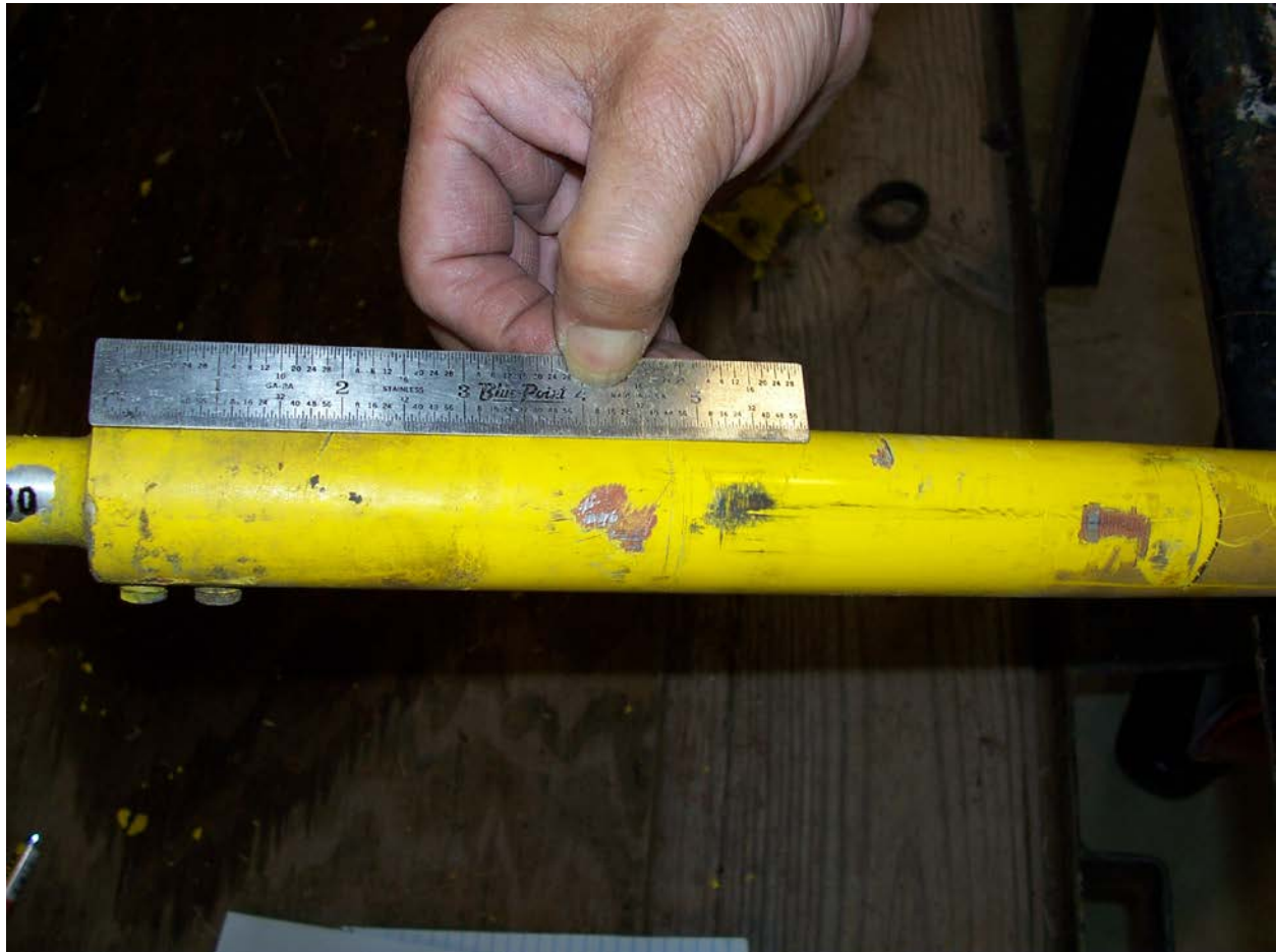
Inboard end of long aileron pushrod (p/n 70013-1) showing fresh chafe marks
