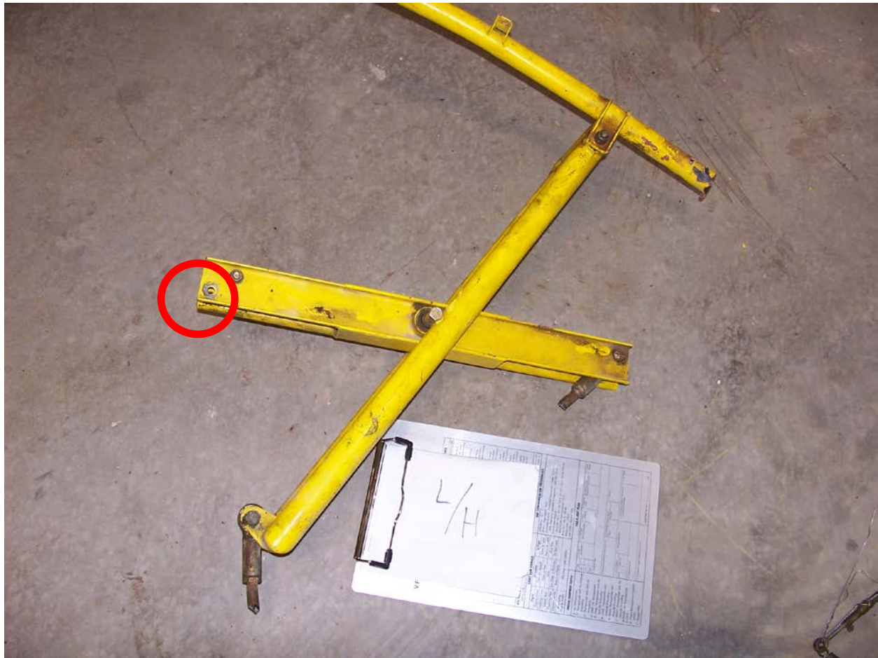
Righthand Aileron Bellcrank and Moveable Frame
