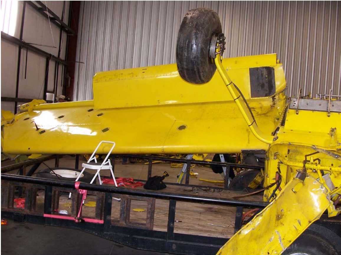
Condition of Wreckage As Examined (Mid Fuselage, L/H Main Landing Gear, and L/H Wing Shown)
