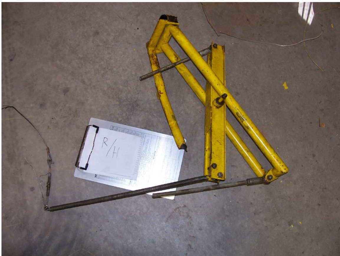
Righthand Aileron Bellcrank and Moveable Frame
