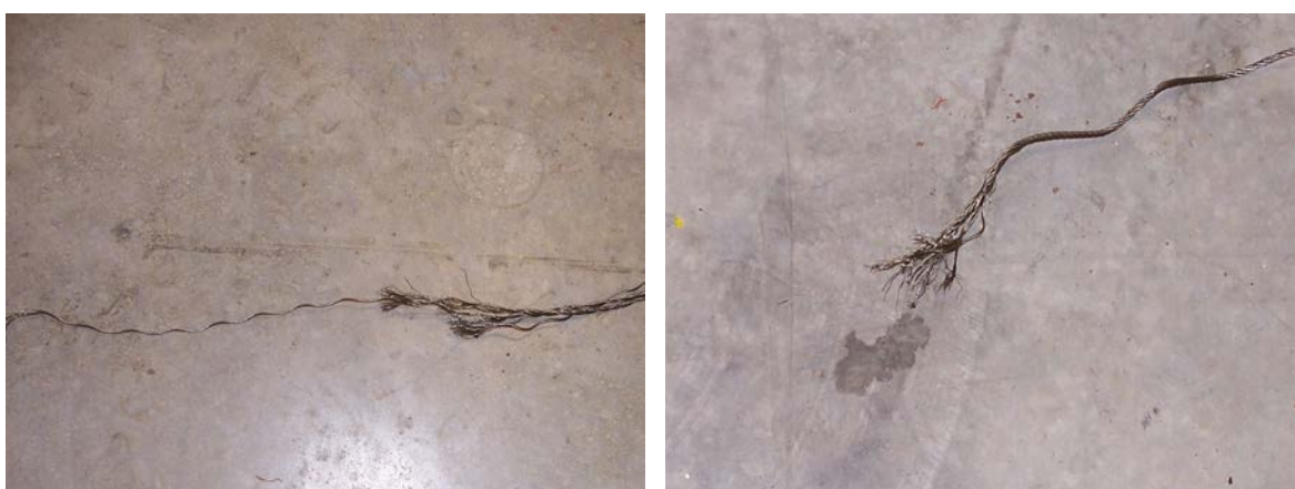
Ends of Rudder Cables
