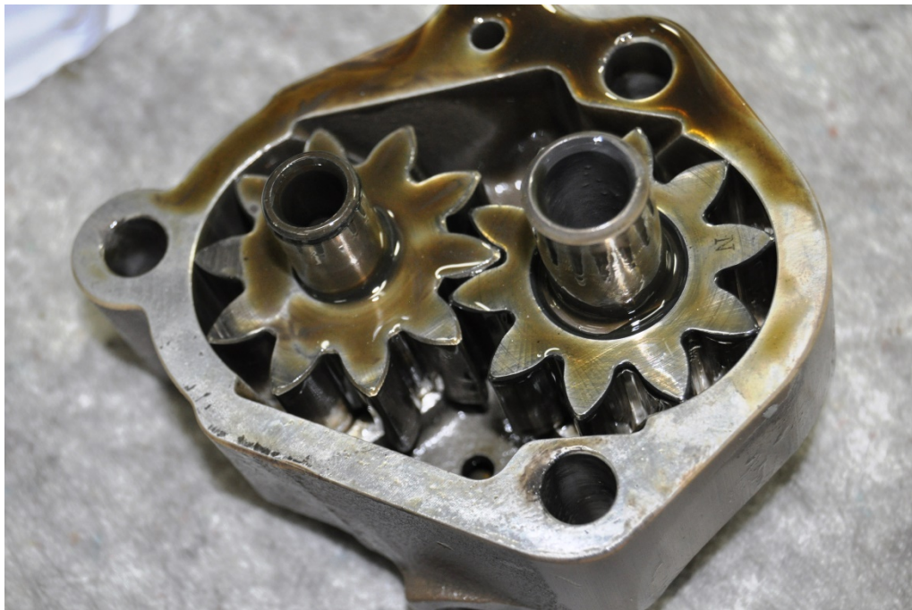
Photograph 29 Interior of oil pump with no indications of significant debris circulating through the pump.
