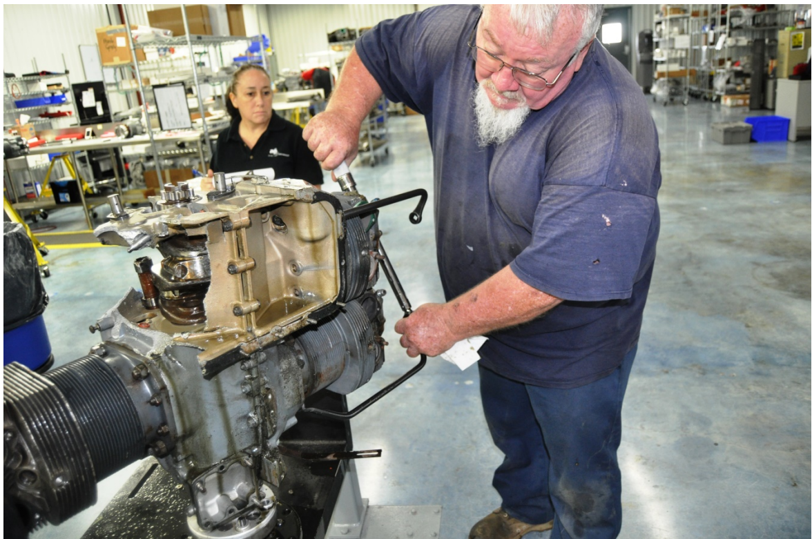
Photograph 4 Checking cylinder flange nut torque during disassembly
