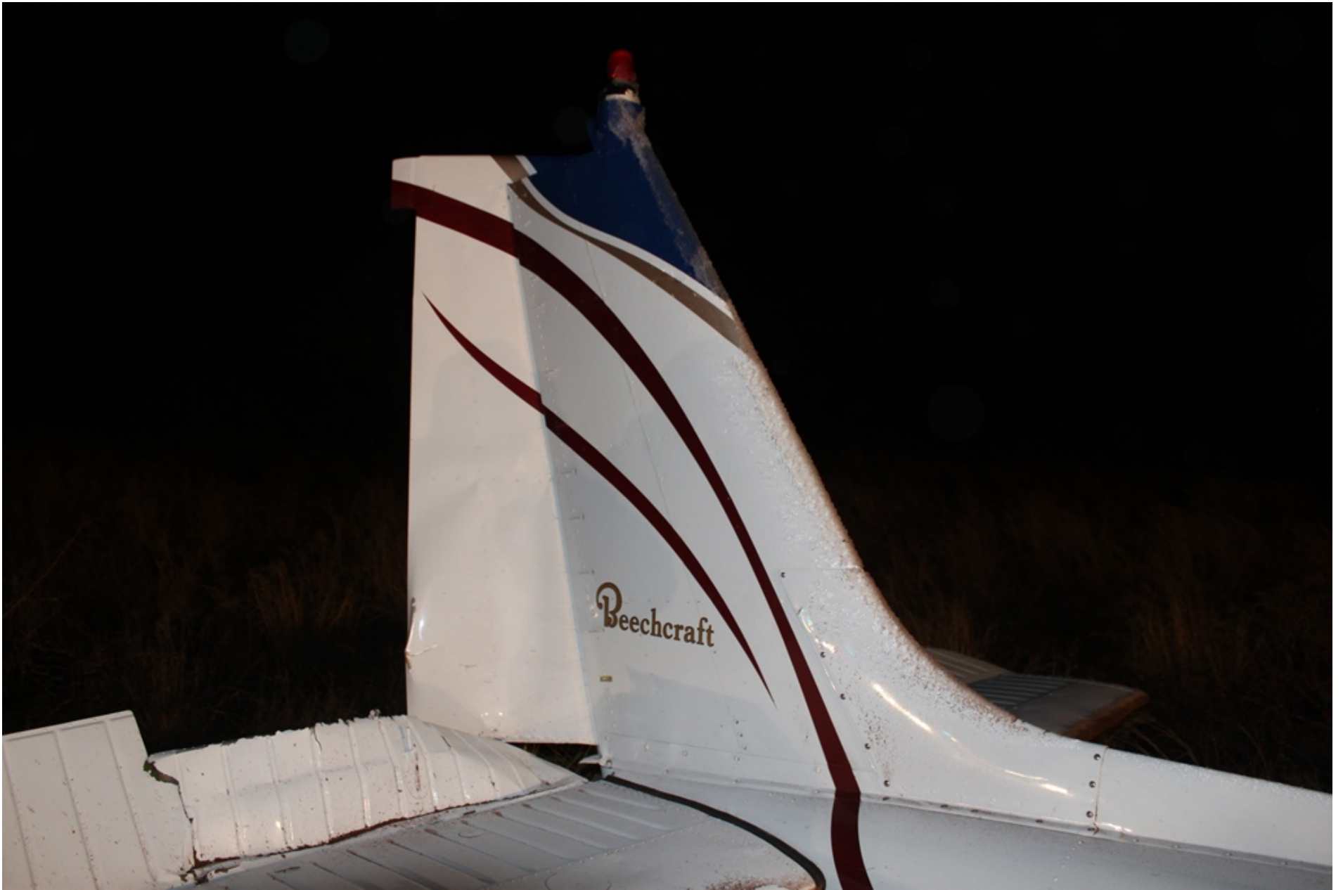
Photo 3 – Ice on the Vertical Stabilizer
