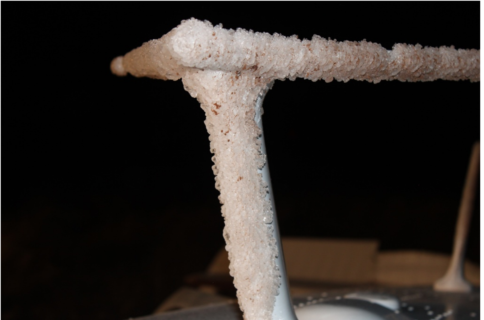
Photo 7 – Ice on Antenna
