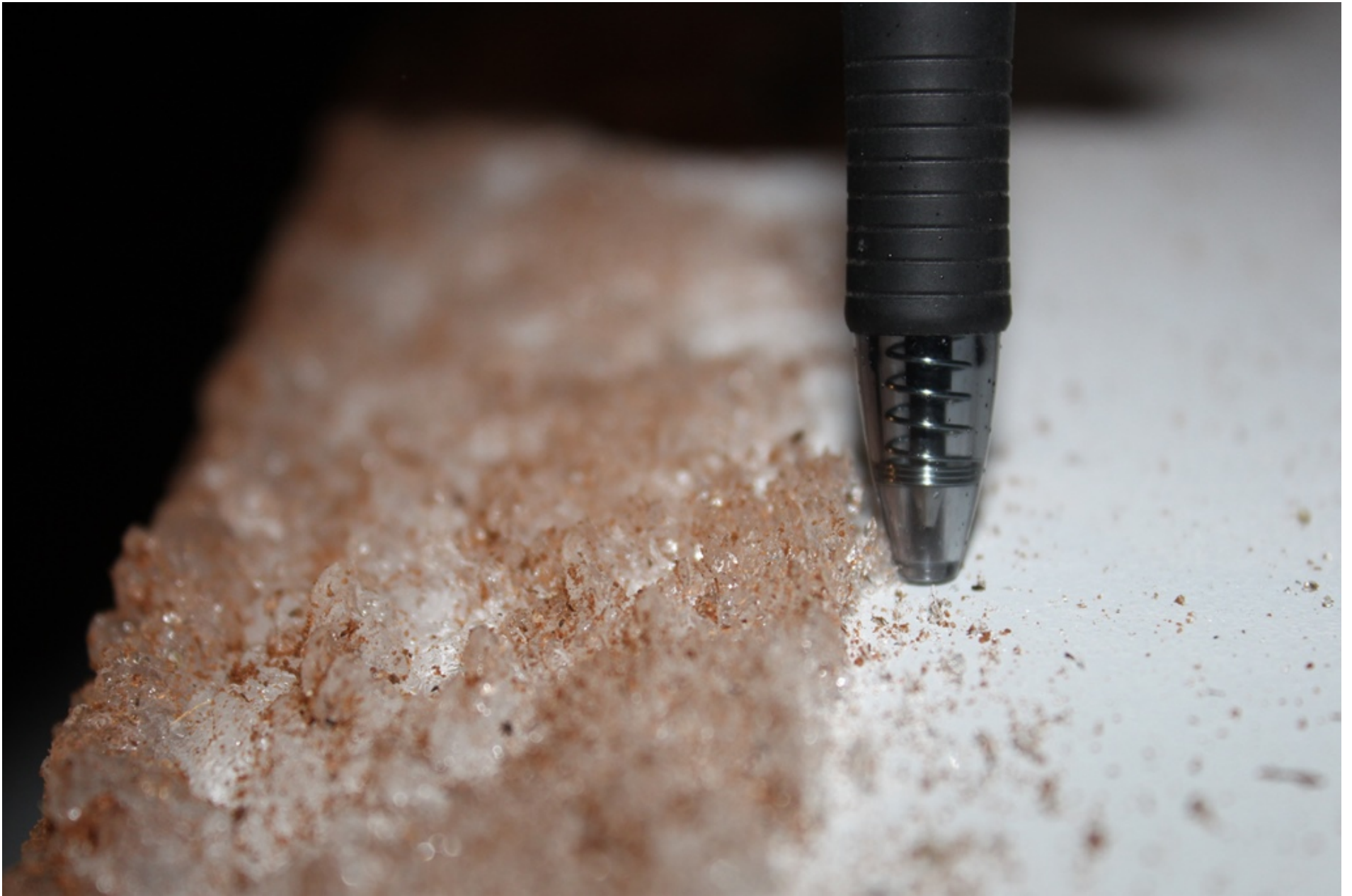
Photo 11 – Ice on Left Horizontal Stabilizer
