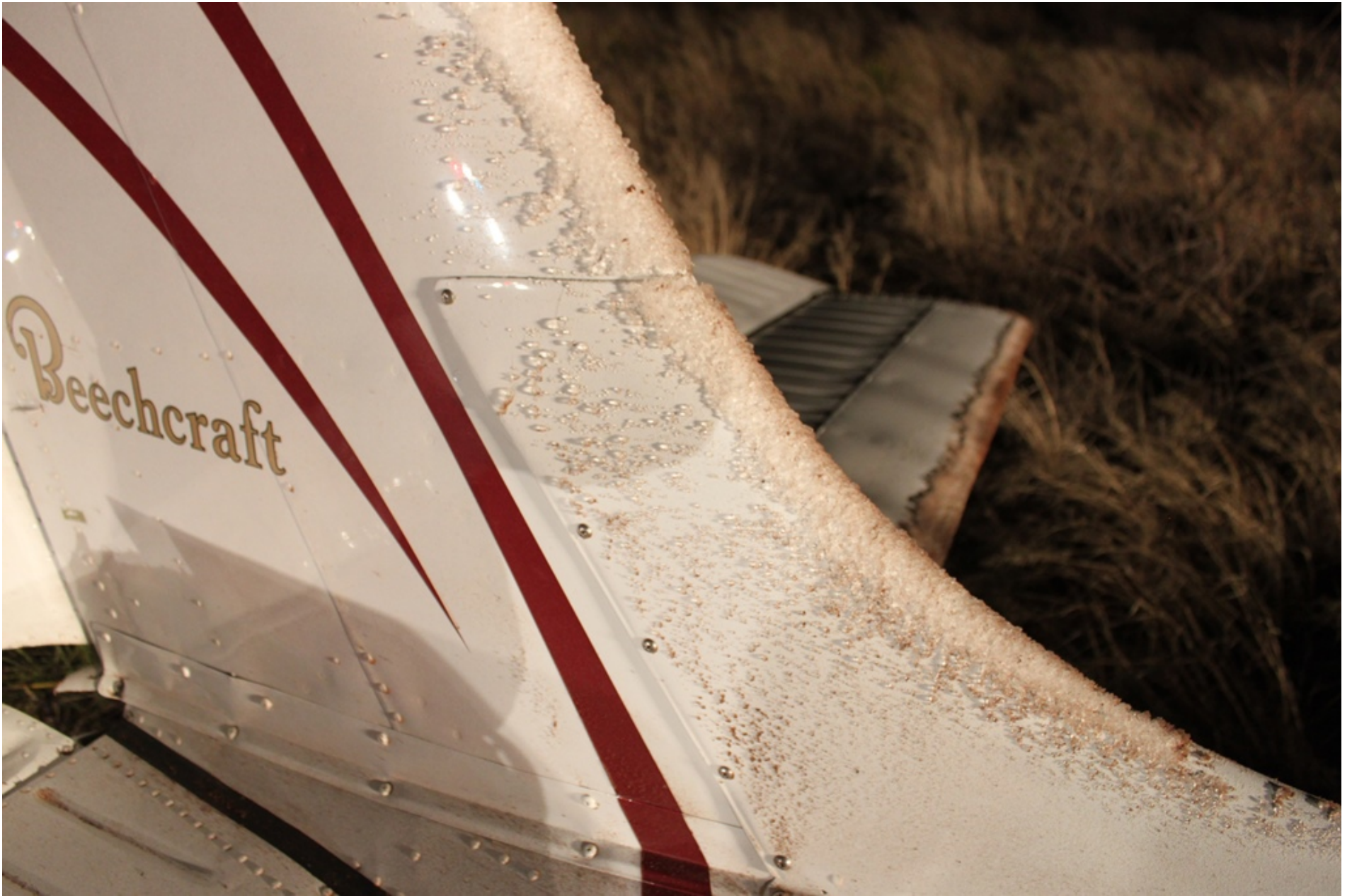
Photo 4 – Ice on the Vertical Stabilizer
