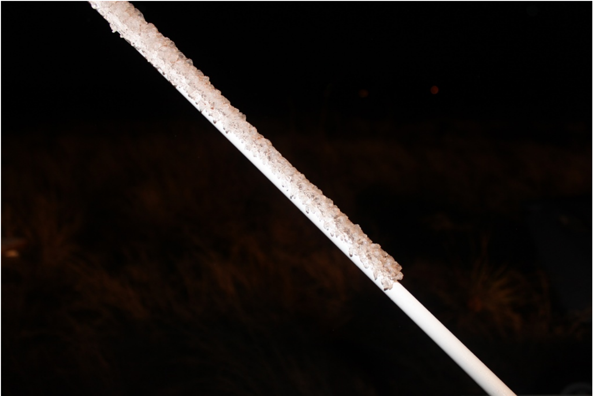
Photo 8 – Ice on Antenna
