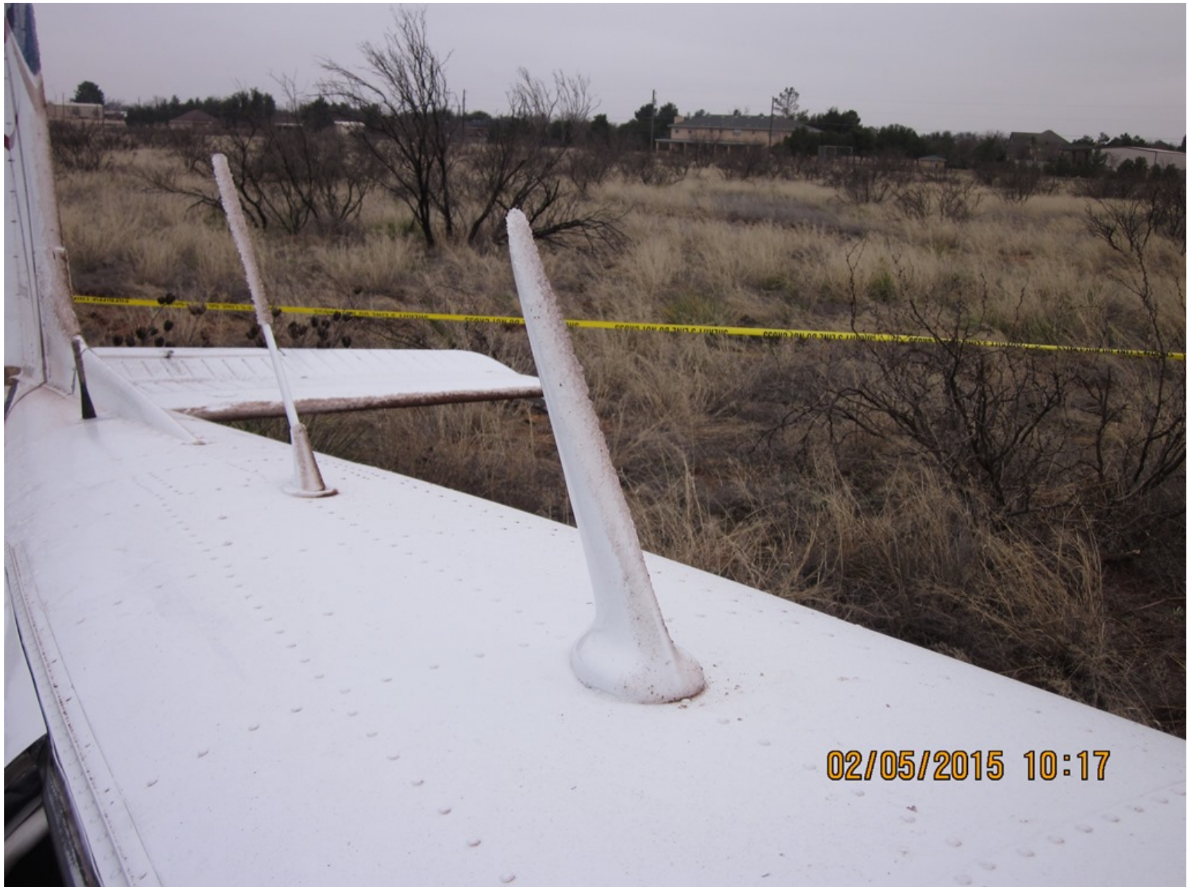
Photo 6 – Ice on the Antennas
