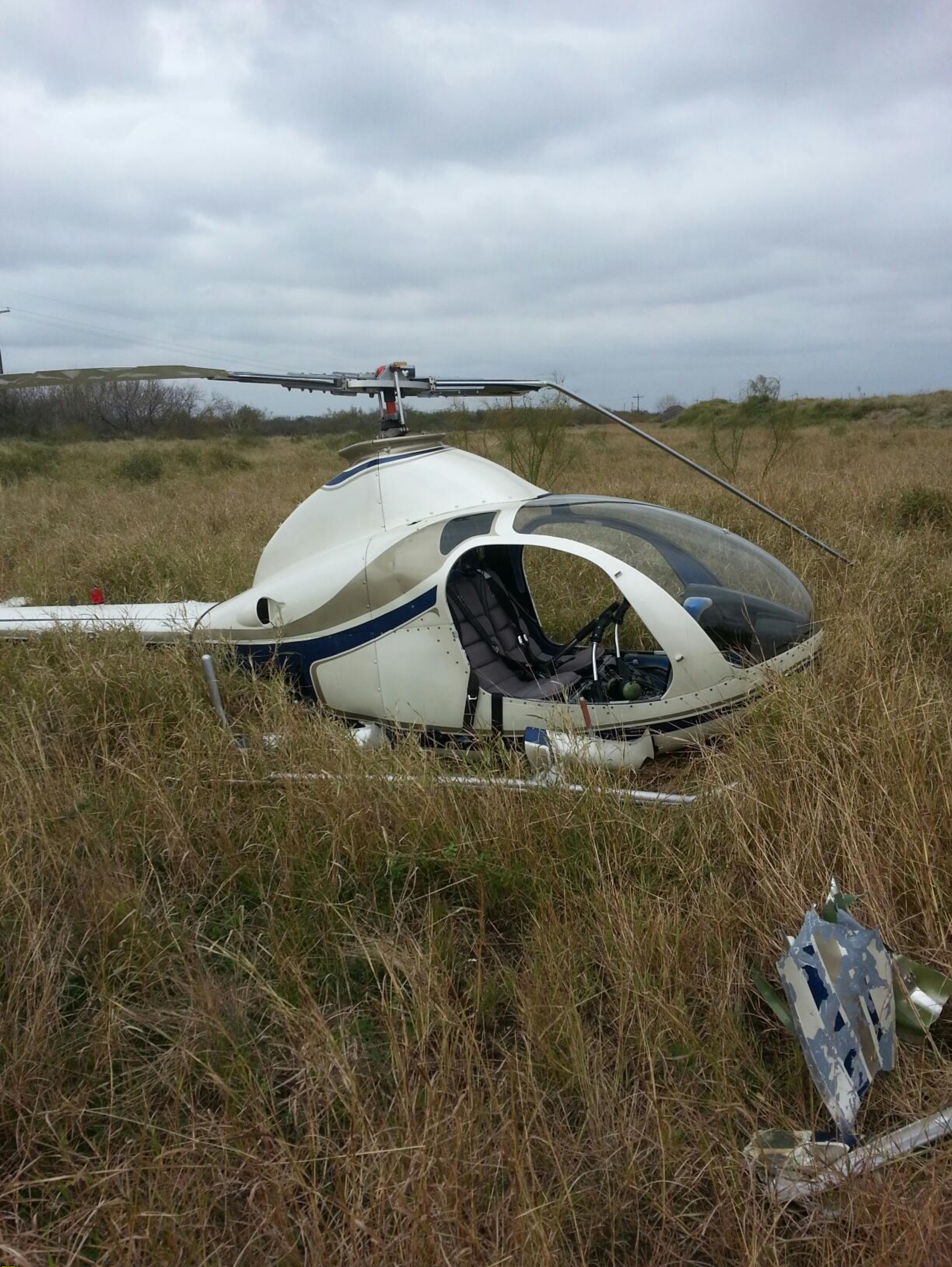
Photo 2 - Closer view shows bent rotor blades and buckled skids
