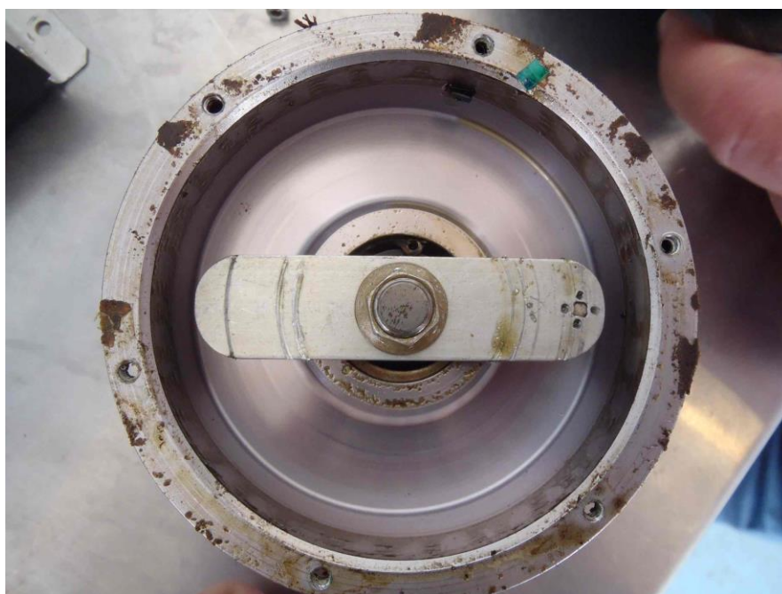
Photo 7 - Hall Effect Module Rotor
