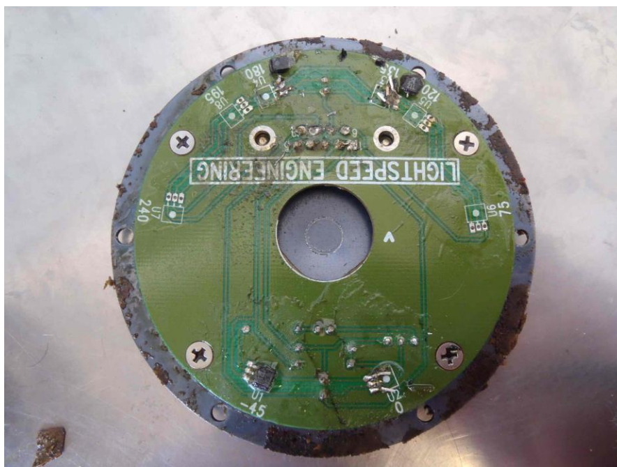
Photo 6 - Hall Effect Module Circuit Board
