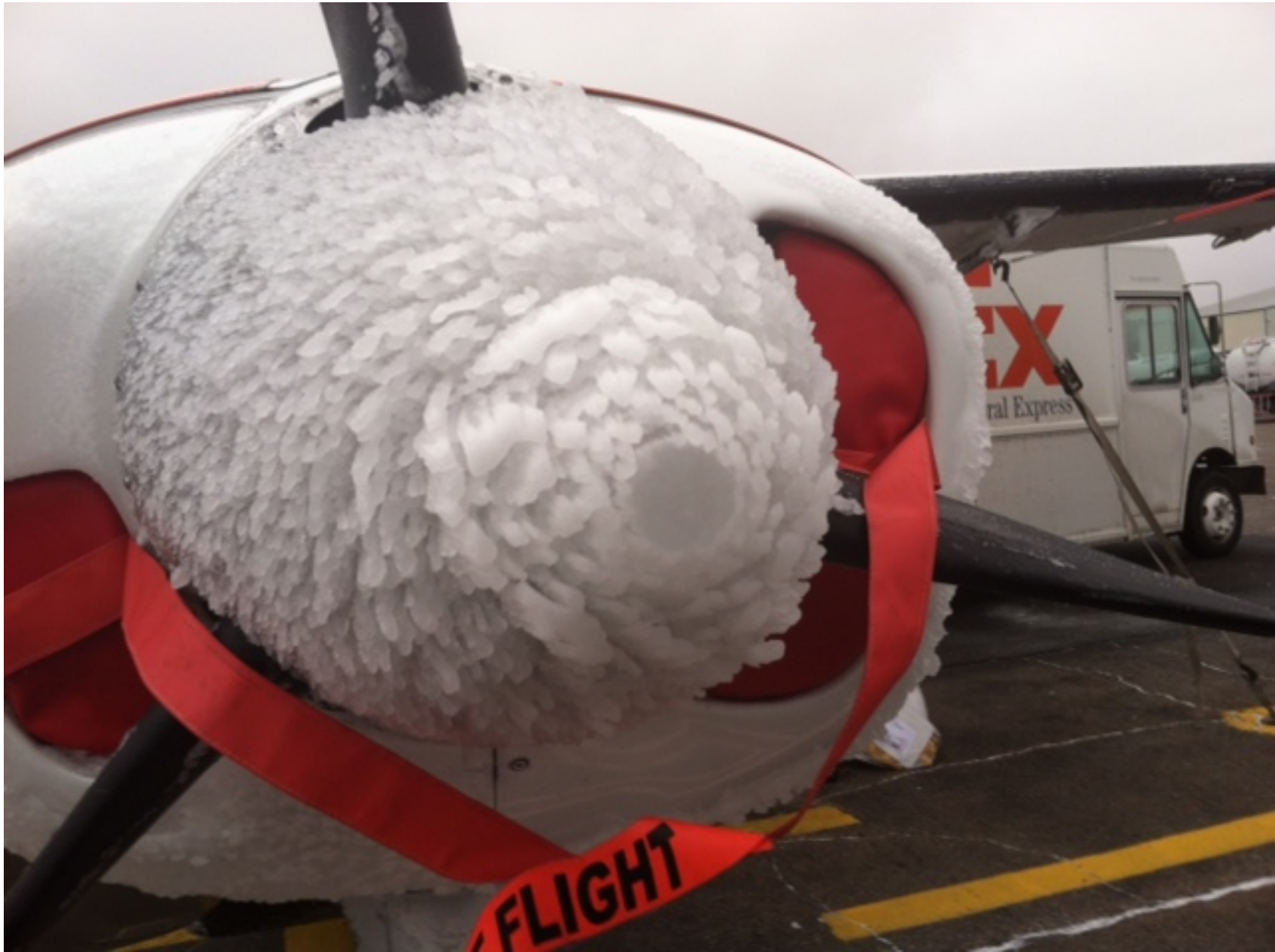
Photo 2 - Spinner – Frost and Ice buildup
