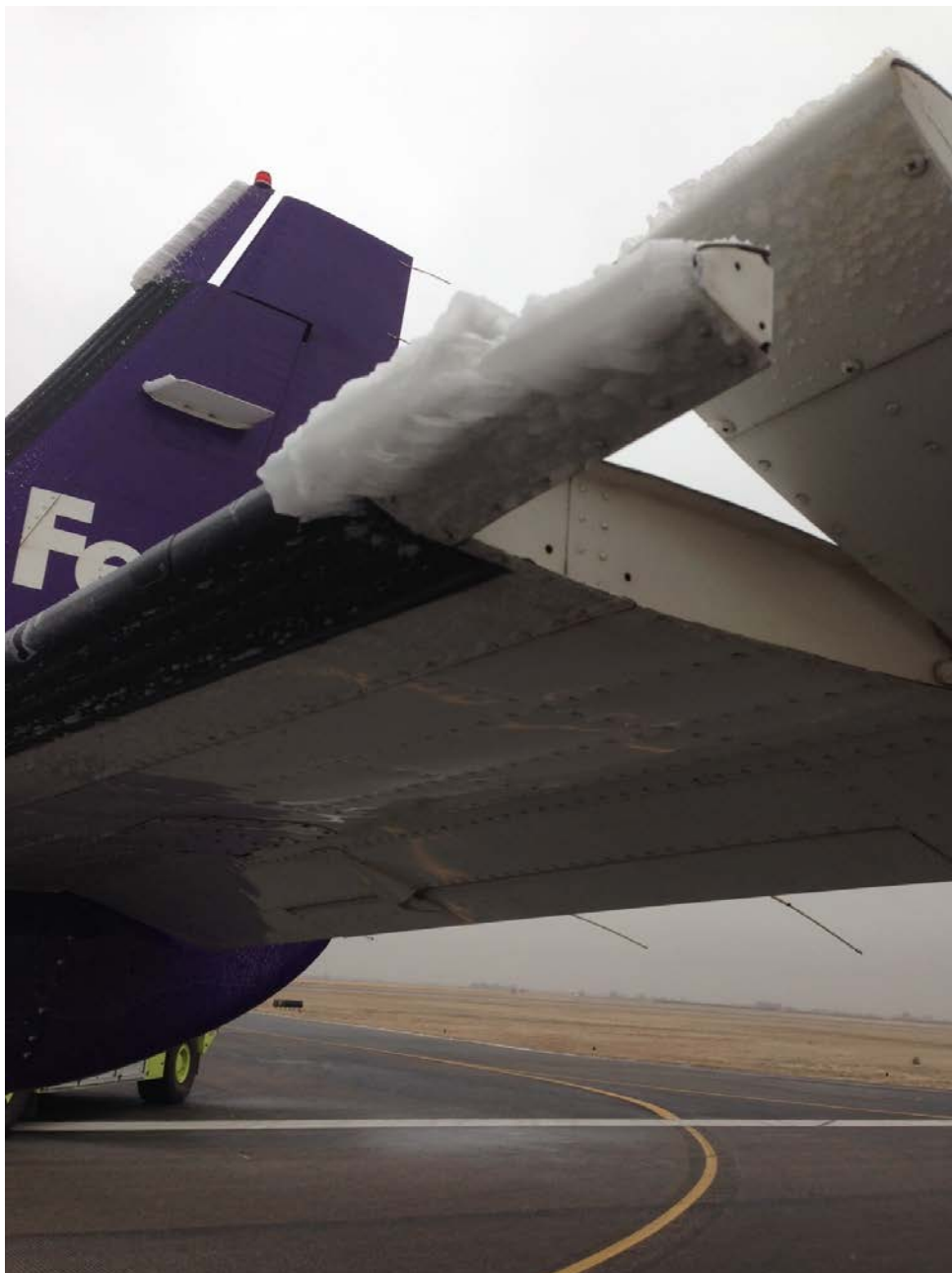
Photo 1 - Ice build-up on outboard of horizontal and elevator tip
