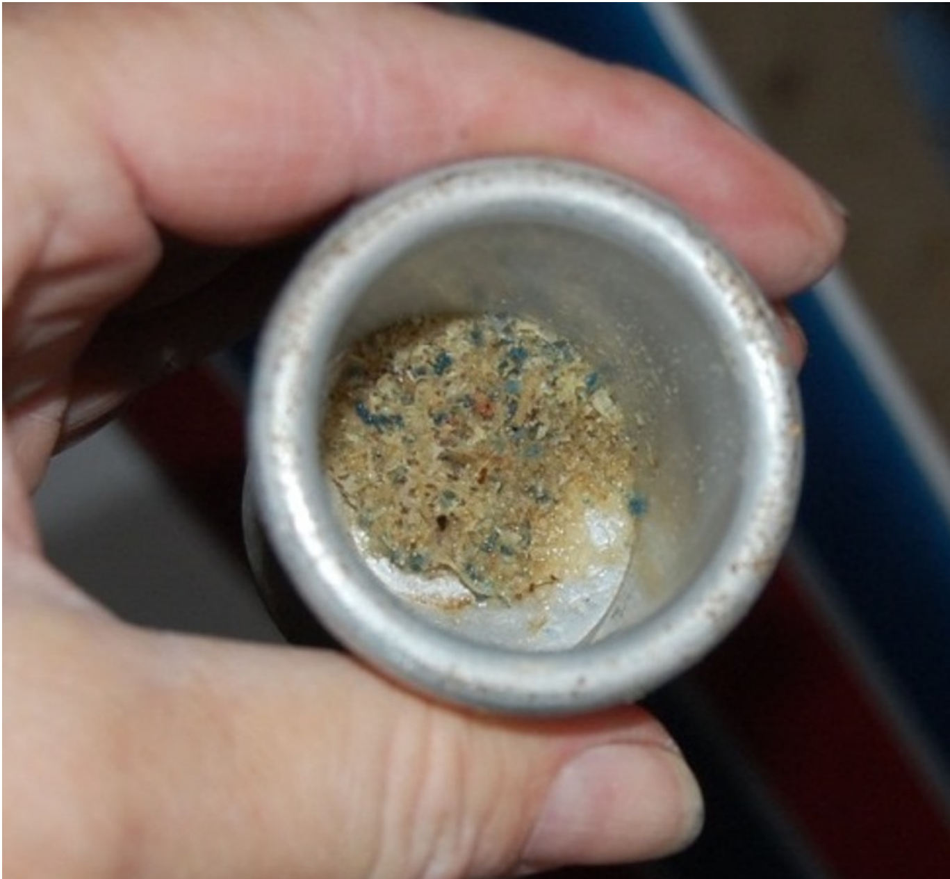
Photo 6 – Close-up view of Debris in the Gascolator Bowl
