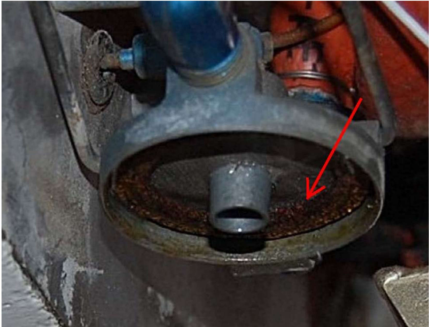
Photo 5 – Close-up View of the Bottom of the Gascolator Housing
