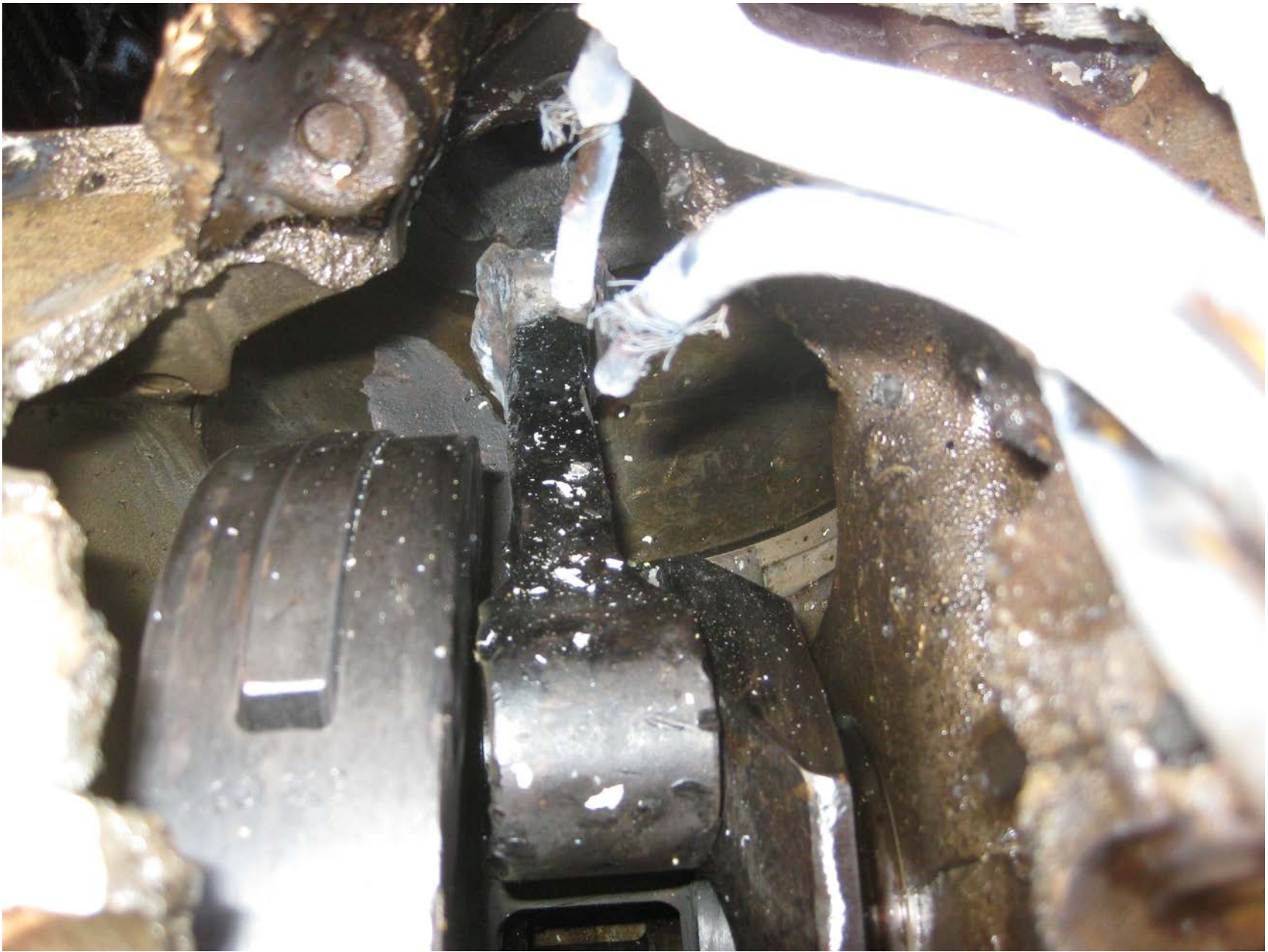
Photo 4 – Hole in crankcase of engine
