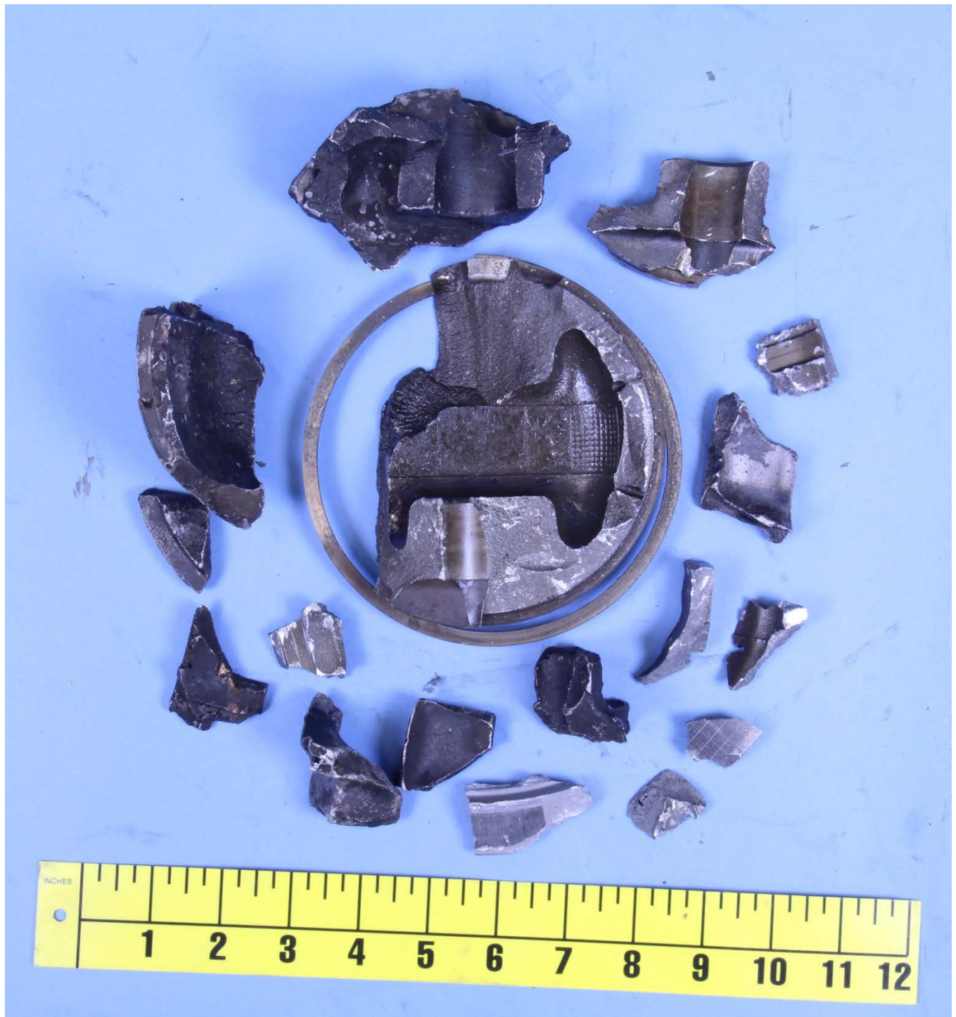
Figure 1. An overall view of the piston fragments including the top compression ring.
