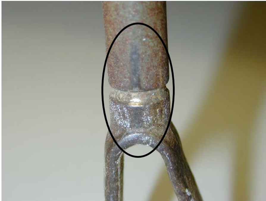
Figure 7. View of the underside of the trim tab push-pull rod showing light wear (circled). Magnification: x2.8.
