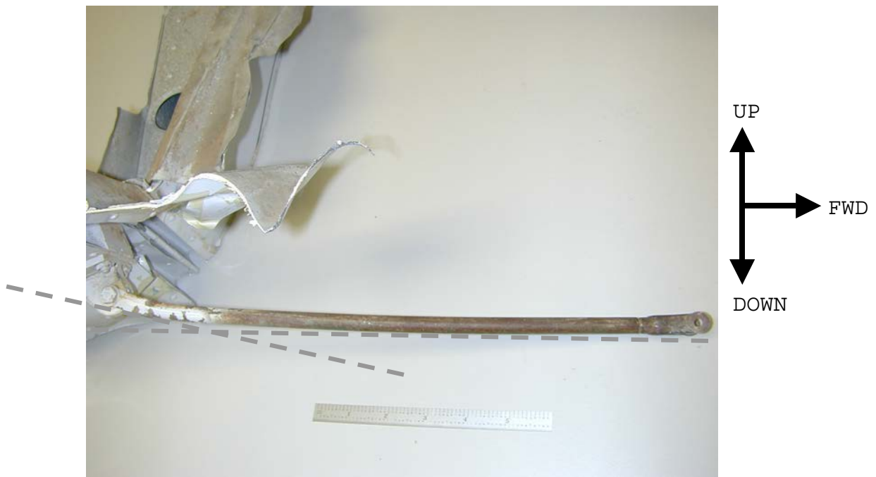
Figure 11. View of a trim tab actuator rod. Note that the rod has been bent upward near the trim tab.
