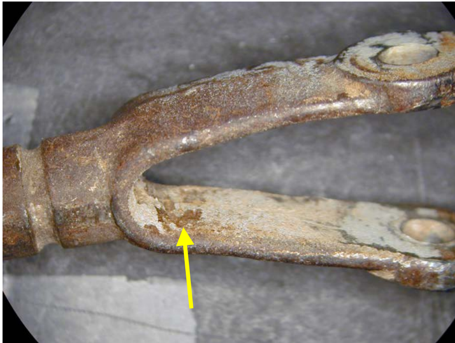
Figure 9. Close up view showing light wear marks on the inner surface of one of the forward clevis (arrow). Magnification: x2.9.
