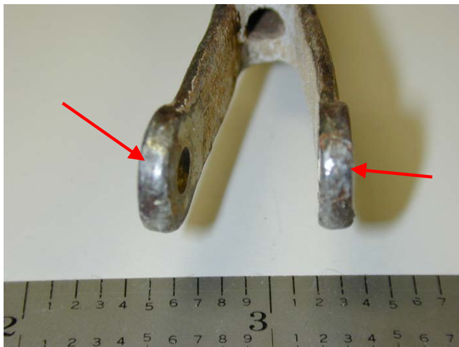
Figure 6. Close-up view of the ends of the forward clevis forks, showing some non-corroded worn areas (arrows). Magnification: x2.45.
