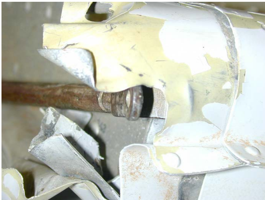
Figure 15. View of the lead edge of the elevator, looking aft, showing the indentations and the corresponding positions of the legs of the forward trim tab actuator clevis.
