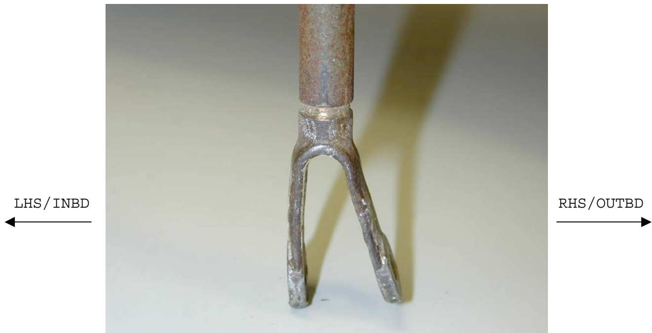
Figure 5. View of the forward clevis of the trim tab push-pull rod, which was spread open approximately 0.3 inches. Magnification: x1.4.
