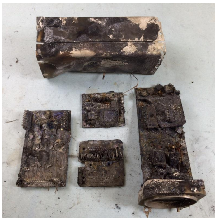
Figure 2. The JPI EDM-700 after disassembly and inspection.
