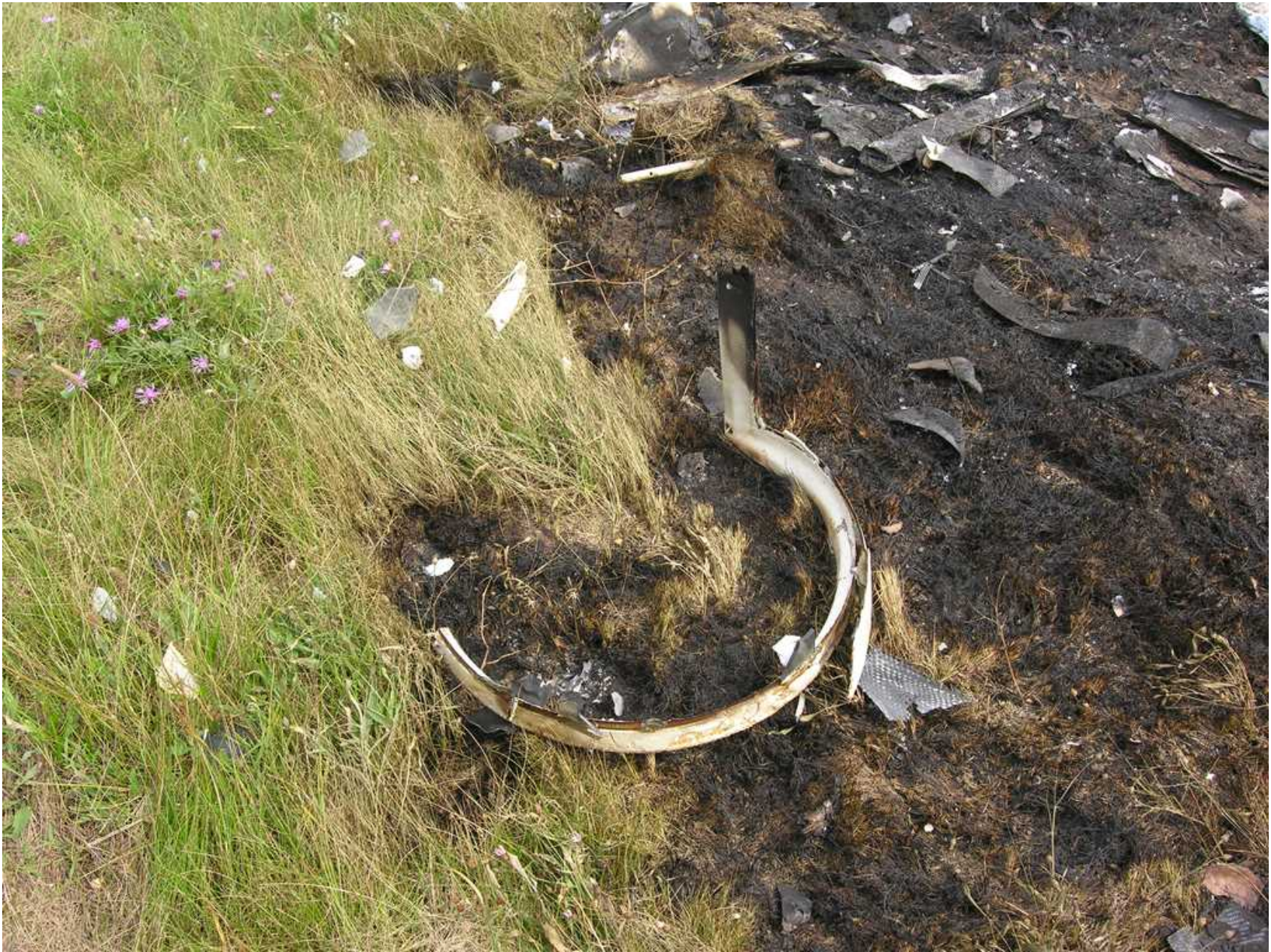
Photo 5 - Wreckage: canopy bow
