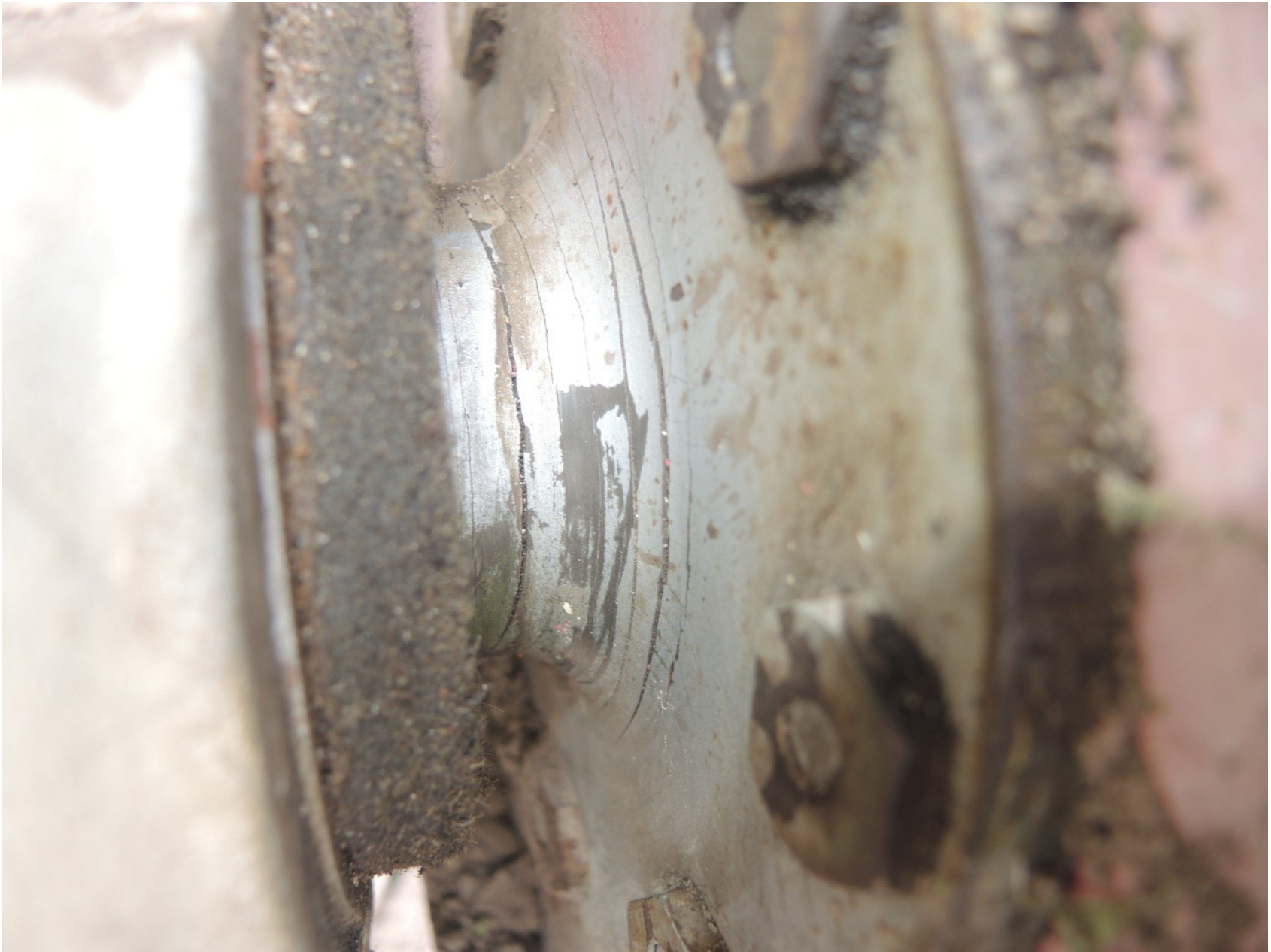
Photo 8 - Torsional Stress Mark Signatures on the Engine Crankshaft Propeller Flange
