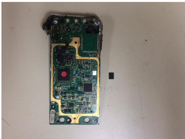
Figure 4. Photo of NVM chip after removal from circuit board.
