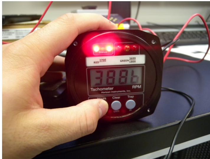
Figure 1. P1000 displaying tachometer time in hours.
